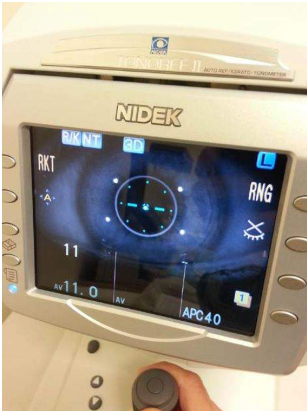
Figure 2-8. Nidek TONOREF II™ manual measurement (no “A” box at top of the screen).
