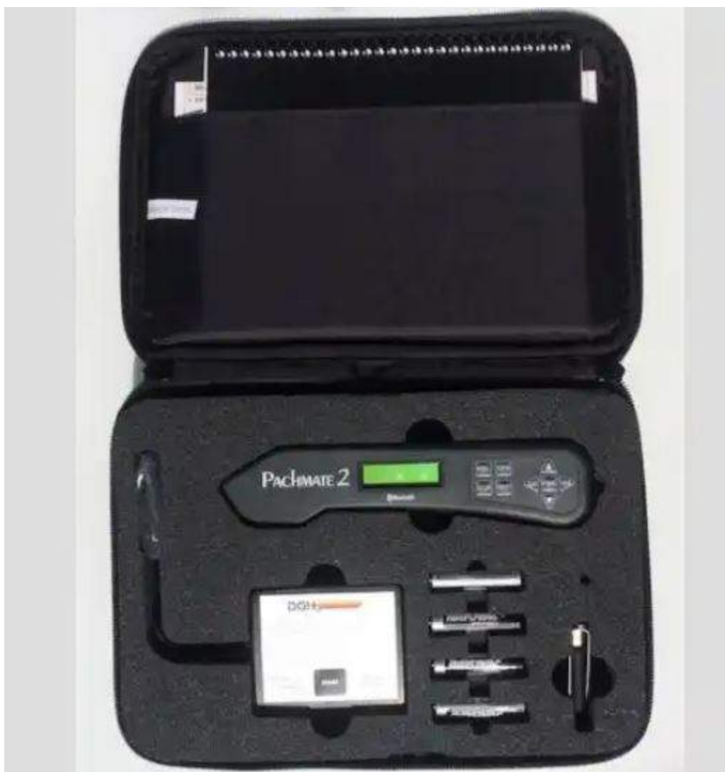
Figure. 3-44. Pachmate® handheld pachymeter and calibration box.
