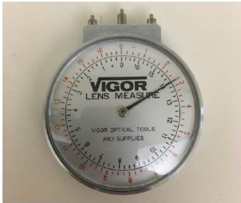
Figure 3-43. Lens clock.
