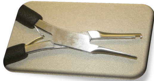
Figure 3-58. European pad adjusting pliers.
