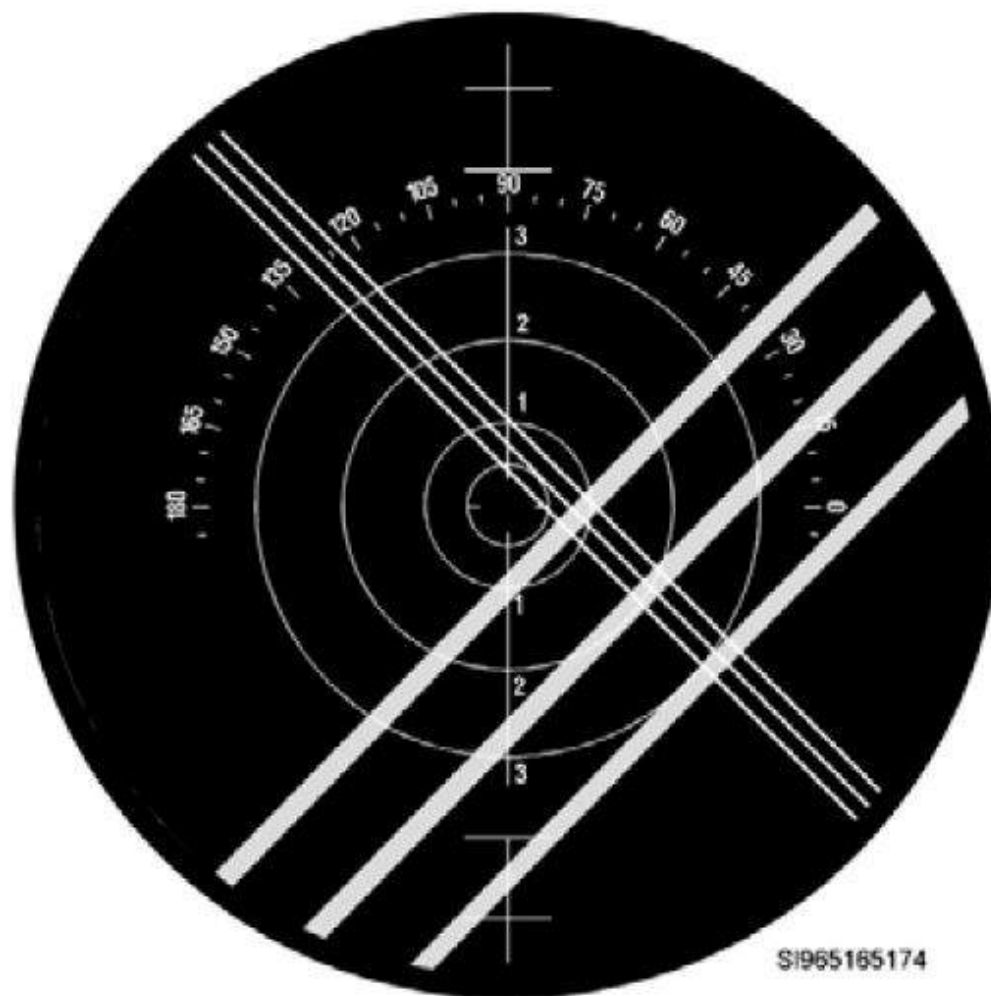
Figure 3-30. Unfocused sphere and cylinder power lines (mires).
