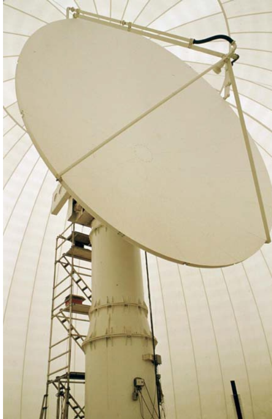
Figure 2-16. Inside view of Doppler radar.
