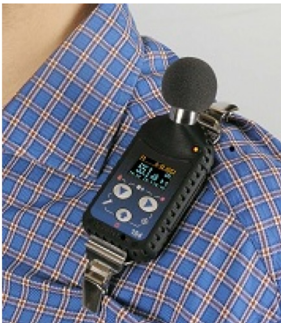
Figure 5–12. Placement of Dosimeter Microphone.
