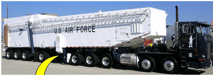
Figure 1-17. TE environmental control unit.
