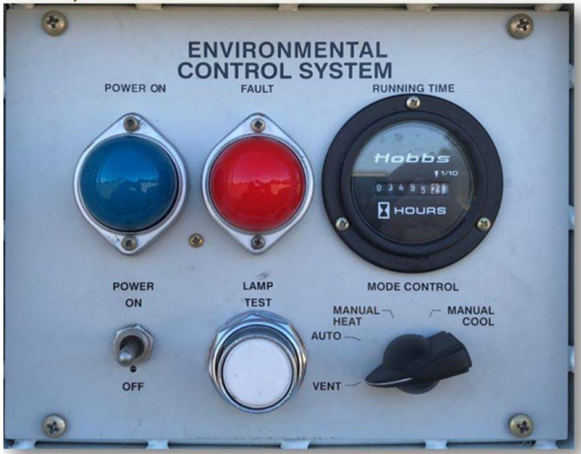
Figure 1-25. PT ECS Control Panel.
