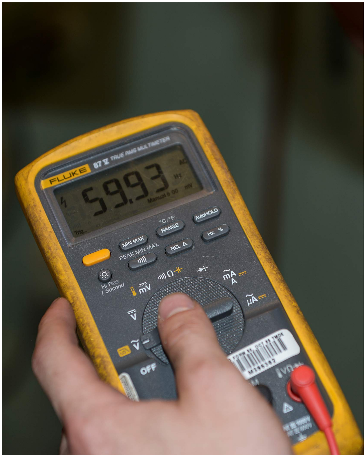
A member of 91st Missile Maintenance Squadron (MMXS) facilities maintenance section verifies diesel hertz on a multi-meter at a launch facility near Minot Air Force Base, North Dakota, July 17, 2018. The annual code change requires maximum effort across the wing.
