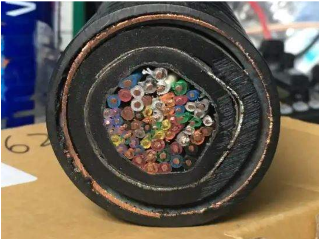
A section of a hardened intersite cable used to connect MMIII silos to launch control centers (LCCs). This came from the demolished wings around Whiteman AFB.
