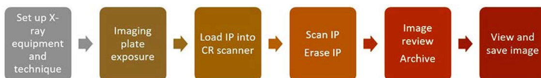
Figure 2-2. CR imaging flowchart.
