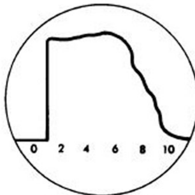
RINGING SIGNAL FROM UNBONDED AREA
