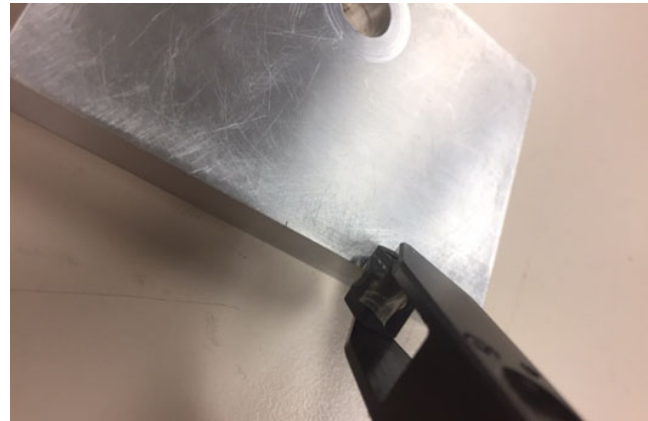
Figure 1-29. Conformal probe used with standard.
