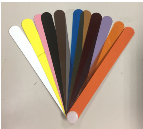
Figure 1-38 Shims used for lift-off compensation.
