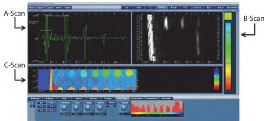
Figure 2-22. A-scan, B-scan, and C-scan.
