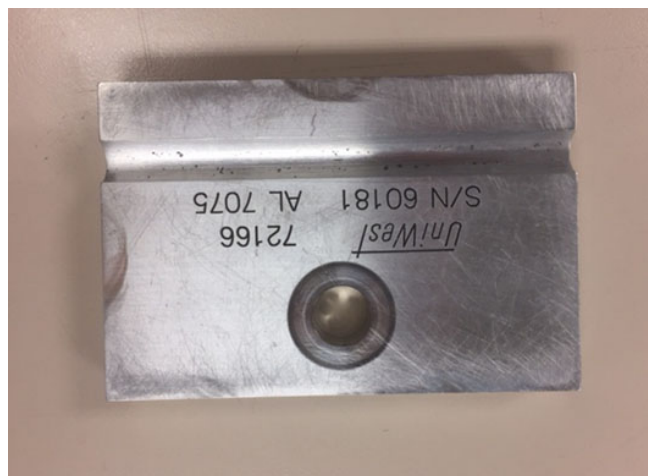
Figure 1-30. Conformal probe standard.
