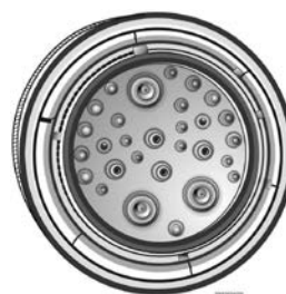
Figure 2-8. Generic MIL-STD-1760 compliant connector face.
