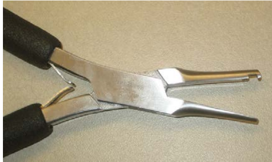
Figure 3-58. European pad adjusting pliers.
