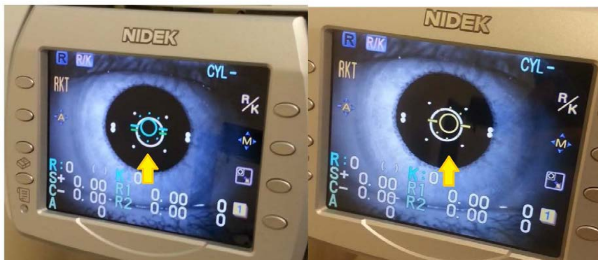
Figure 3–23. Nidek TONOREF II™ blue to yellow target alignment change.
