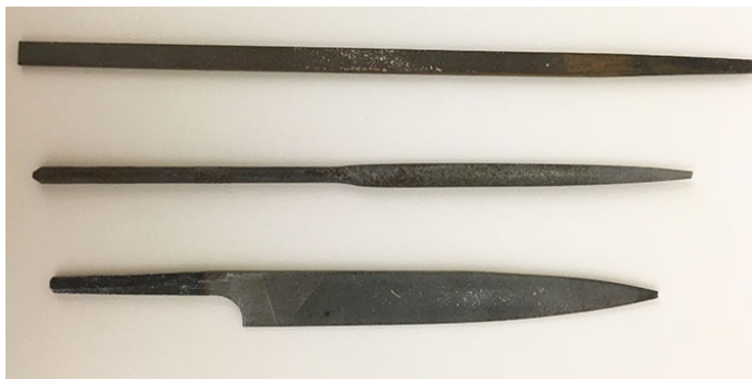
Figure 3-64. Files that can be used on spectacles.
