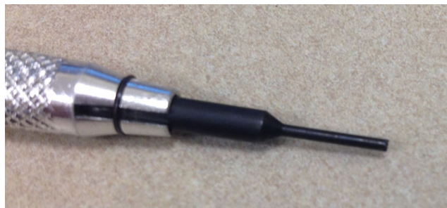
Figure 3-53. Screw remover/extractor.
