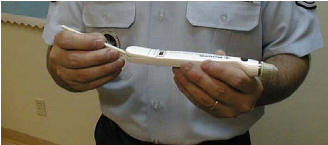
Figure 2-11. Tono-pen®, remove battery cover with stylus.
