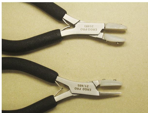
Figure 3-65. Zyl gripping pliers.
