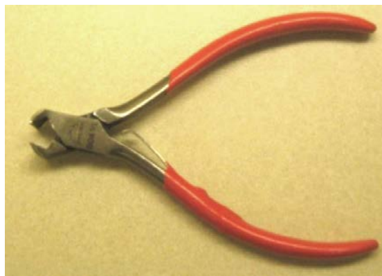
Figure 3-70. End cutting pliers.
