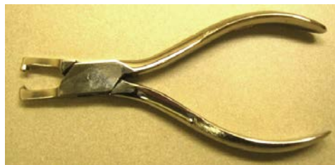
Figure 3-52. Flaring (screw or rivet peening) pliers.
