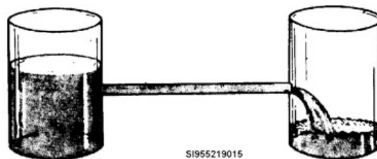
Figure 2-2. Demonstrating the flow of electrons from a surplus to a deficit.
