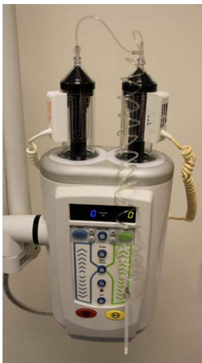
Figure 3-38. Dual-head automatic IV pressure injector.
