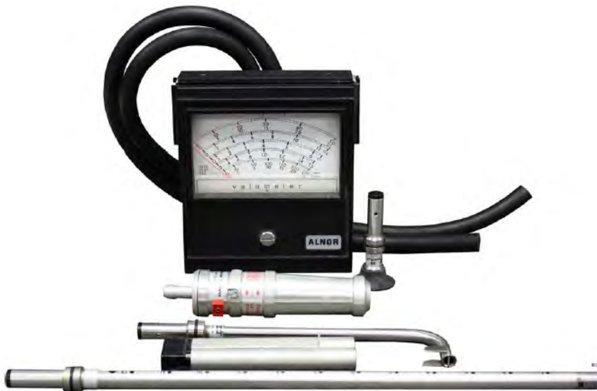
Figure 2–32. Velometer—swing anemometer.
