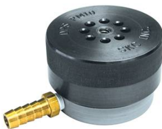
Figure 3-16. Inertial impactor collection device used with the DPS.
