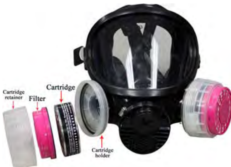
Figure 3-1. Full-face air purifying respirator.
