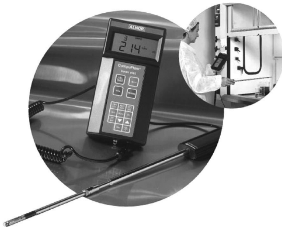
Figure 2-33. Thermal anemometer.
