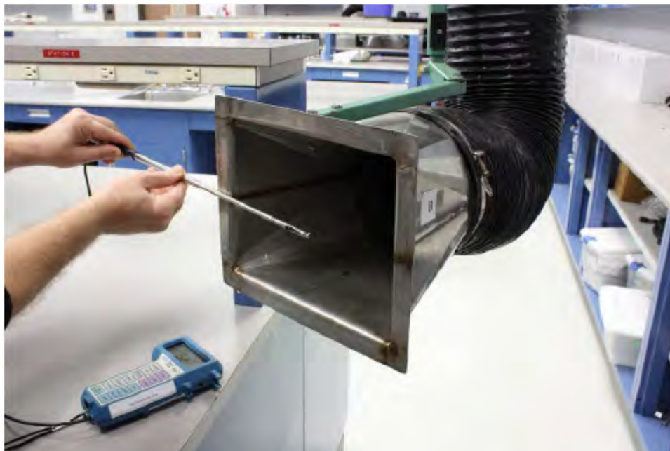
Figure 2–31. Face velocity measurement.
