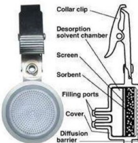
Figure 3-7. Passive air monitor. [3]
