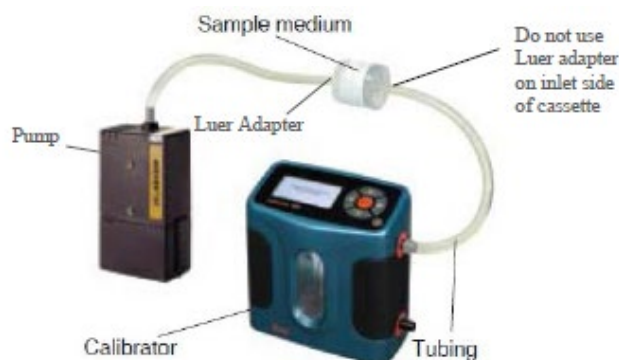
Figure 3-21. Calibration with near-frictionless piston meter.
