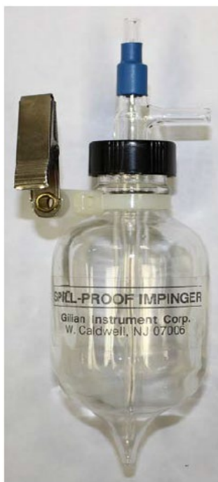
Figure 3–9. Absorption sampling device (standard midjet impinger).
