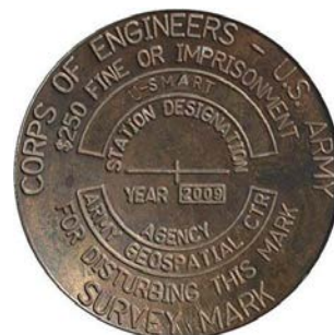
Figure 2-1. Standard brass survey disk.
