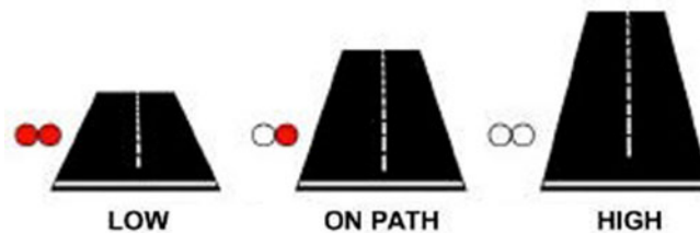
Figure 2-54. Glide slope indicators.
