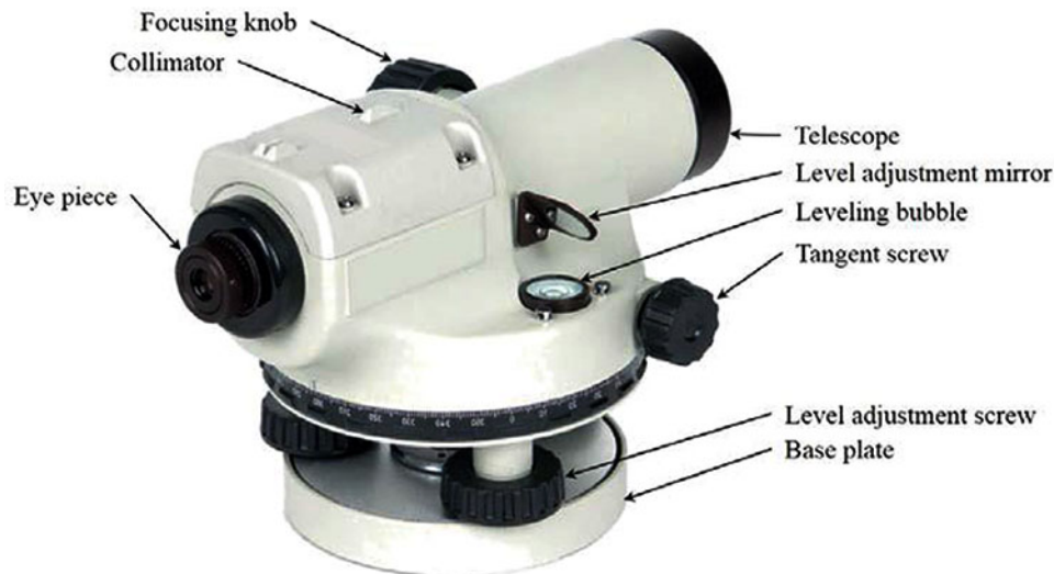
Figure 2-14. Common auto-level.
