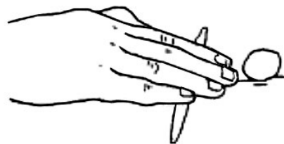
Figure 2-32. Roll or thread test.
