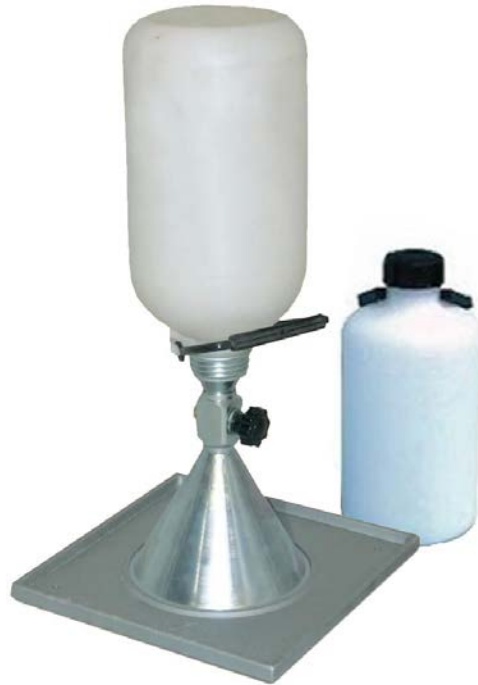
Figure 2-41. Sand cone apparatus and container.
