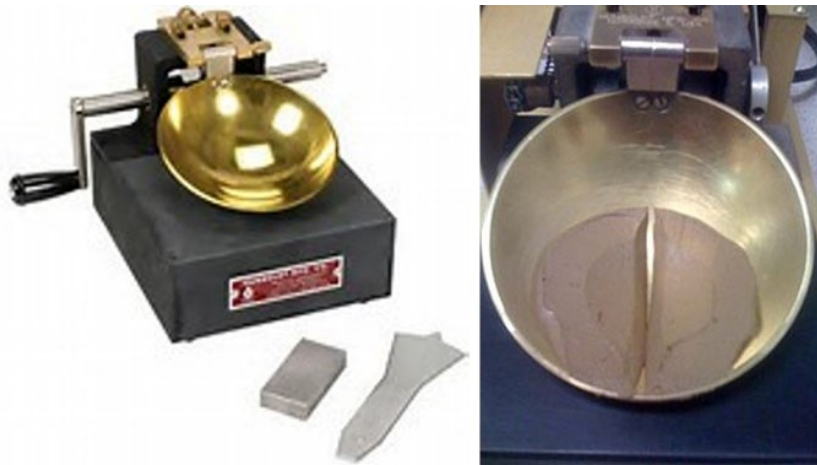
Figure 2-39. Casagrande cup for the liquid limit test.
