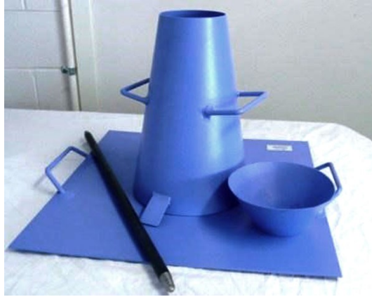
Figure 2-46. Slump test equipment.
