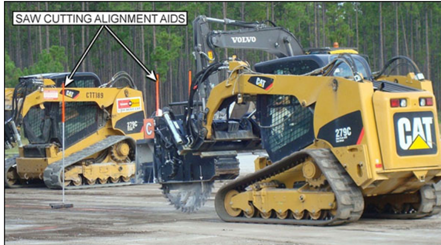
Figure 1-14. Pavement cutting alignment aids.
