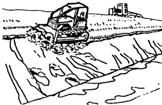
Figure 1-24. Cut-and-spread sequence.
