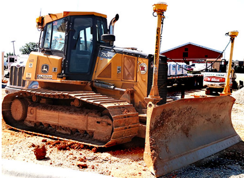
Figure 3-14. GPS dozer masts.
