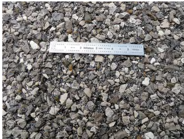
Figure 5-15. Polished aggregate.
