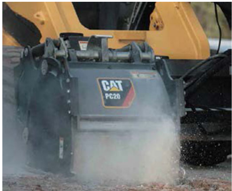
Figure 1-14. Cold planer attachment.
