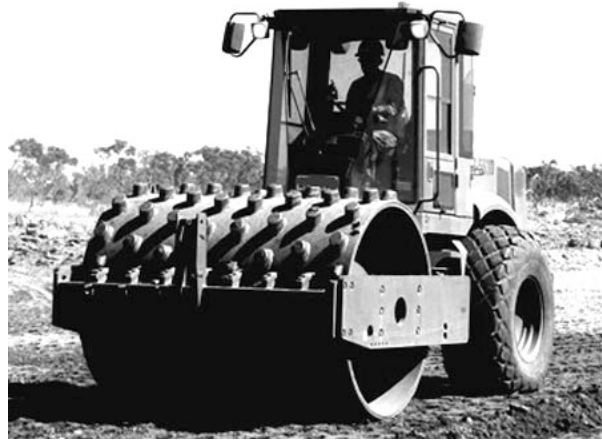
Figure 4-4. Self-propelled sheepfoot roller.
