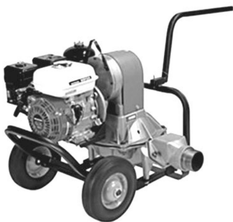
Figure 3-18. Diaphragm pump.
