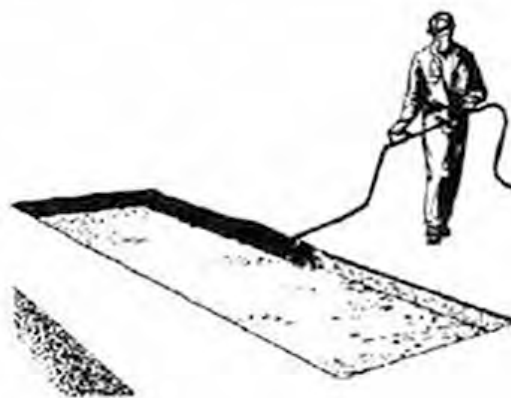
Figure 5-16. Applying a tack coat to the vertical faces.
