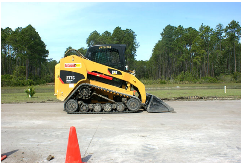
Figure 1-10. Compact track loader.
