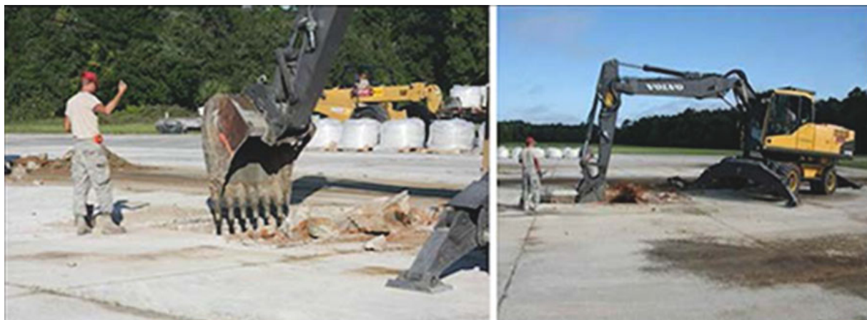
Figure 1-19. Excavator bucket with 24 inch reference marks.
