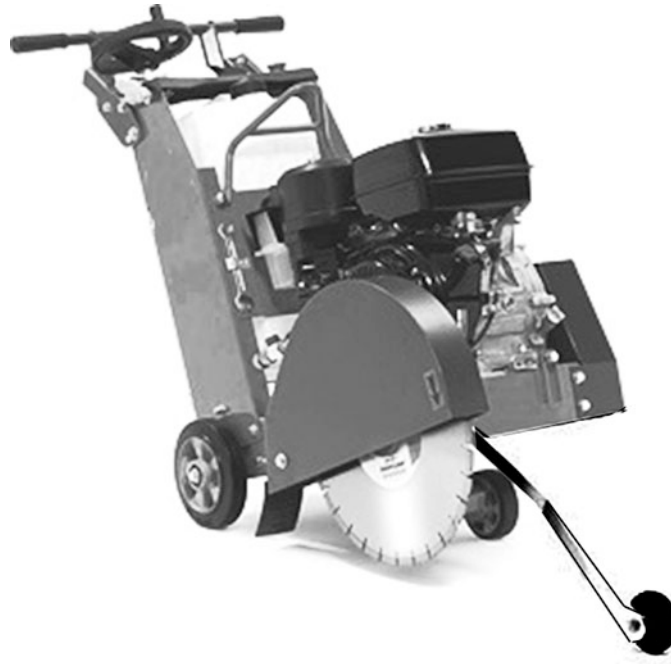
Figure 4-10. Typical walk-behind concrete saw.
