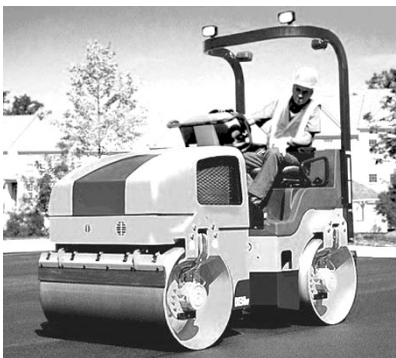
Figure 4-5. Steel-wheel (vibratory compactor) roller.
