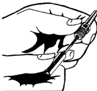
Figure 5-29. Cleaning a disassembled torch tip.
