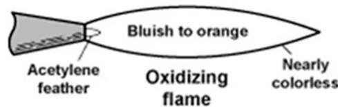
Figure 5-12. Oxidizing flame.
