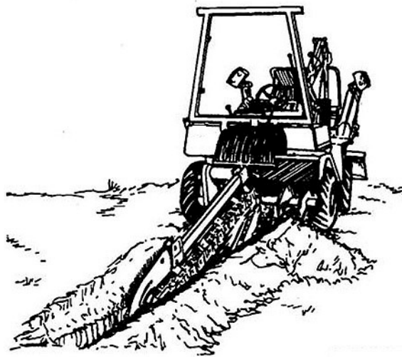
Figure 3-2. Digging with a trencher.
