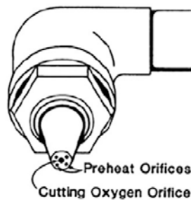
Figure 5-15. Cutting tips.
