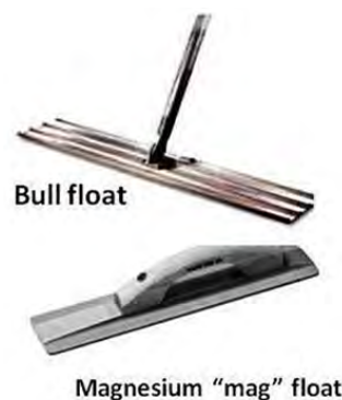
Figure 2–7. Bull float and “mag” float.
