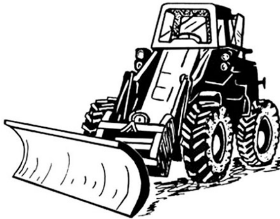
Figure 1-9. Blade attachment.
