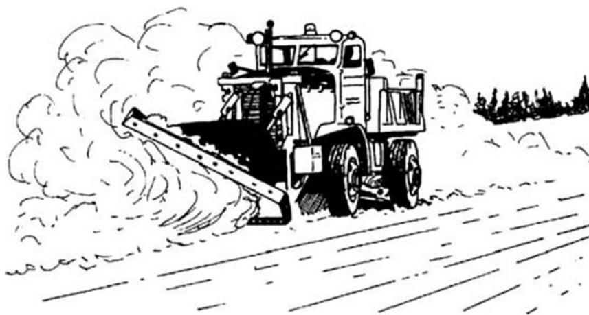
Figure 4-23. Rollover plow.
