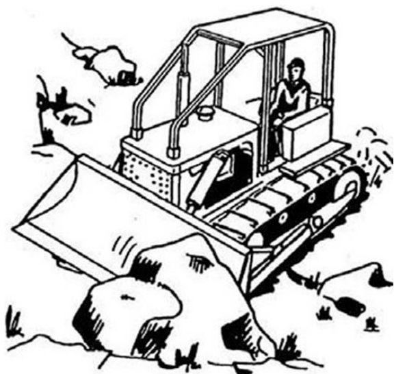
Figure 1-20. Straddle loading.
