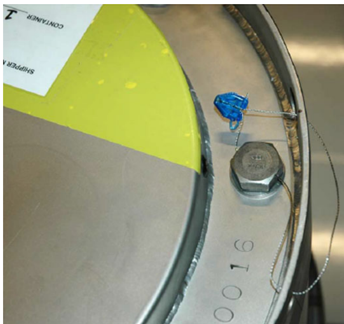
Figure 2-10. Security seal routing.
