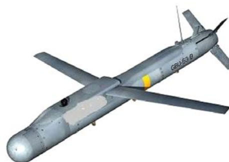
Figure 1-18. GBU-53 small diameter bomb (wings extended).
