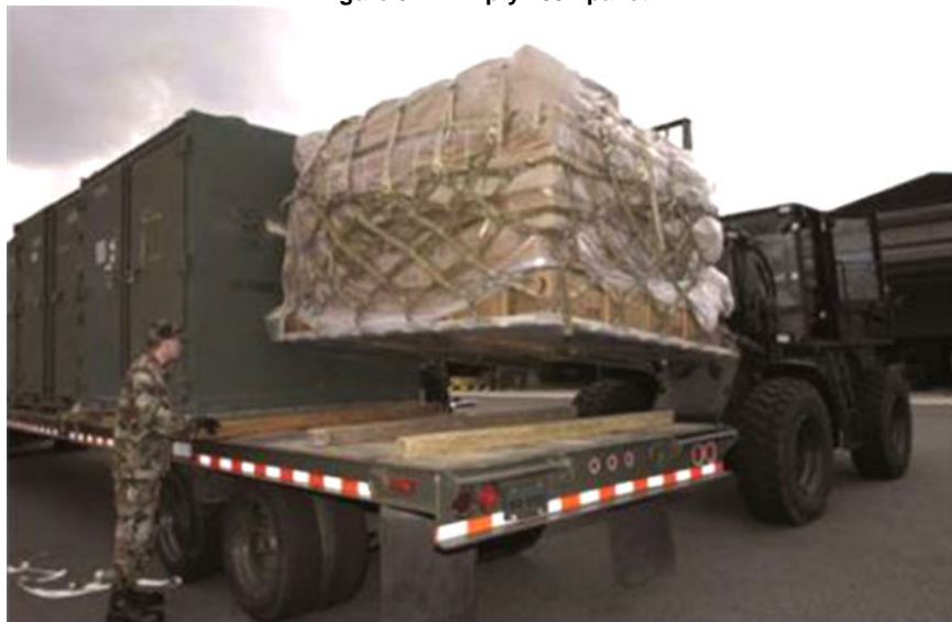
Figure 3-2. Loaded 463L pallet.
