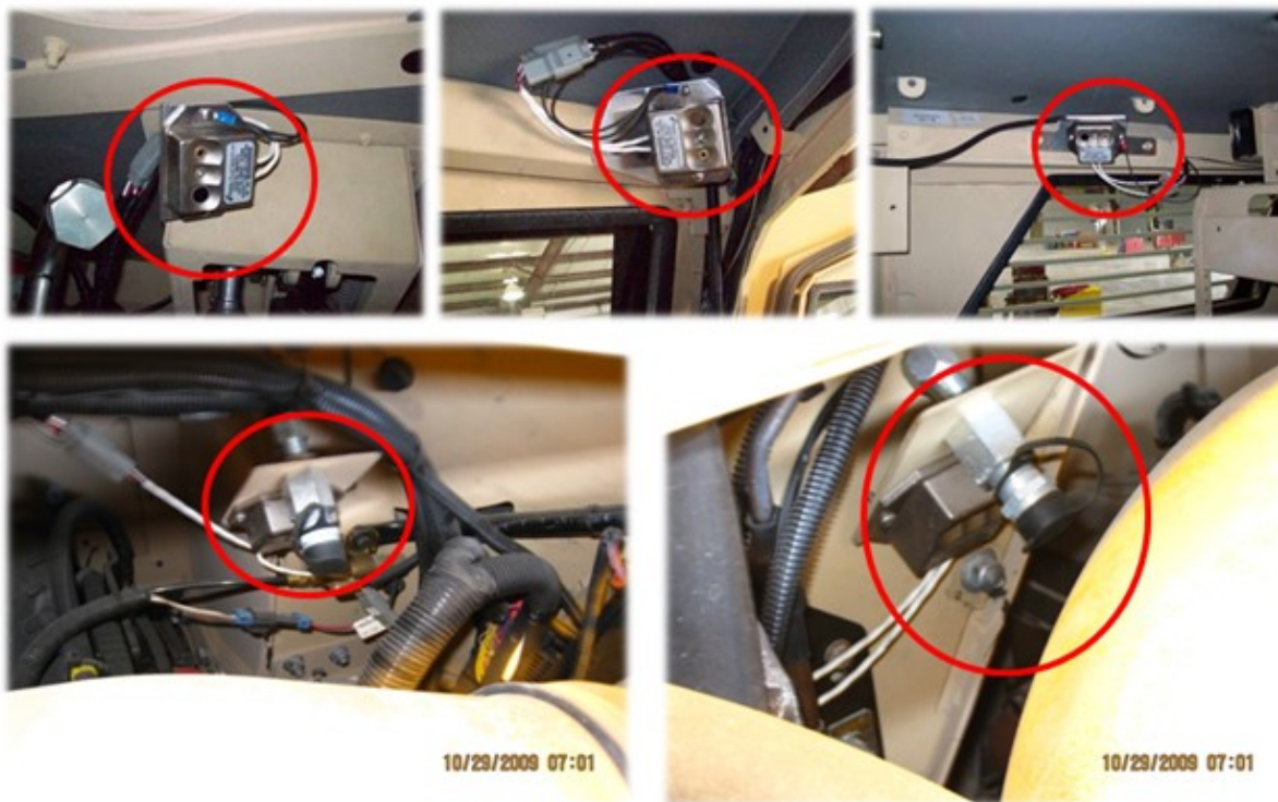
Figure 3-44. Kidde optical fire sensors.
