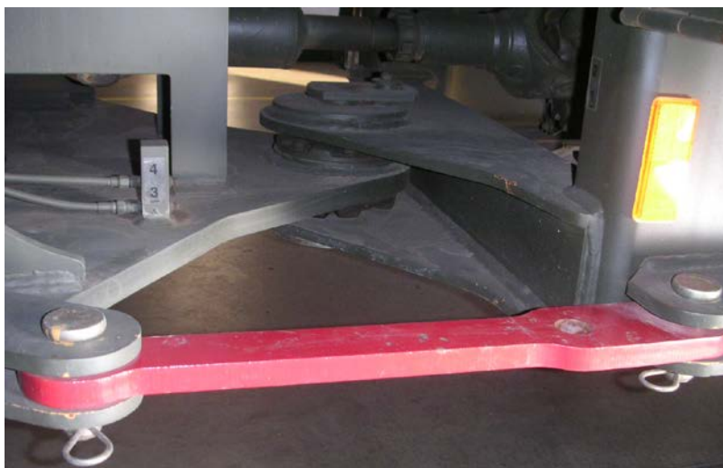
Figure 1-61. Steering frame lock link.
