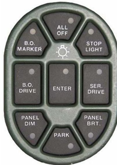
Figure 3-11. Push-button headlight switch.
