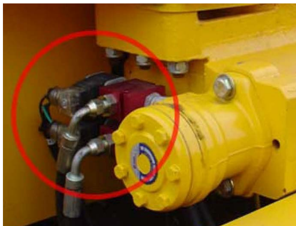
Figure 1-23. Swing cut-out solenoid valves.
