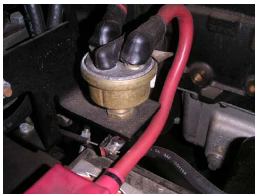
Figure 1-43. Emergency disconnect switch.
