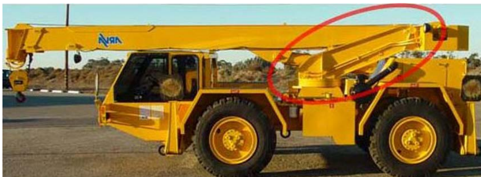
Figure 1-12. Turntable assembly.
