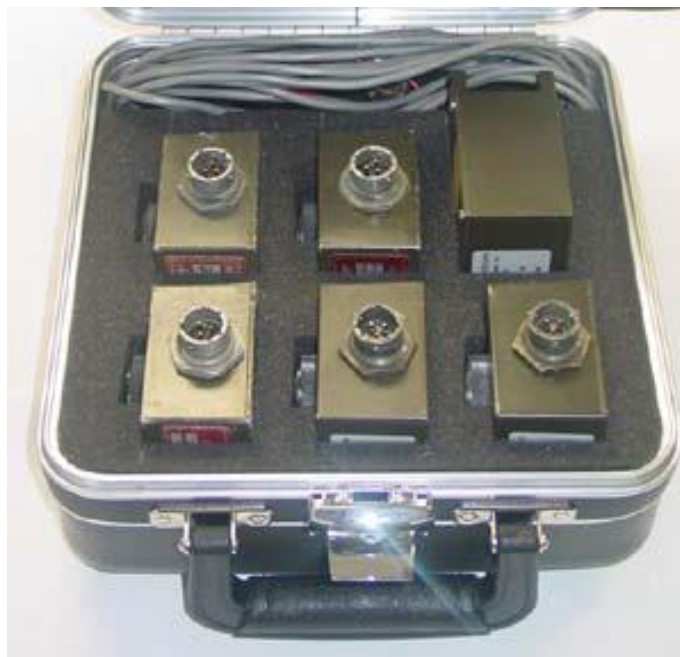
Figure 3-50. AFES test set.
