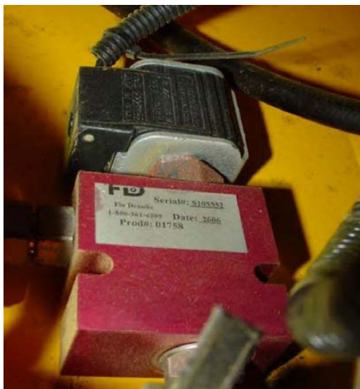
Figure 1-22. Pilot cut-out solenoid valve.
