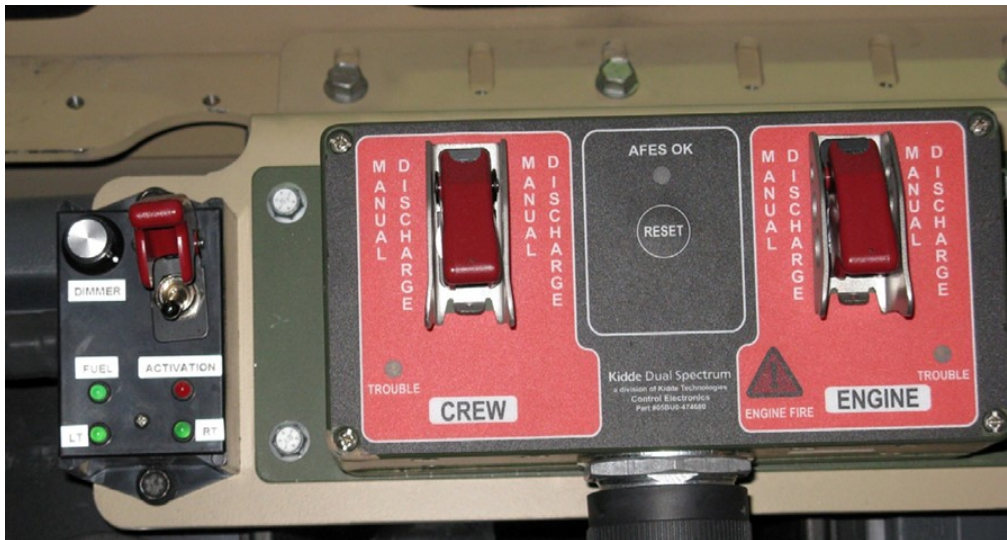
Figure 3-45. FSS control panel.
