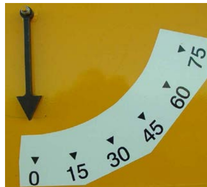
Figure 1-16. Boom angle indicator.
