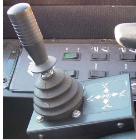
Figure 1-7. Joystick manipulator.
