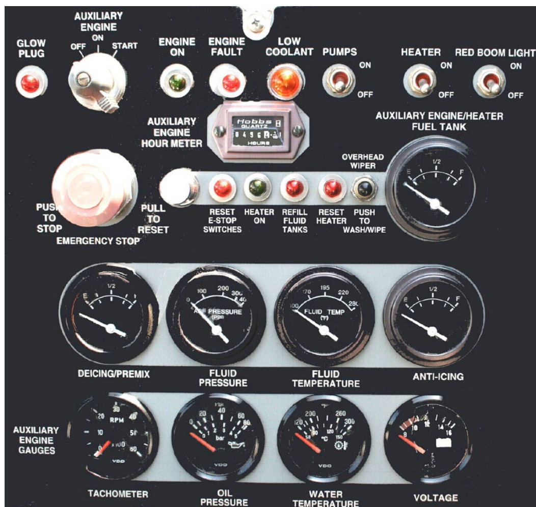
Figure 3-17. Truck control panel.
