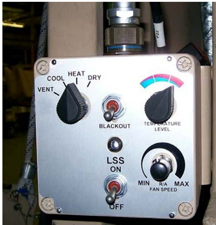
Figure 3-43. HVAC/LSS control panel.
