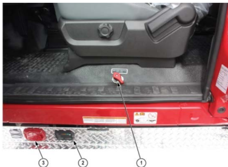
Figure 5-5. Battery switch, battery status indicator, and 110 VAC connection port.
