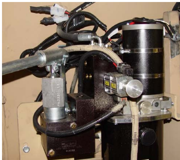
Figure 3-48. Rear door hydraulic pump assembly.
