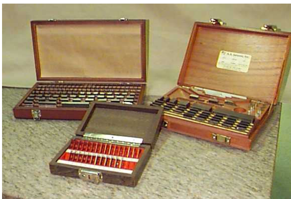
Figure 1.2-1: Gage Block Sets
