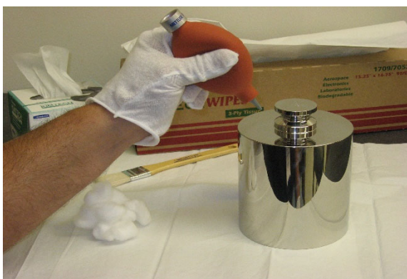
Figure 1.5-6: Cleaning the TI Using an Air Puffer
