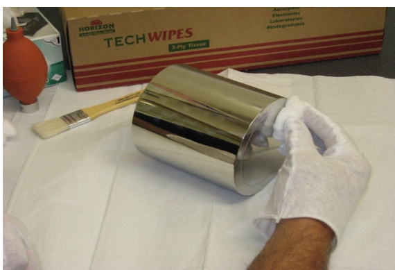
Figure 1.5-7: Cleaning the TI Using a Cotton Ball
