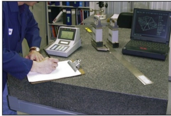
Figure 1.3-5: Electronic Leveling System
