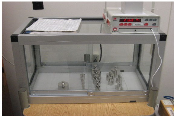
Figure 1.5-4: Mass Standards in an Enclosure
