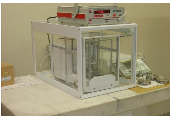
Figure 1.5-3: Balance with Draft Shield and Enclosure
