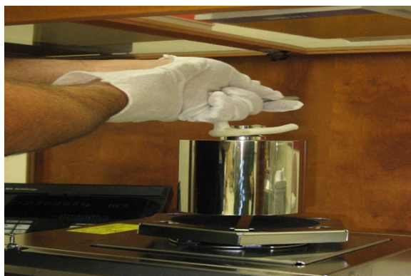
Figure 1.5-9: Leather-wrapped metal handle used to lift large weights
