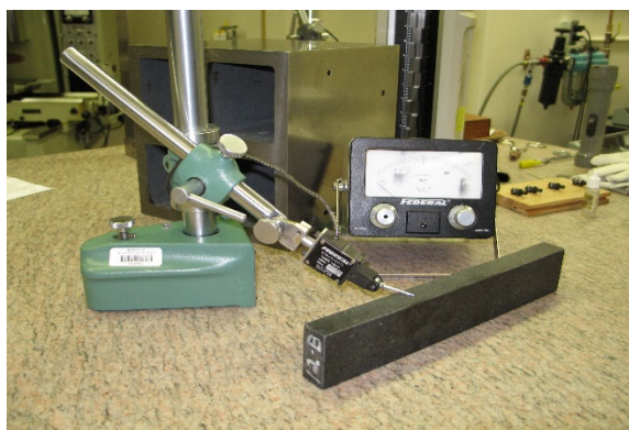
Figure 1.1-7: Straightness Measurement
