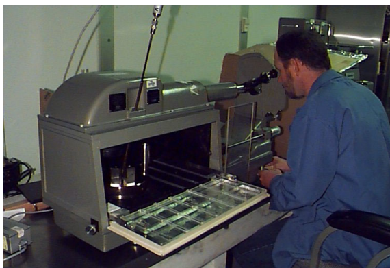
Figure 1.2-3: Interferometric Gage Block Calibration
