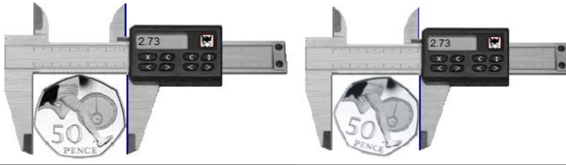
Figure 1.1-12: Ineffective way to measure roundness
