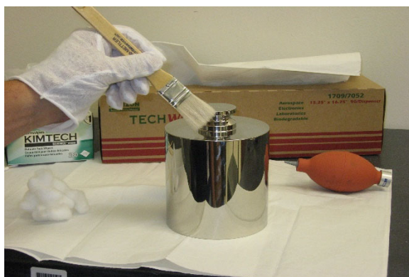
Figure 1.5-5: Cleaning the TI Using a Brush
