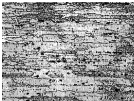
Figure 3-9. Cross section of 7075-T6 aluminum alloy.
