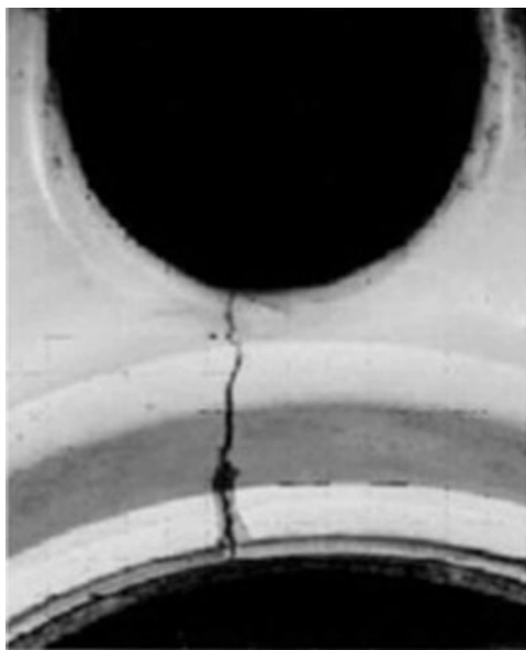
Figure 3-16. Stress cracking corrosion.
