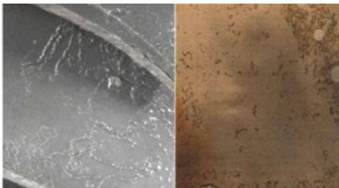
Figure 3-15. Filiform corrosion.
