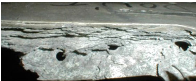
Figure 3-11. Exfoliation corrosion.
