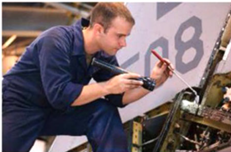
Figure 3-17. Inspection mirror usage.
