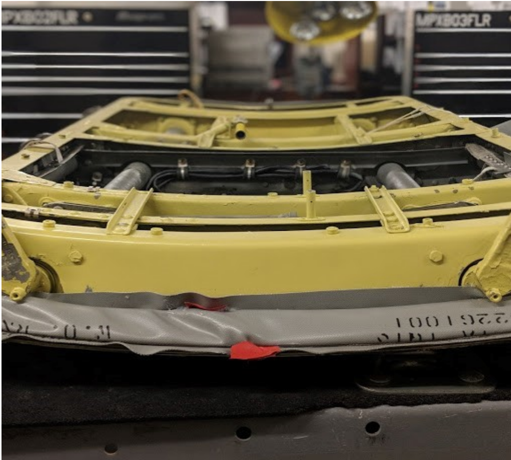
Figure 3-15. Diaphragm-type seal.
