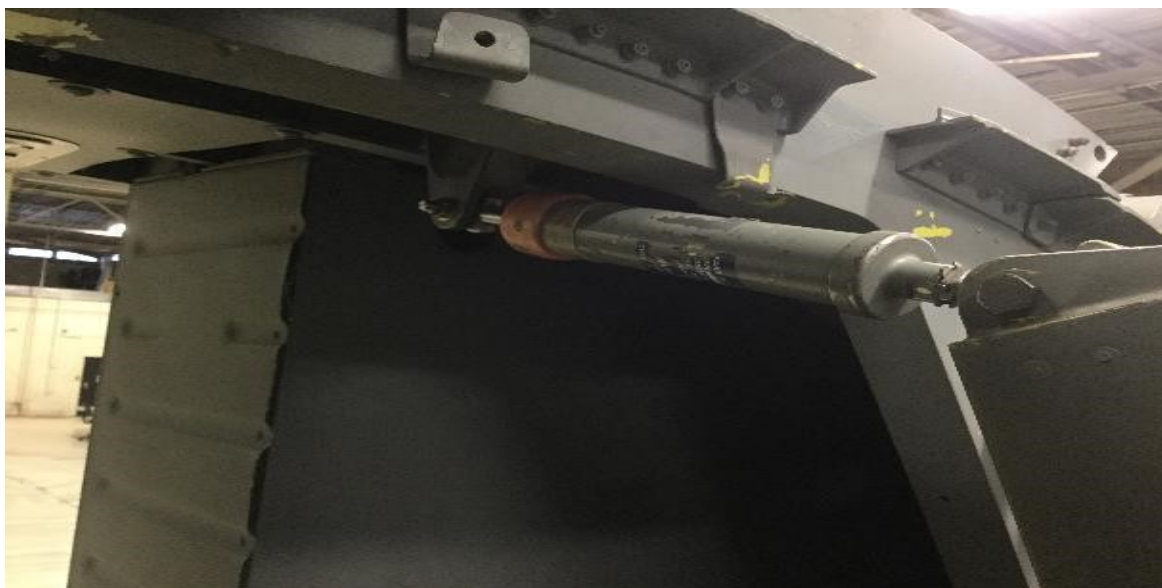
Figure 4-7. Carriage load arrestor.
