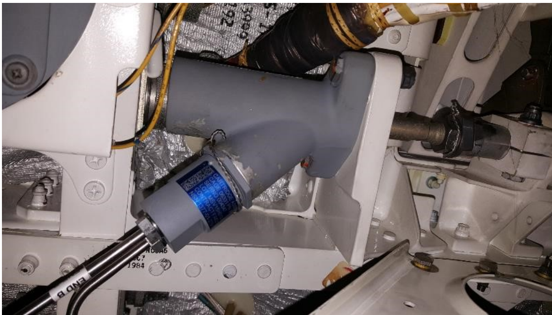
Figure 4-14. Central equipment bay (CEB) hatch pin puller.
