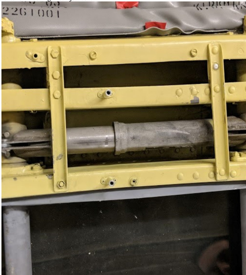
Figure 3-14. Hydraulic damper.
