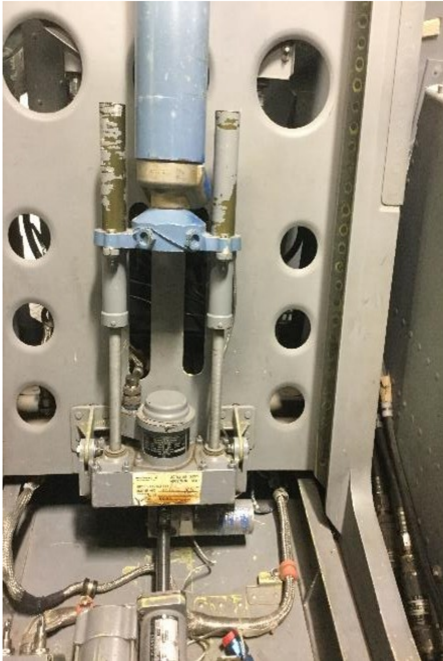
Figure 4-5. Vertical actuator.
