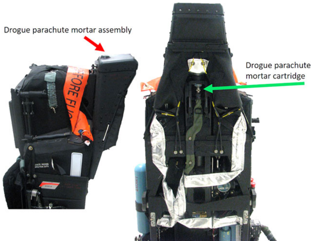
Figure 3-2. Drogue parachute mortar assembly.
