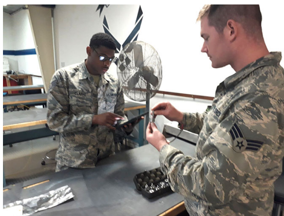
Figure 1–5. DTA/ECRL inspection gage set (go-no-go).
