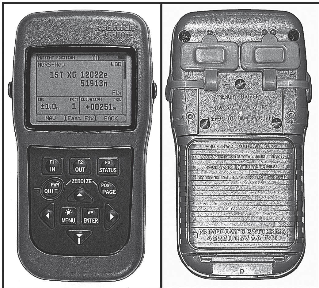
Figure I-1. Defense advanced GPS receiver (DAGR)
