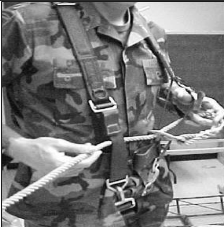
Figure 16-14. Safety Line Connected to Personnel Located on the Outside.
