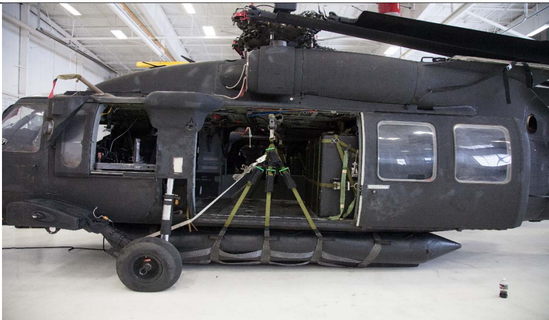
Figure 12-19. Complete K-Duck Harness with CRRC Installation.
