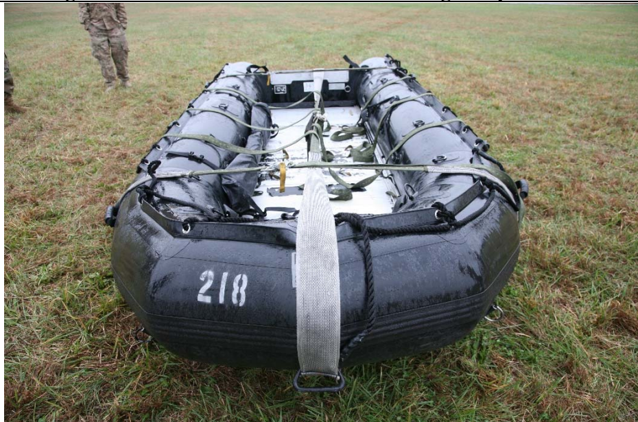
Figure 12-6. K-Duck Cradle Installed on CRRC with Restraining Straps Folded into Boat. (Bow View)
