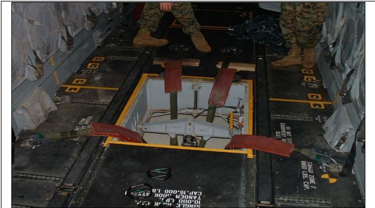
Figure 10-16. V-22 AFT Cargo Hook Hatch Opened for SPIES Operations.
