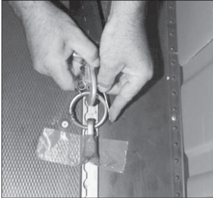
Figure 17-32. Safety wire installed through snap hook of anchor line system
