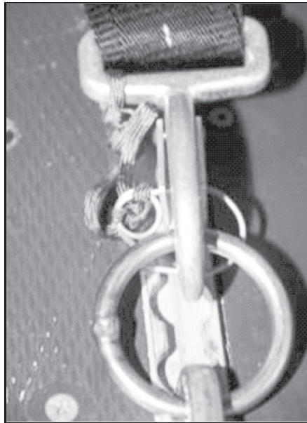
Figure 17-33. End of safety wire around snap hook of anchor line system
