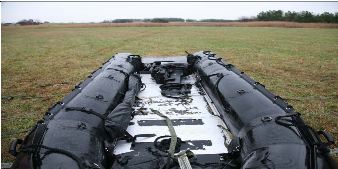
Figure 12-3. CRRC with Engine Removed from Transom (Aerial View).
