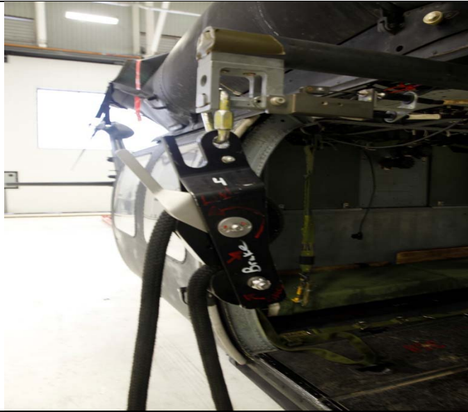
Figure 16-19. H60 AIRTEP deployment hand brake.
