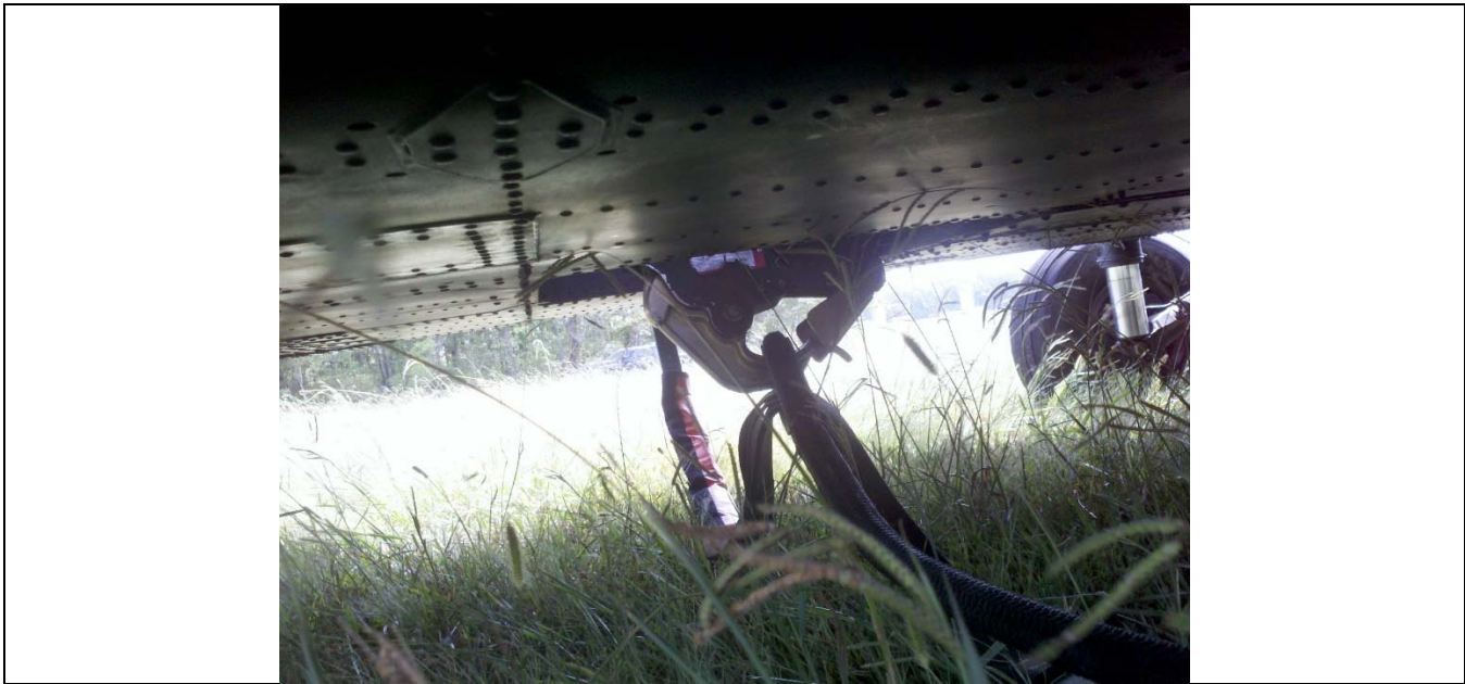
Figure 16-20. AIRTEP H-60 Cargo Hook Attachment Point.
