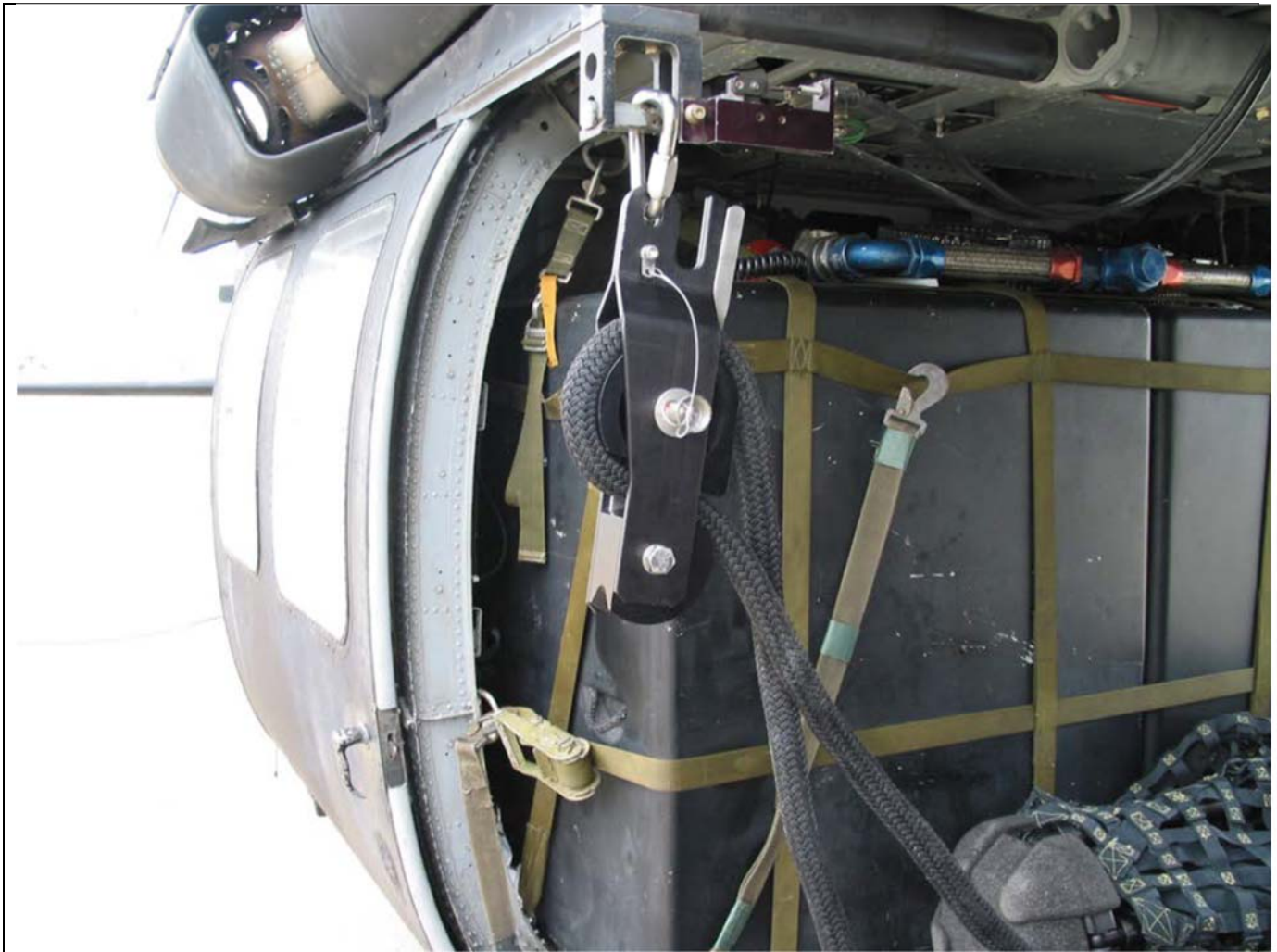
Figure 8-5. Rigging of Descent Devices.
