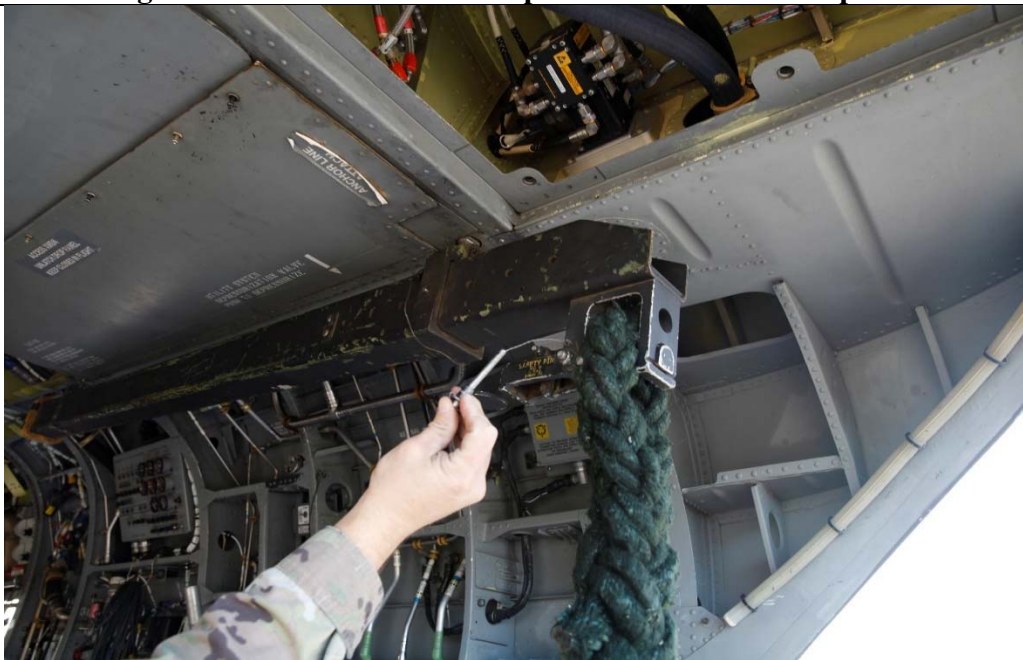
Figure 9-40. H-47 Fast Rope Attached and AFT Release Bar Seated.
