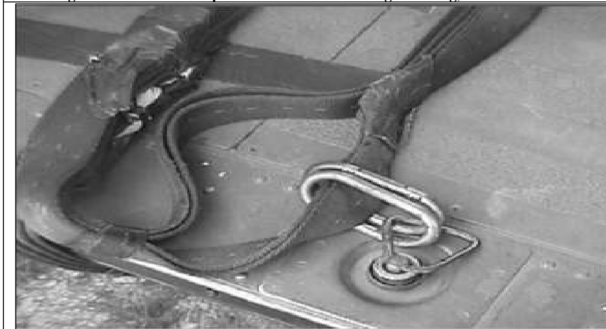
Figure 10-12. H-60. Snap Links Alternating on Strap.
