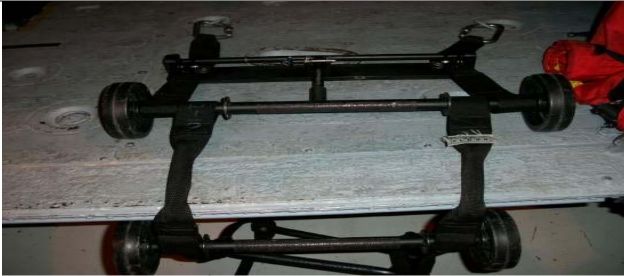
Figure 11-12. Jacobs Ladder Attached to H-60 Tie-Downs.
