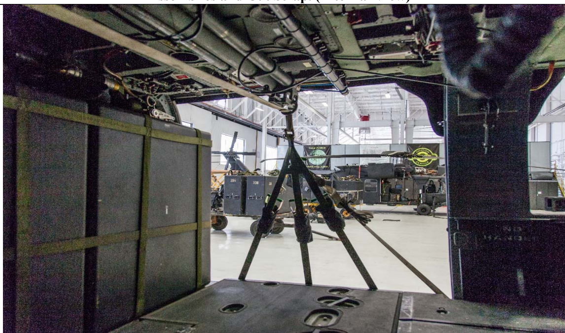
Figure 12-28. Final Installation of Crow's Foot Tensioning Assembly Cut Strap. (Internal View)
