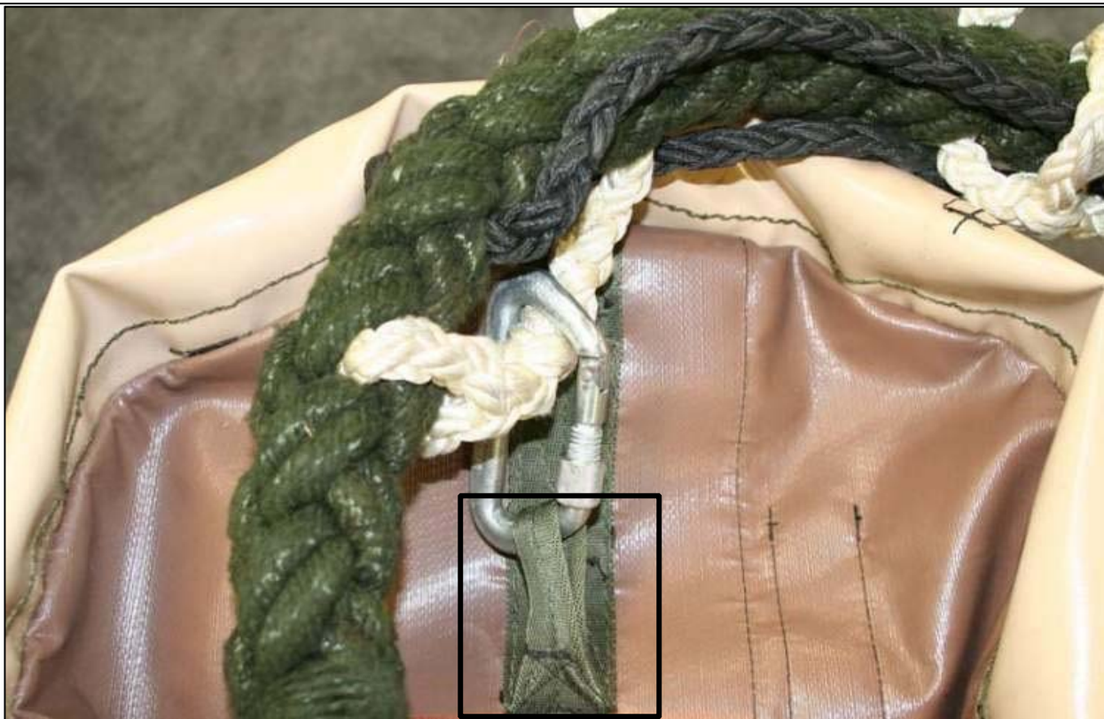
Figure 9-20. Fast Rope Attached to the Attaching Loop Inside the Fast Rope Bag.
