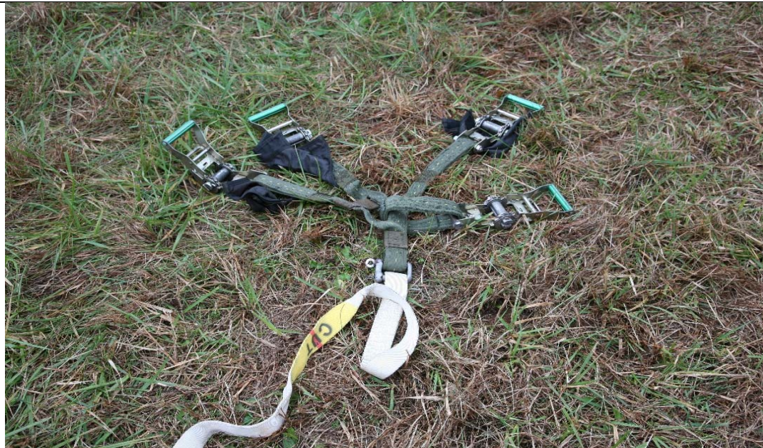
Figure 12-2. Crow's Foot Assembly Separated from Cradle.
