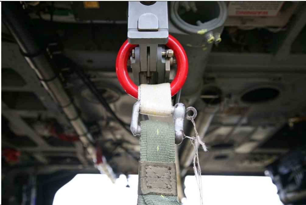
Figure 12-13. H-60. Close up of Cut Strap Routed Through FRIES H Bar. Alternate Rigging with Supplied Medium Airdrop Clevis (PS70087-2) When H Bar Ring is not Present.
