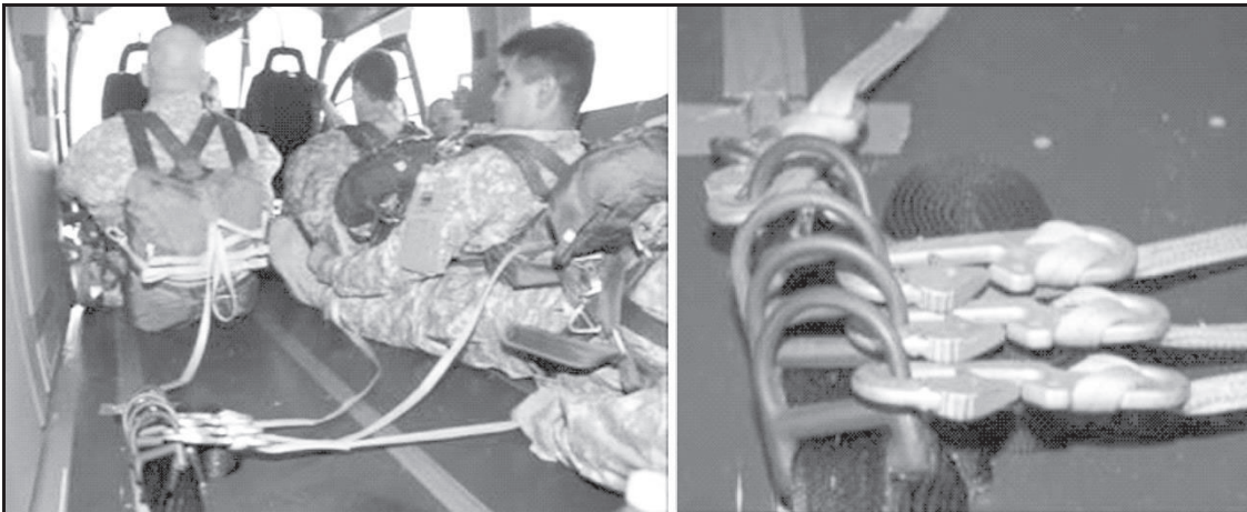
Figure 17-41. Slack retainer stowed properly
