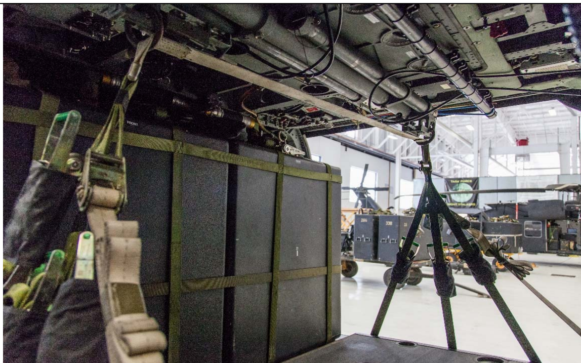
Figure 12-27. Final Installation of both Crow's Foot Tensioning Assemblies and Cut Strap. (Internal View)
