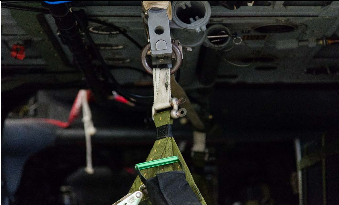
Figure 12-17. Close up of Cut Strap Routed Through FRIES H Bar. Alternate Rigging with Supplied Medium Airdrop Clevis (PS70087-2) When H Bar Ring is not Present.
