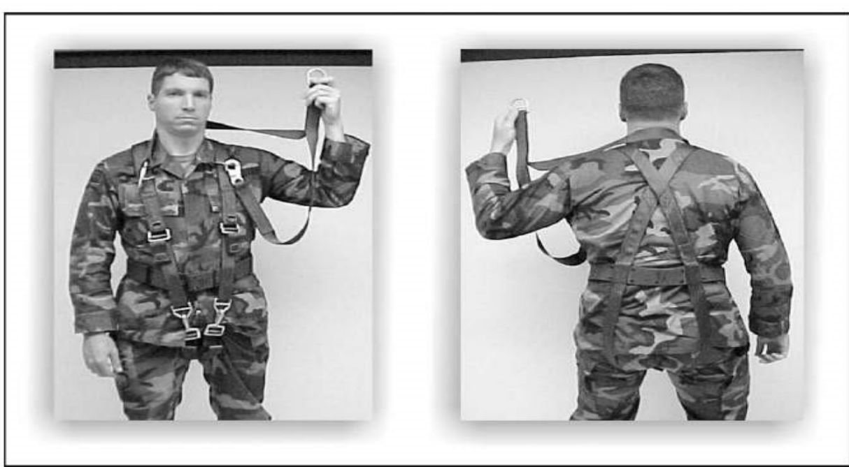
Figure 16-12. STABO Harness with Bridle.
