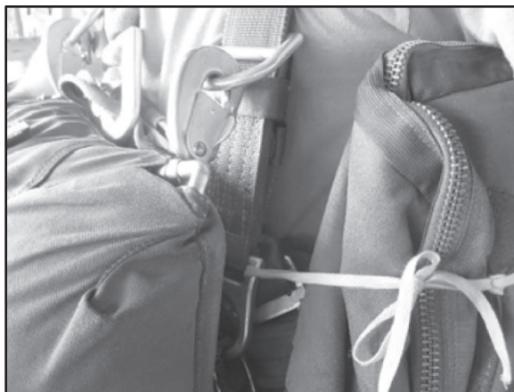
Figure 12-55. Routing the upper tie-down tape
