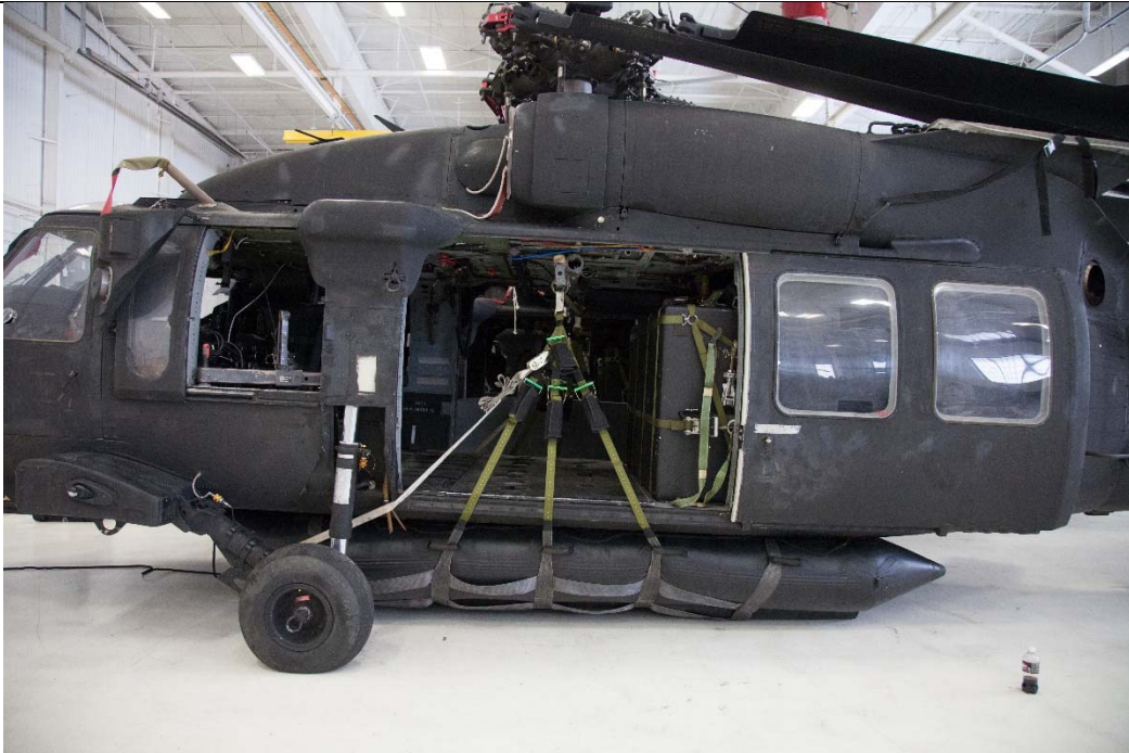
Figure 12-21. Final Installation of Crow's Foot Tensioning Assembly Showing Harness Leg Routing.
