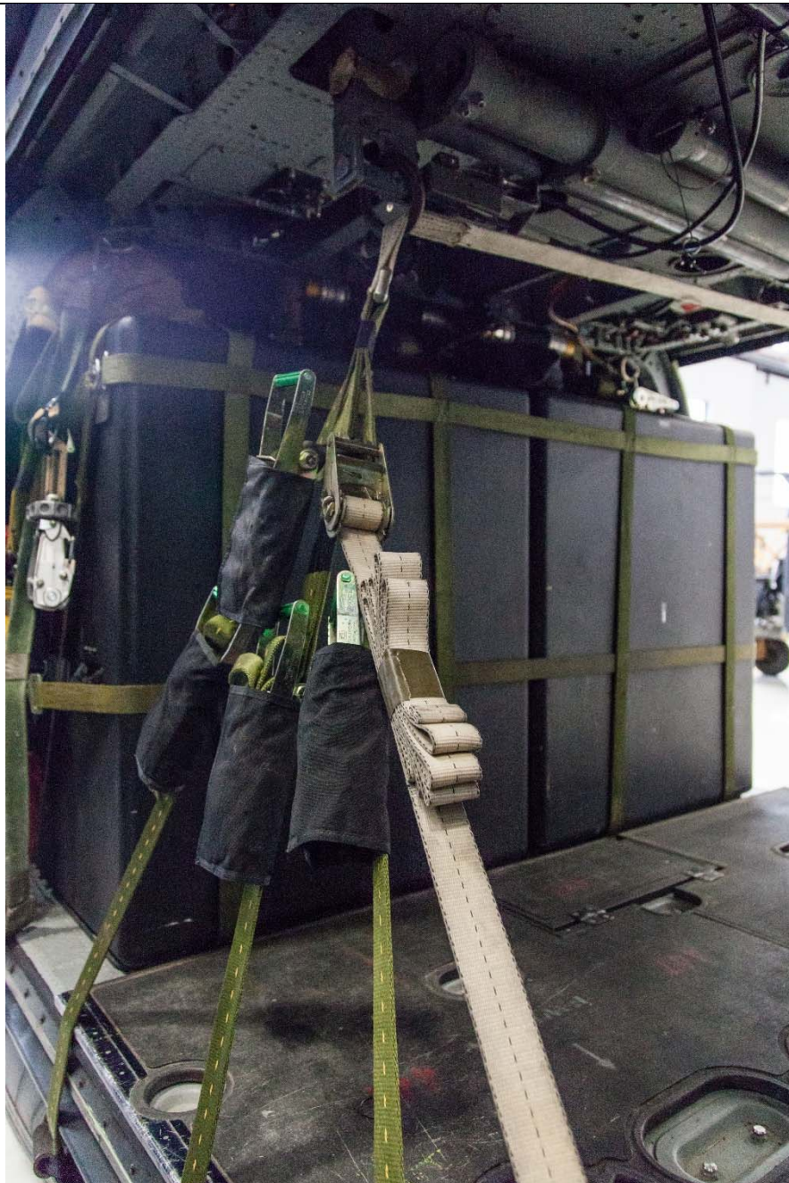
Figure 12-29. Final Installation of Crow's Foot Tensioning Assembly Highlighting Bow Strap Free End Stowage.
