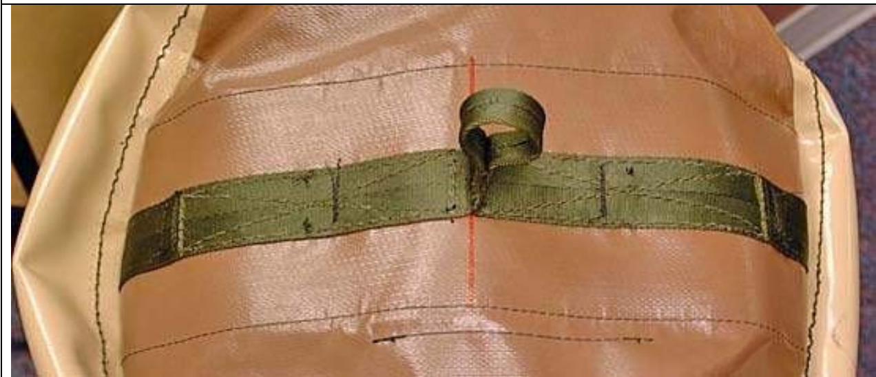
Figure 9-19. Attaching Loop.
