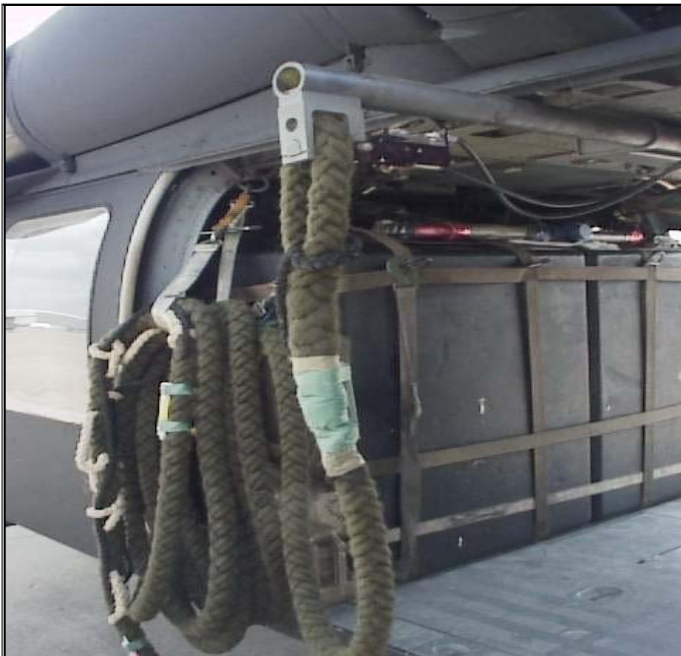
Figure 9-34. Fast Rope Attached to H-60 FRIES Bar and Fast Rope Restraint Strap Attached to Aft, Upper Tie-down Fitting.
