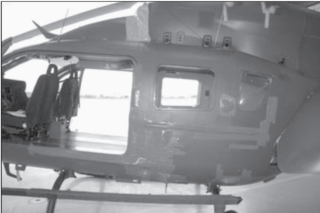
Figure 17-25. Left UH-72A Lakota exterior shown with tape and skid pad cover
