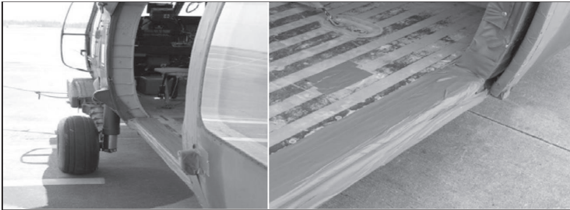
Figure 17-3. UH-60 series door edge padded and taped
