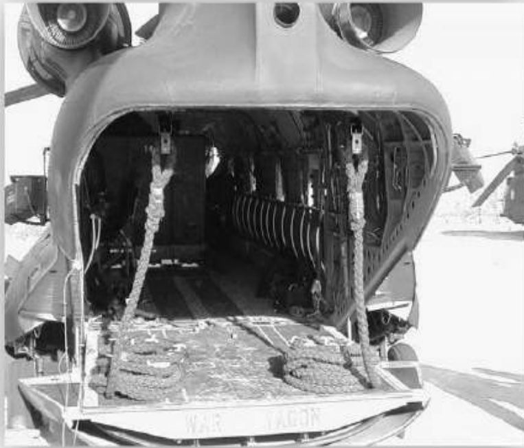
Figure 9-41. H-47 Rigged with Two AFT Fast Ropes.
