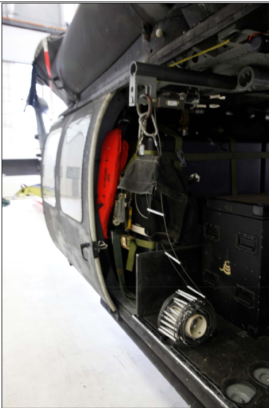
Figure 11-6. Caving Ladder Attached to FRIES Bar (H-60).
