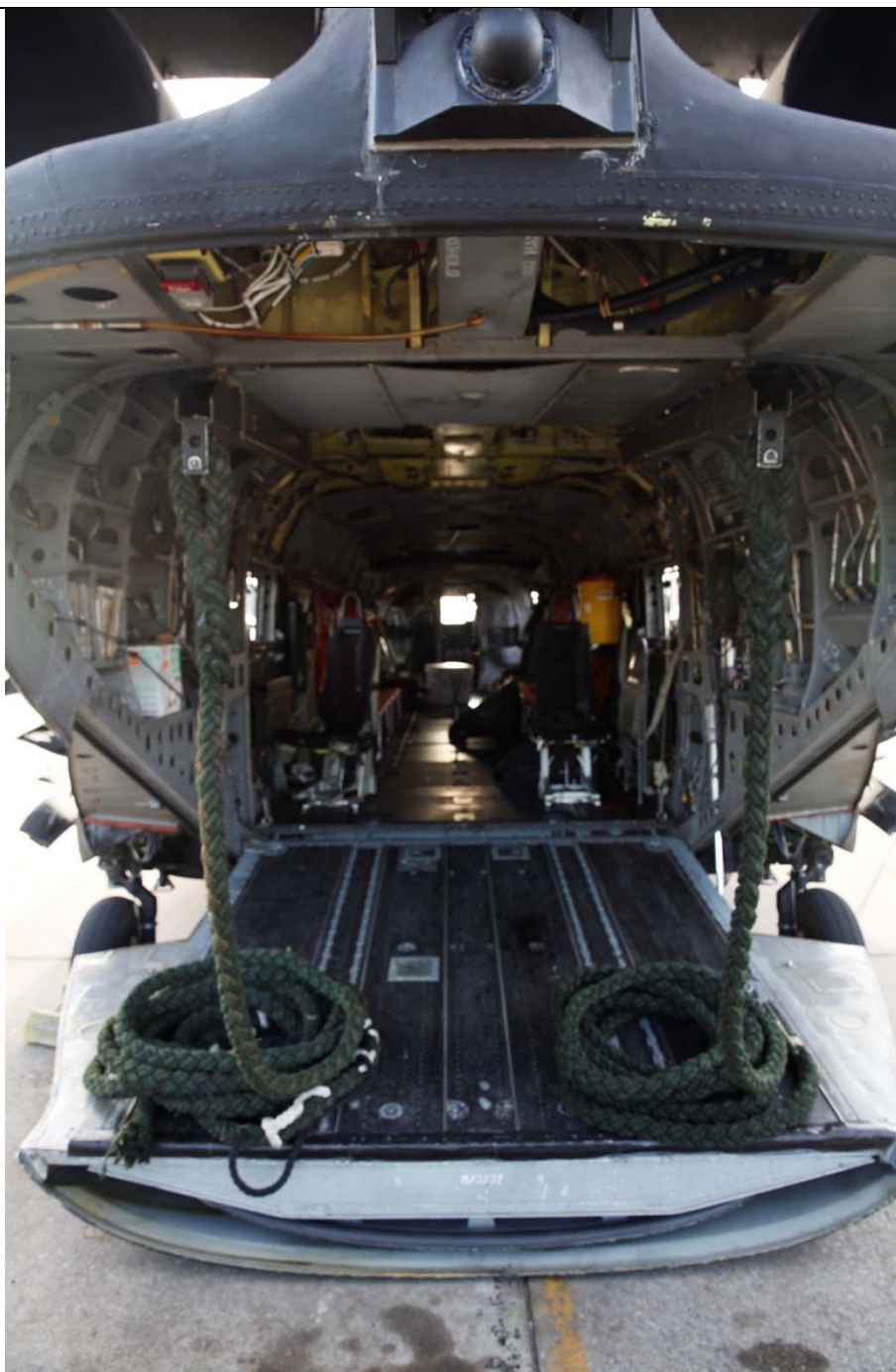
Figure 9-10. FRIES Bars Assembly (AFT).
