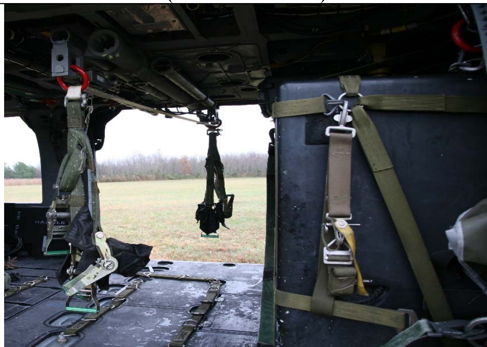
Figure 12-12. Cut Strap and Crow's Foot Assemblies Prepared for Attachment to Cradle.
