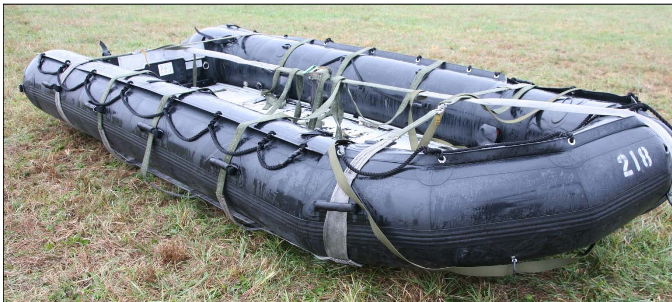
Figure 12-11. K-Duck Cradle Installed on CRRC with Restraining Straps Folded into Boat. (Starboard/Bow View)
