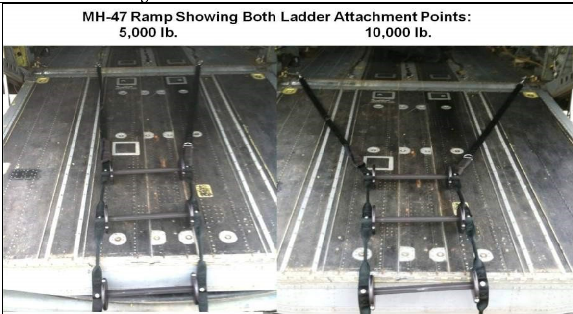
Figure 11-11. Nylon Ladder Connected to 5,000 and 10,000-Pound Cargo Tie-Downs of the H-47.
