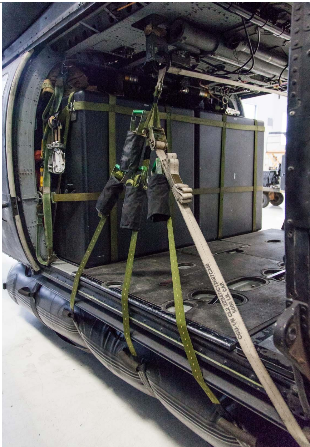
Figure 12-30. Final Installation of Crow's Foot Tensioning Assembly Showing Harness Leg Routing.
