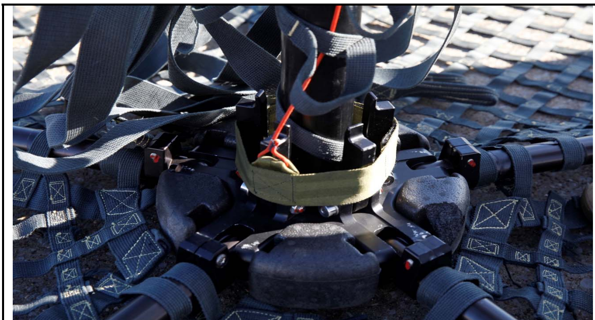
Figure 16-22. AIRTEP lower Platform Lock Disengaged.
