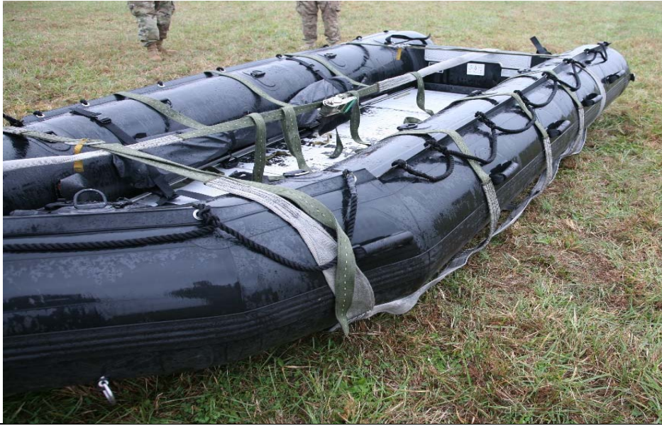
Figure 12-7. K-Duck Cradle Installed on CRRC with Restraining Straps Folded into Boat. (Port/Bow View)
