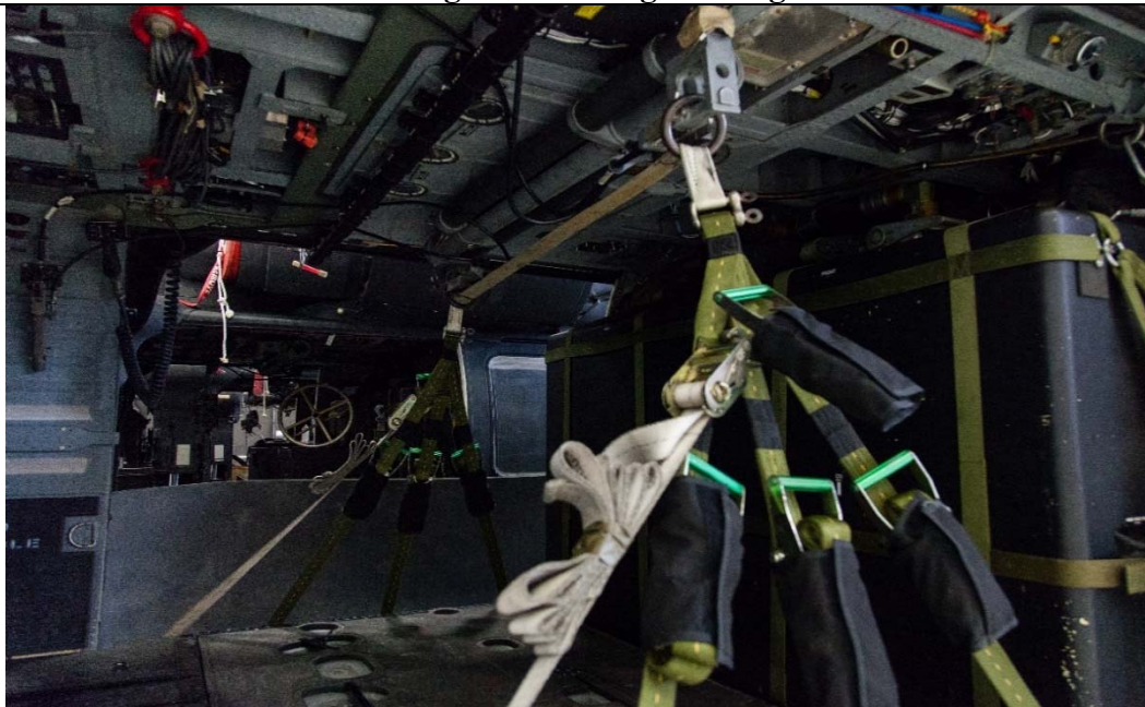
Figure 12-22. Close up of Final Assembly of Crow's Foot Tensioning Assembly Showing Routing of Cut Strap. (Front Angle)
