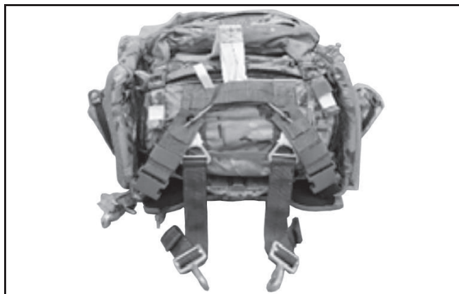
Figure 12-46. Assembled integrated-harness, single point release using the adjustable D-ring attaching straps
