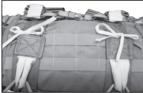
Figure 12-42. Securing HSPR with quarter-inch cotton webbing to M7
