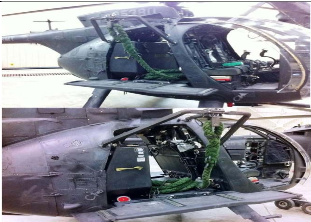
Figure 9-35. Fast Rope Rigged on an MH-6.
