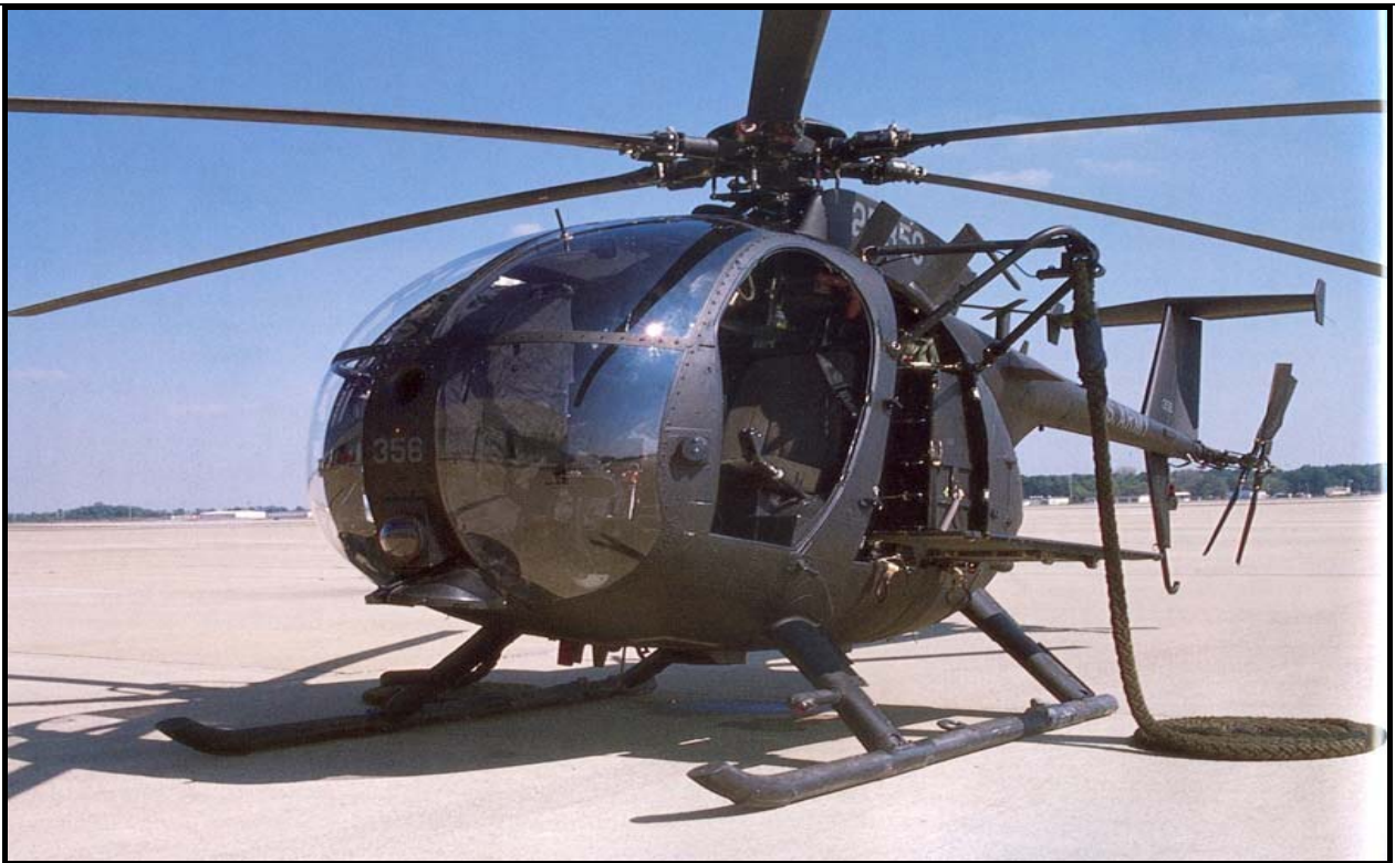
Figure 9-36. MH-6 Fast Rope Rigging
