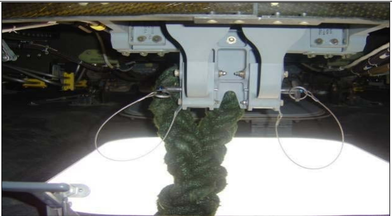
Figure 9-14. Fast Rope Attachment Point with Rope on V-22.
