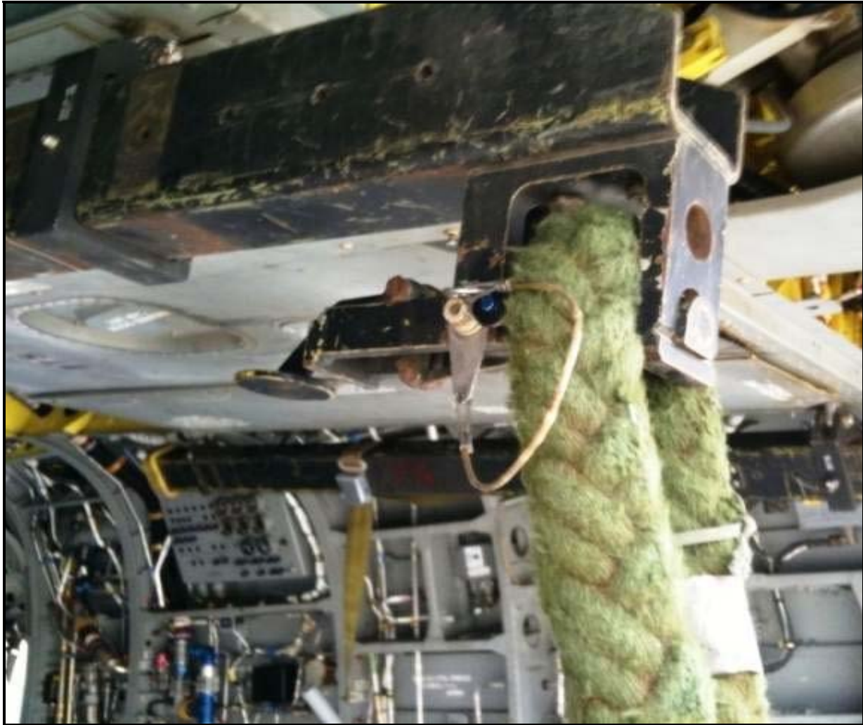
Figure 9-9. H-47 Air Force Tactics (AFT) Quick Release Pin Inserted.
