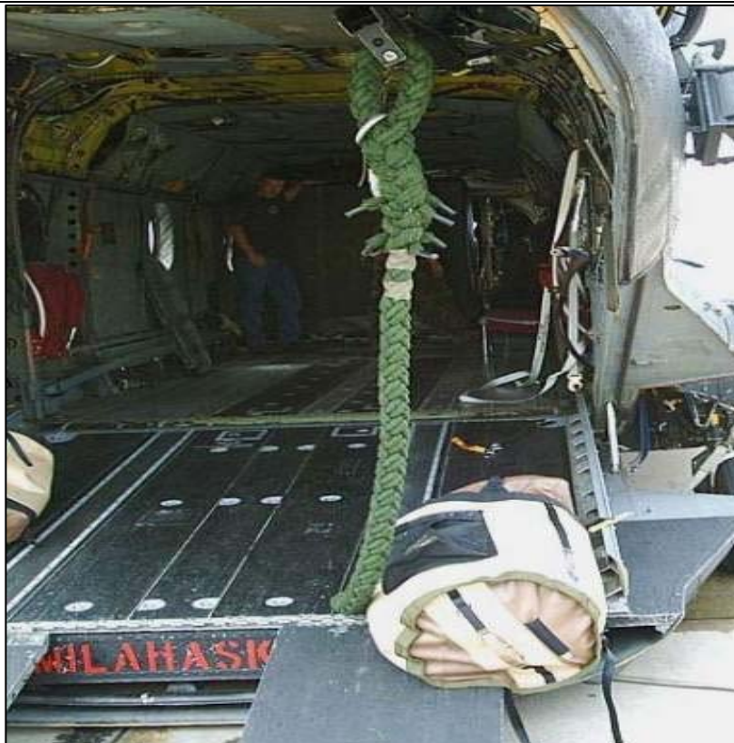
Figure 9-38. Fast Rope Attached to the FRIES Bar on the H-47 Helicopter.
