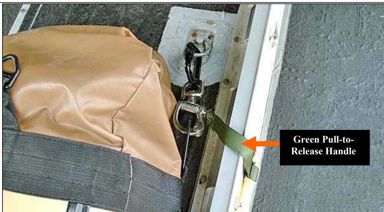
Figure 9-28. Primary Snap Shackle with Green Pull-to-Release Handle.
