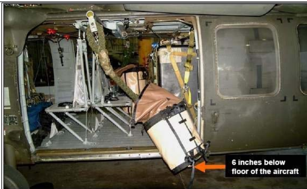
Figure 9-7. H-60 Small Bag Attached to FRIES.
