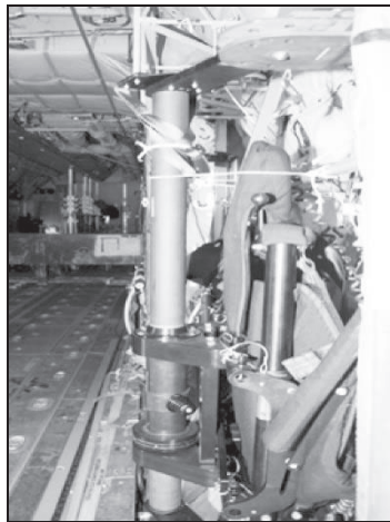
Figure 16-9. Crash worthiness seat with Type III nylon cord
