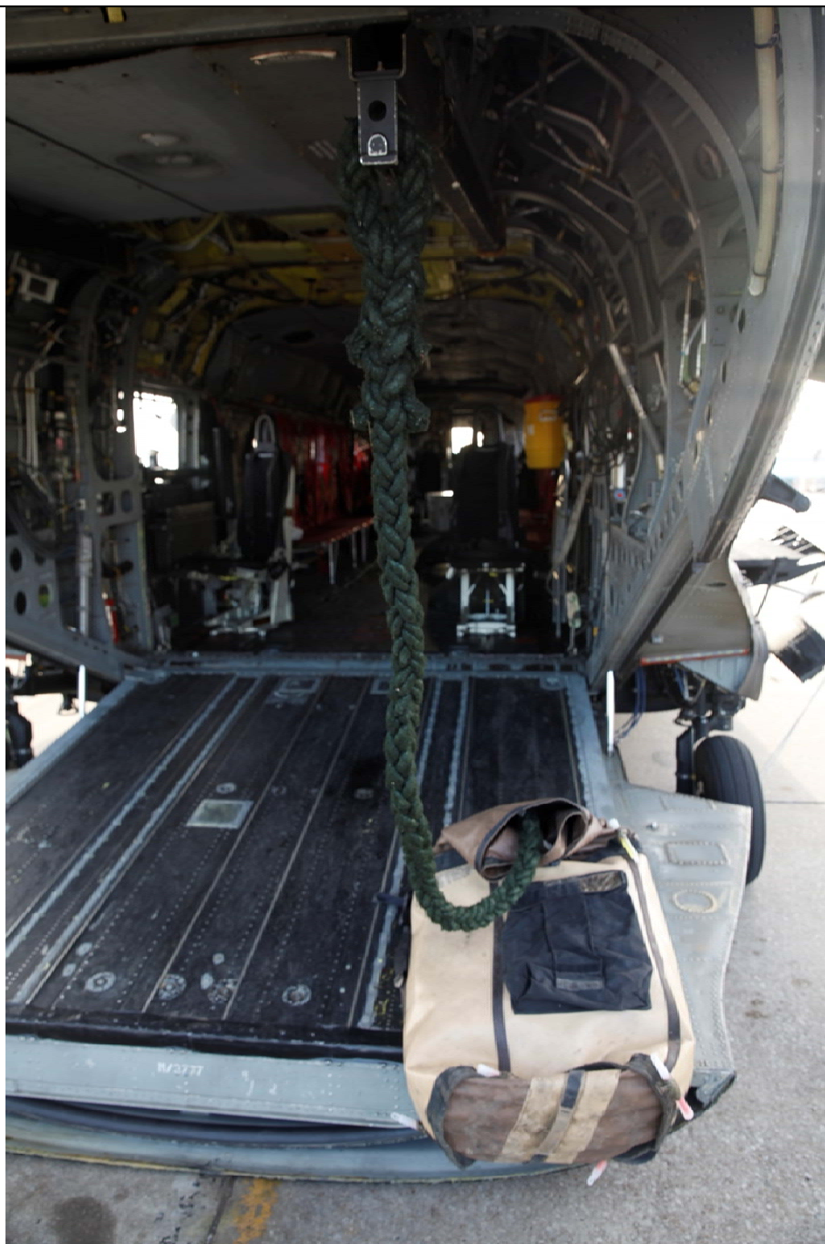
Figure 9-12. FRIES Rope Bag Assembly.
