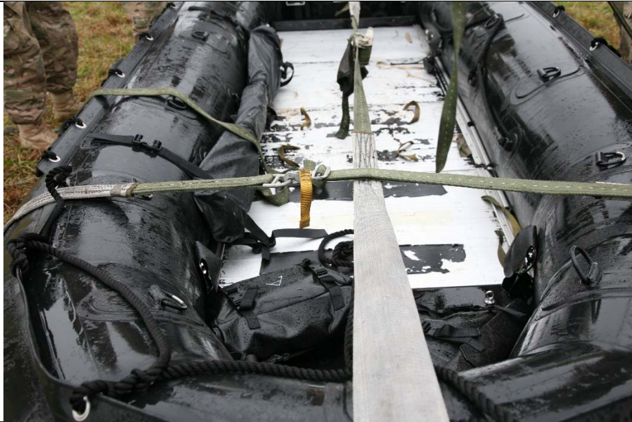
Figure 12-5. Front Cradle/CRRC Securing Strap Installed.
