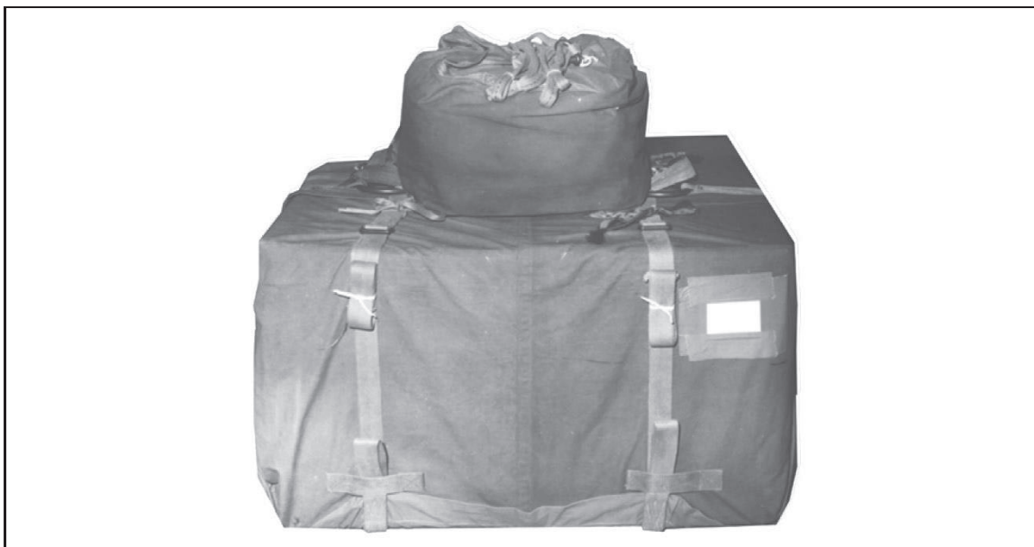
Figure 14-9. Container load rigged for low-velocity paratroop door airdrop
