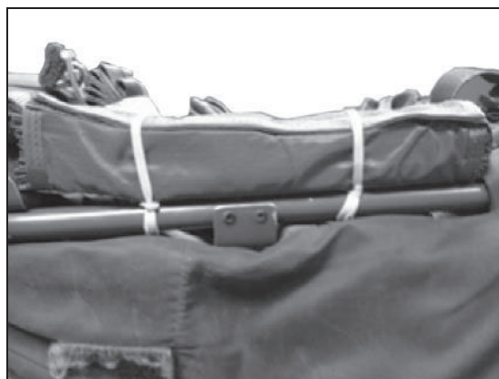
Figure 12-33. Placement of retainer band
