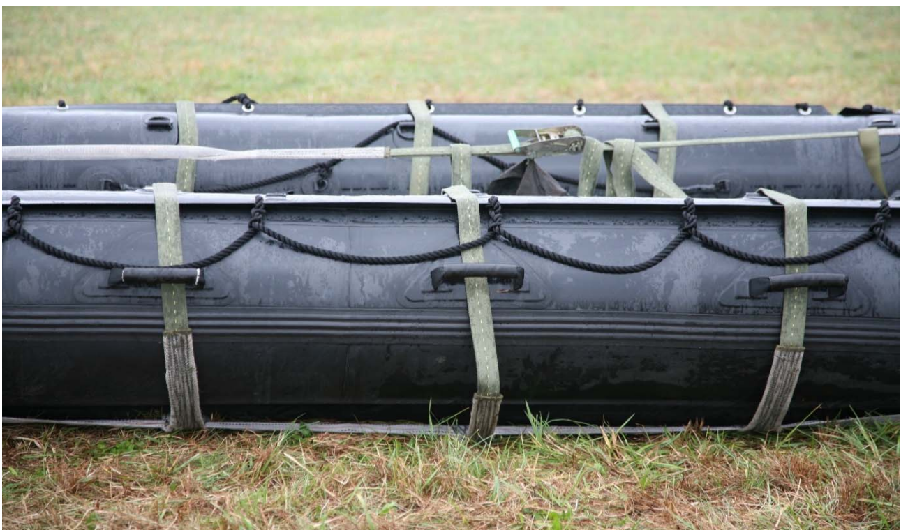
Figure 12-9. K-Duck Cradle Installed on CRRC with Restraining Straps Folded into Boat. (Starboard View)
