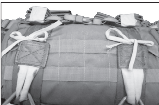
Figure 12-37. Securing HSPR with quarter-inch cotton webbing to MAP
