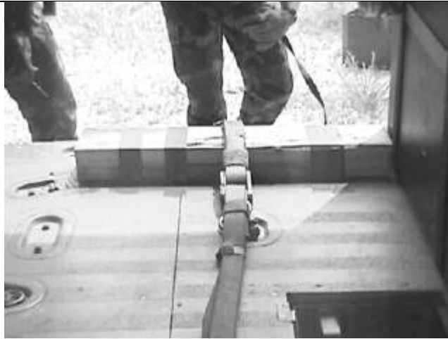
Figure 10-8. H-60 Placement of Wood Block.
