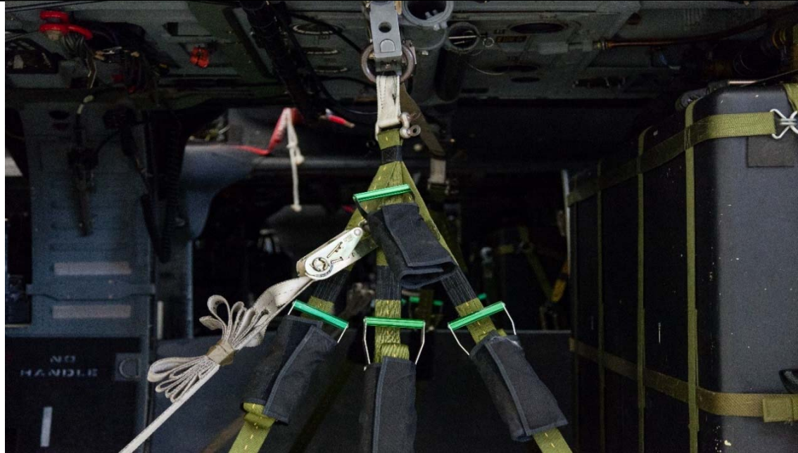
Figure 12-18. Close up of Final Assembly of Crow's Foot Tensioning Assembly.
