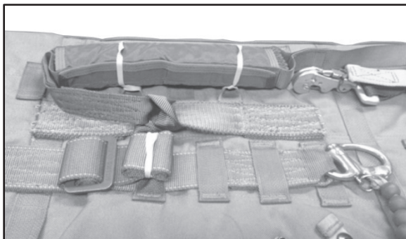
Figure 12-56. Attachment of HPTLL to the MAWC
