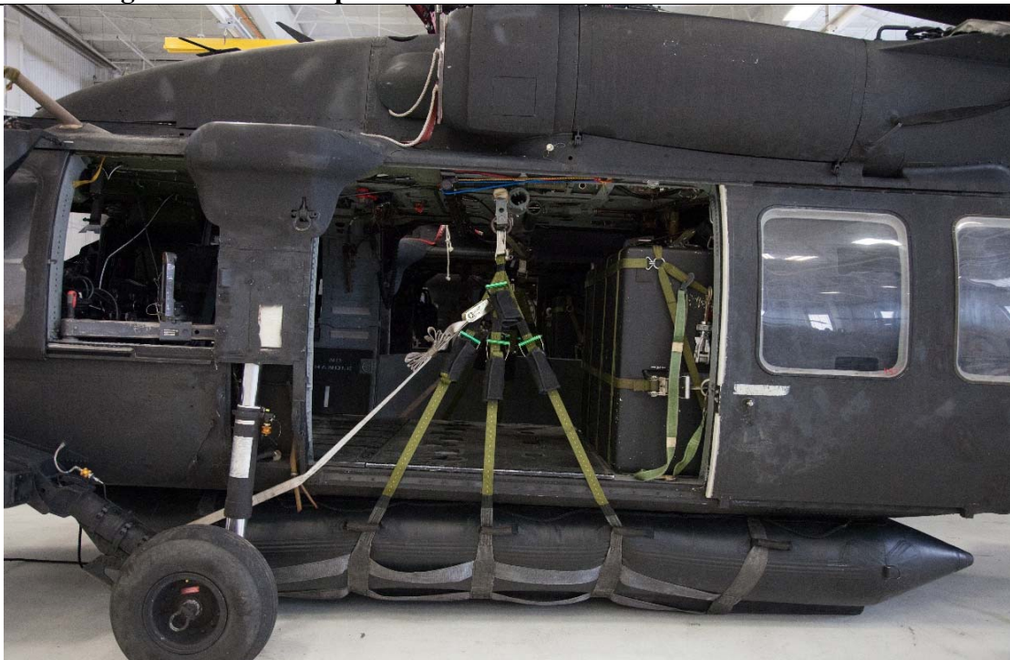
Figure 12-20. Final Installation of Crow's Foot Tensioning Assembly Showing Harness Leg Routing.
