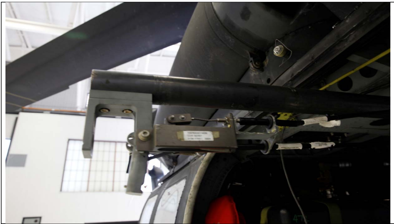
Figure 9-6. H-60 Fast Rope Bar Attachment Point Extended (Outside Aircraft).
