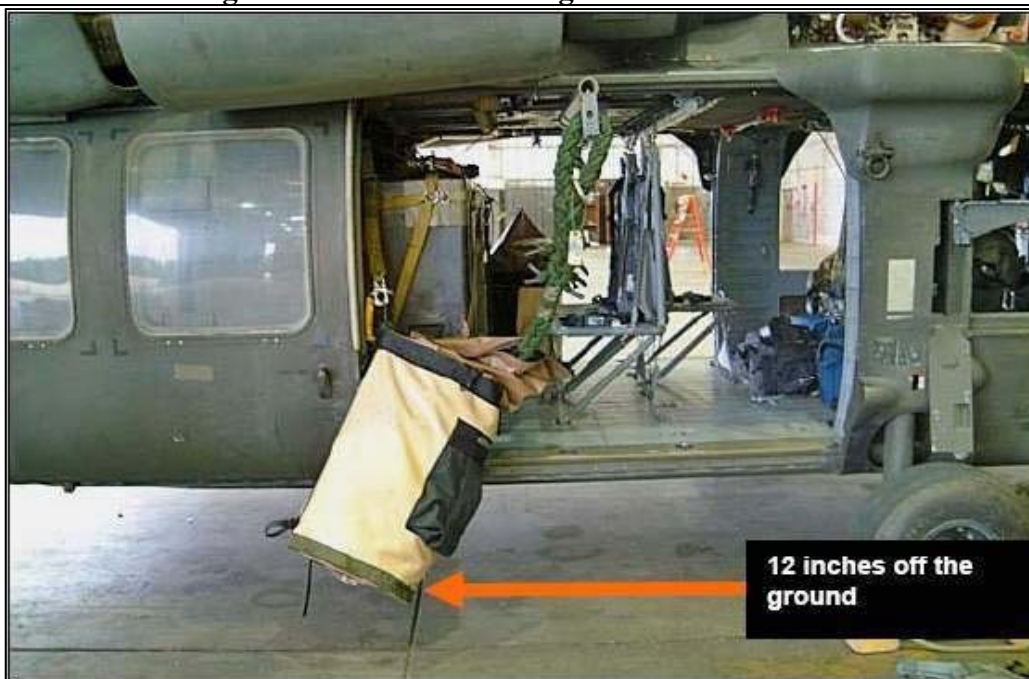
Figure 9-8. H-60 Large Bag Attached to FRIES.
