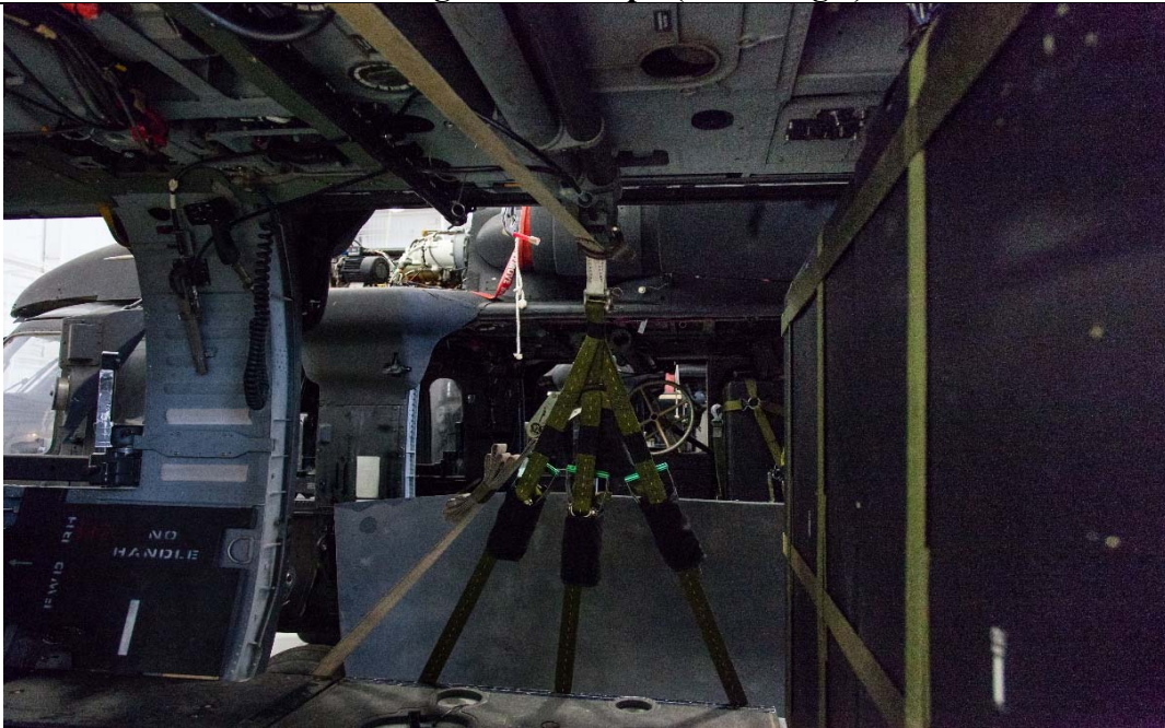
Figure 12-24. Final Installation of Crow's Foot Tensioning Assembly Cut Strap. (Internal View)
