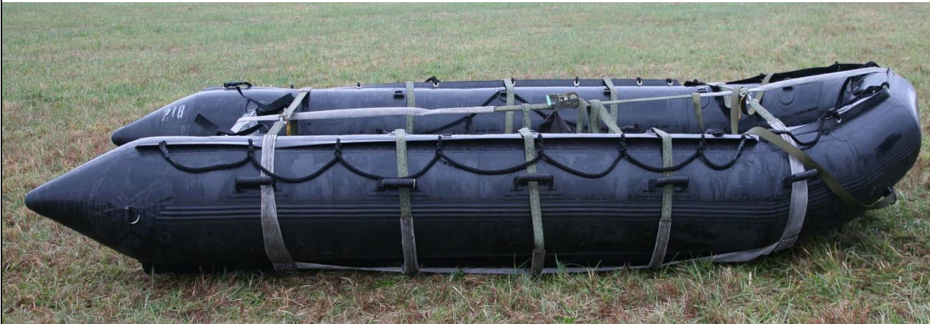
Figure 12-9. K-Duck Cradle Installed on CRRC with Restraining Straps Folded into Boat. (Starboard View)
