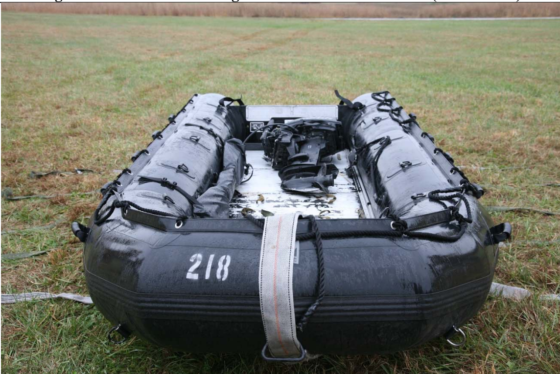
Figure 12-4. CRRC with Engine Removed from Transom (Bow View).
