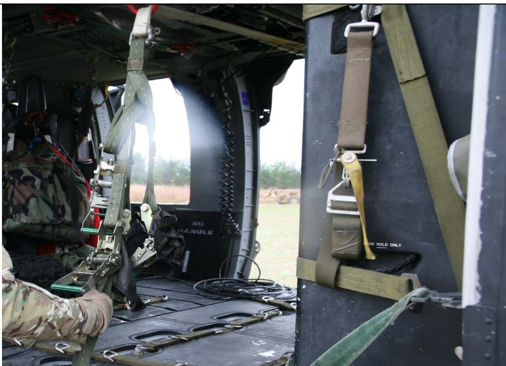
Figure 12-15. Attaching Restraint Slings from Cradle to Crow's Foot Assembly.
