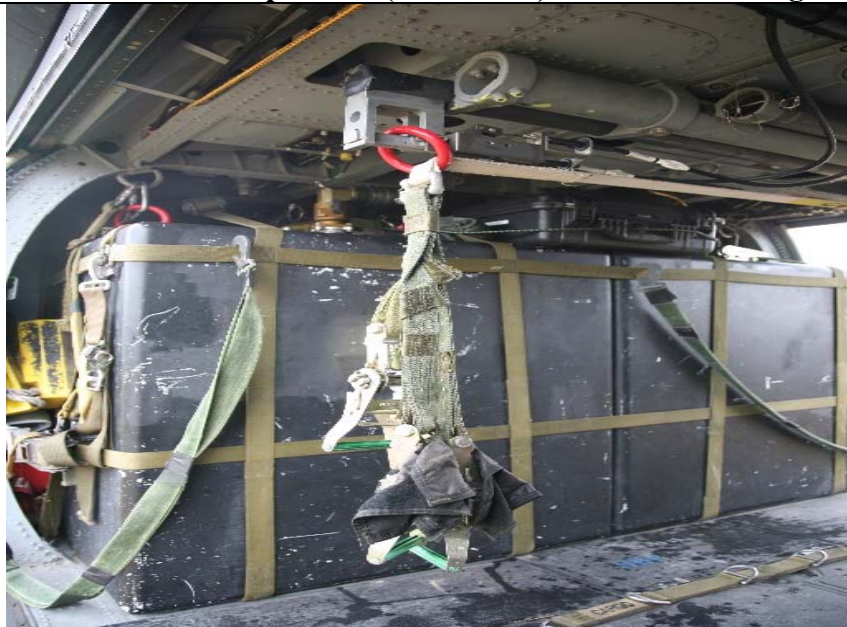
Figure 12-14. Cut Strap and Crow's Foot Assemblies Prepared for Attachment to Cradle. (Left Side)
