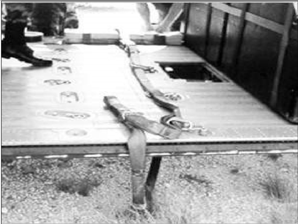
Figure 10-10. H-60 Placement of Four Pairs of Snap Links.
