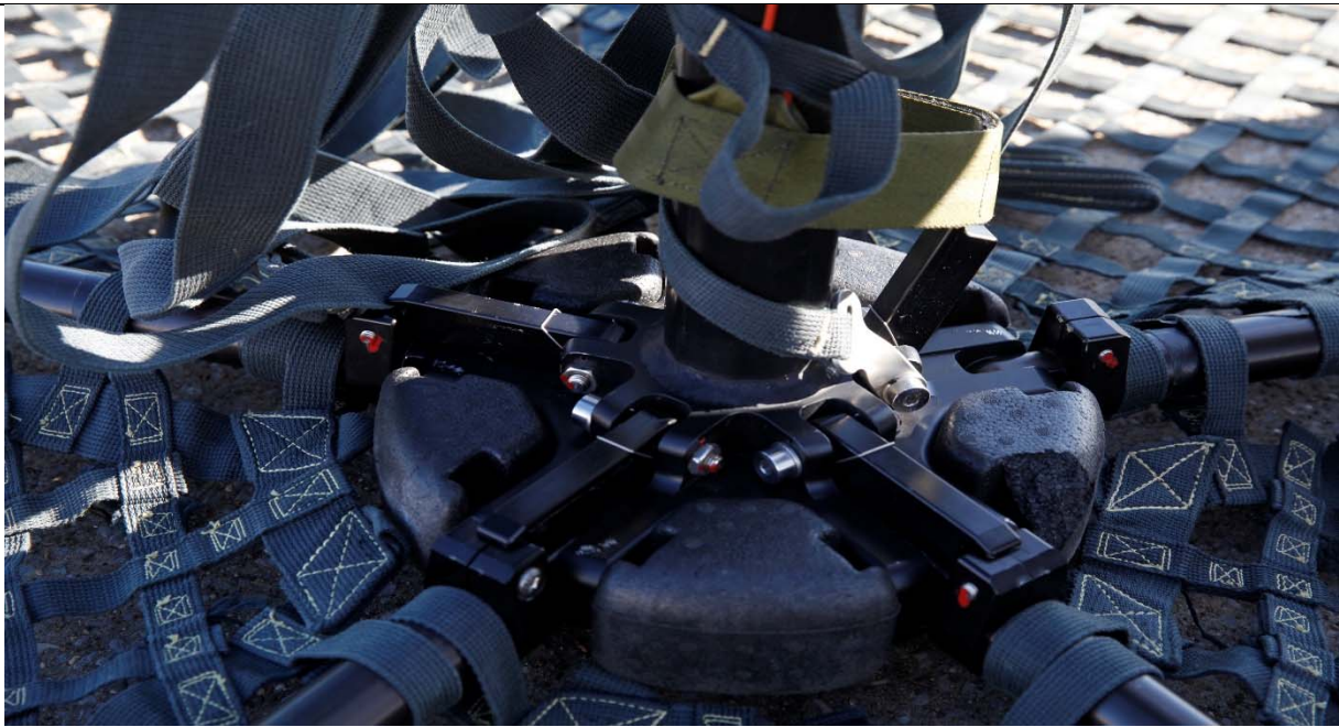
Figure 16-23. AIRTEP Lower Platform Lock Engaged.
