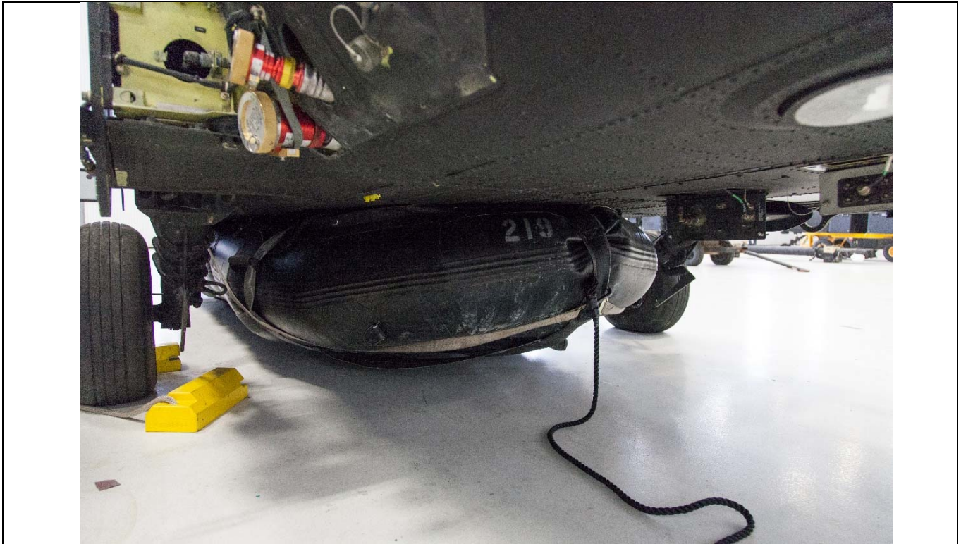
Figure 12-31. Final Installation of CRRC to “Belly” of H-60 Aircraft.
