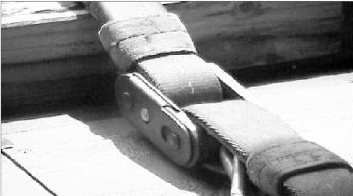
Figure 10-9. H-60 Placement of Type IV Link.
