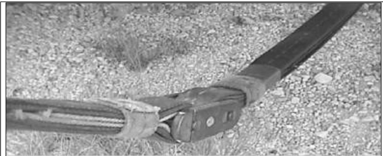
Figure 10-5. H-60 Suspension Slings Connected by Type IV Links.
