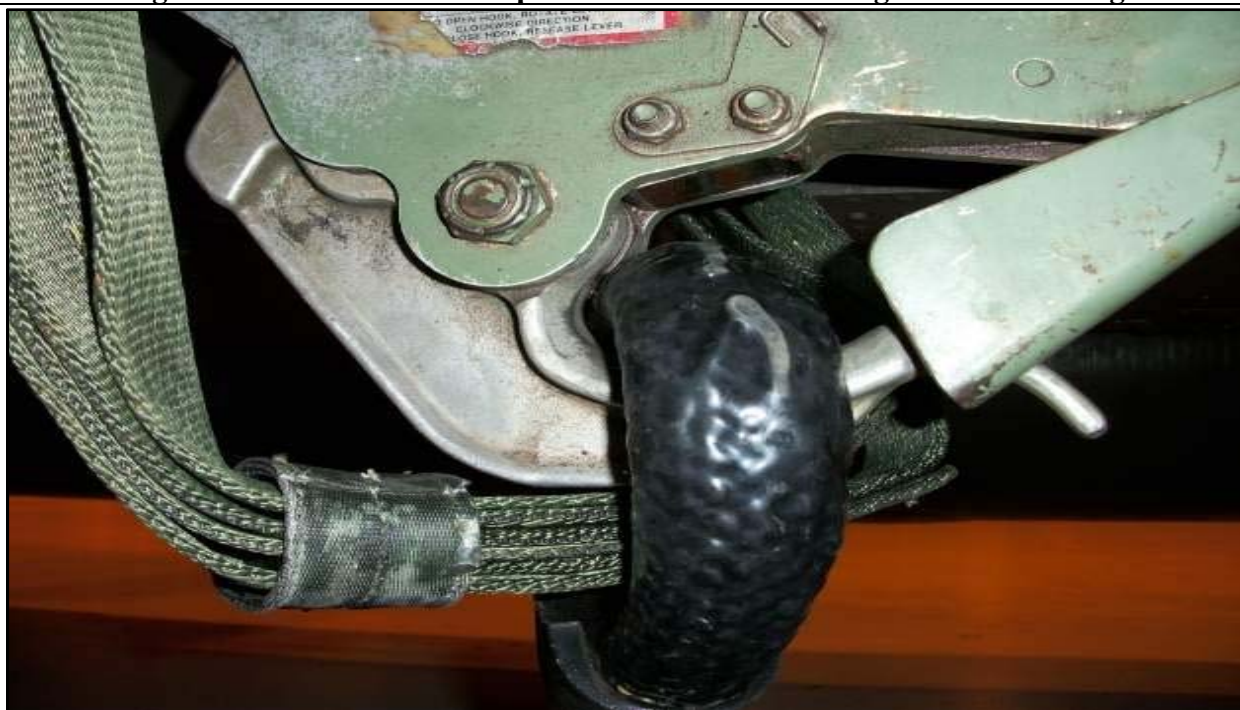
Figure 10-7. H-60 SPIES Rope Connected to H-60 Cargo Hook and Sling (close up view).
