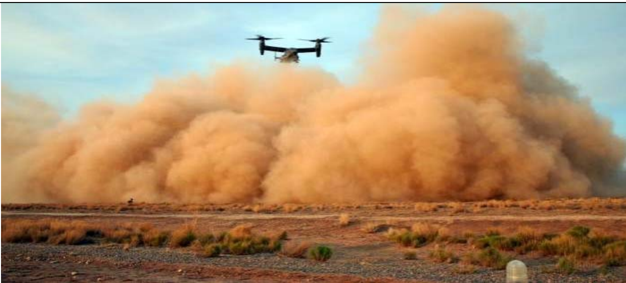
Figure 9-17. Rotor Downwash Characteristics of the V-22.
