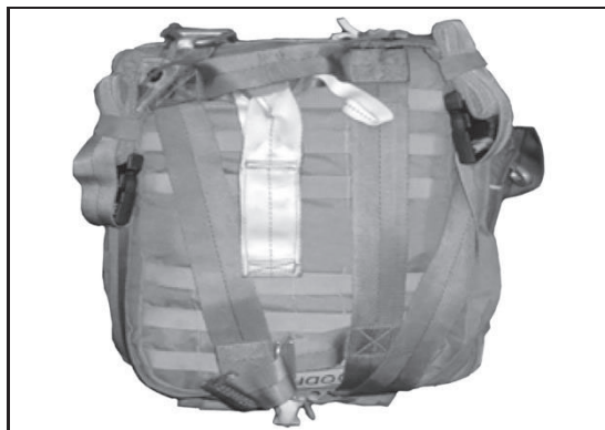
Figure 12-41. Routing of compression straps over release handle cross strap
