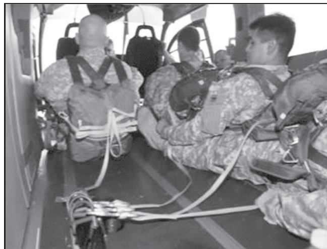
Figure 17-37. Seating configuration for static line personnel without combat equipment and crew chief
