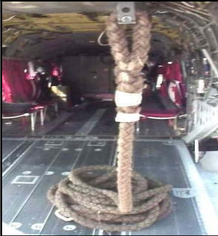
Figure 9-11. Fast Rope Attached to H-47 AFT FRIES Bar.
