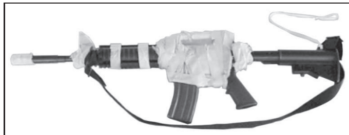
Figure 12-53. Padding, taping the M16 rifle or M4 carbine configured for jumping exposed
