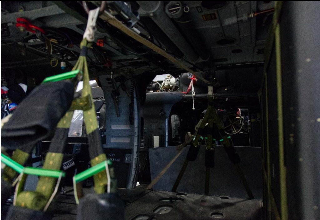
Figure 12-23. Close up of Final Assembly of Crow's Foot Tensioning Assembly Showing Routing of Cut Strap. (Rear Angle)
