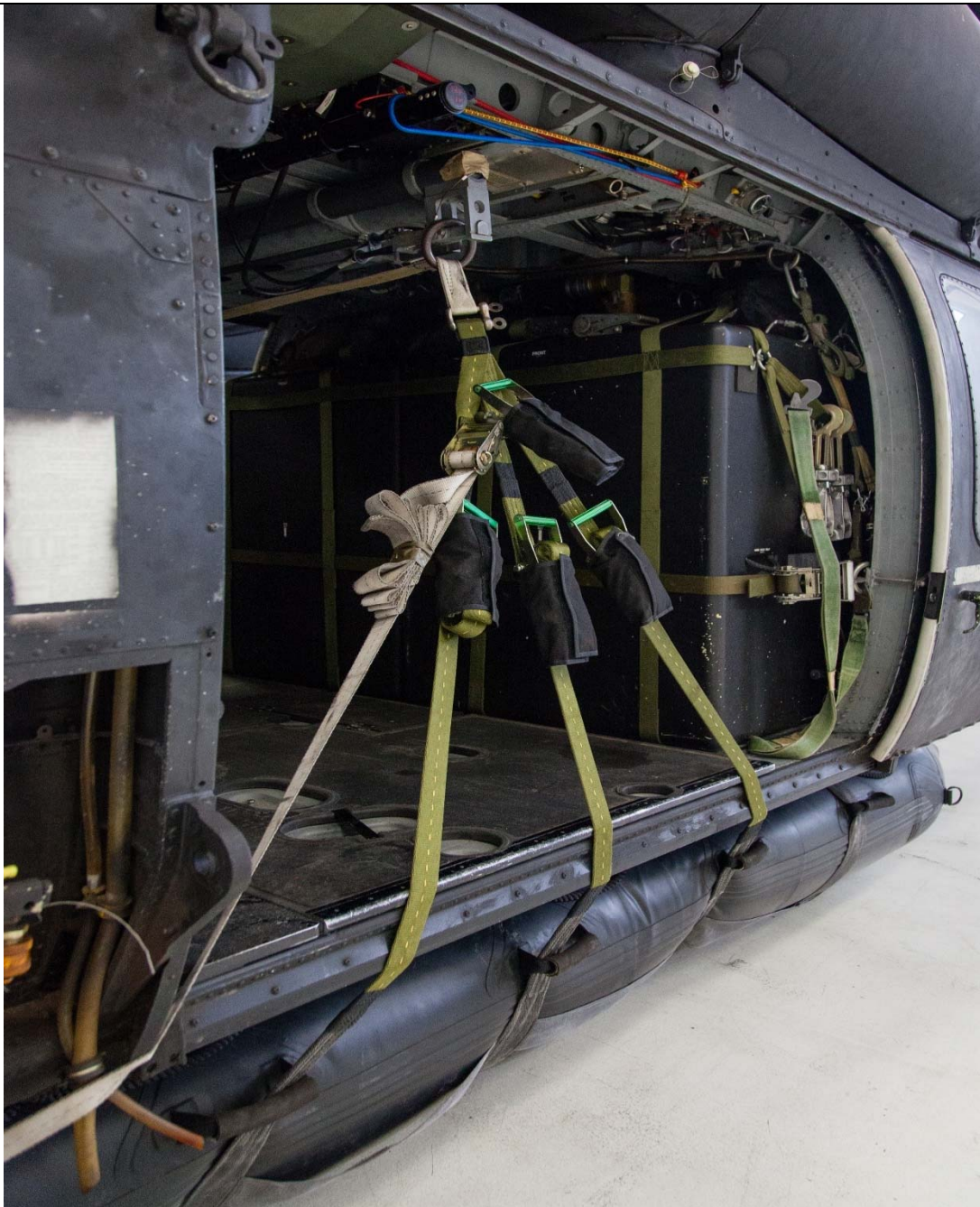
Figure 12-34. Final Installation of Crow's Foot Tensioning Assembly Showing Cradle Leg Routing.
