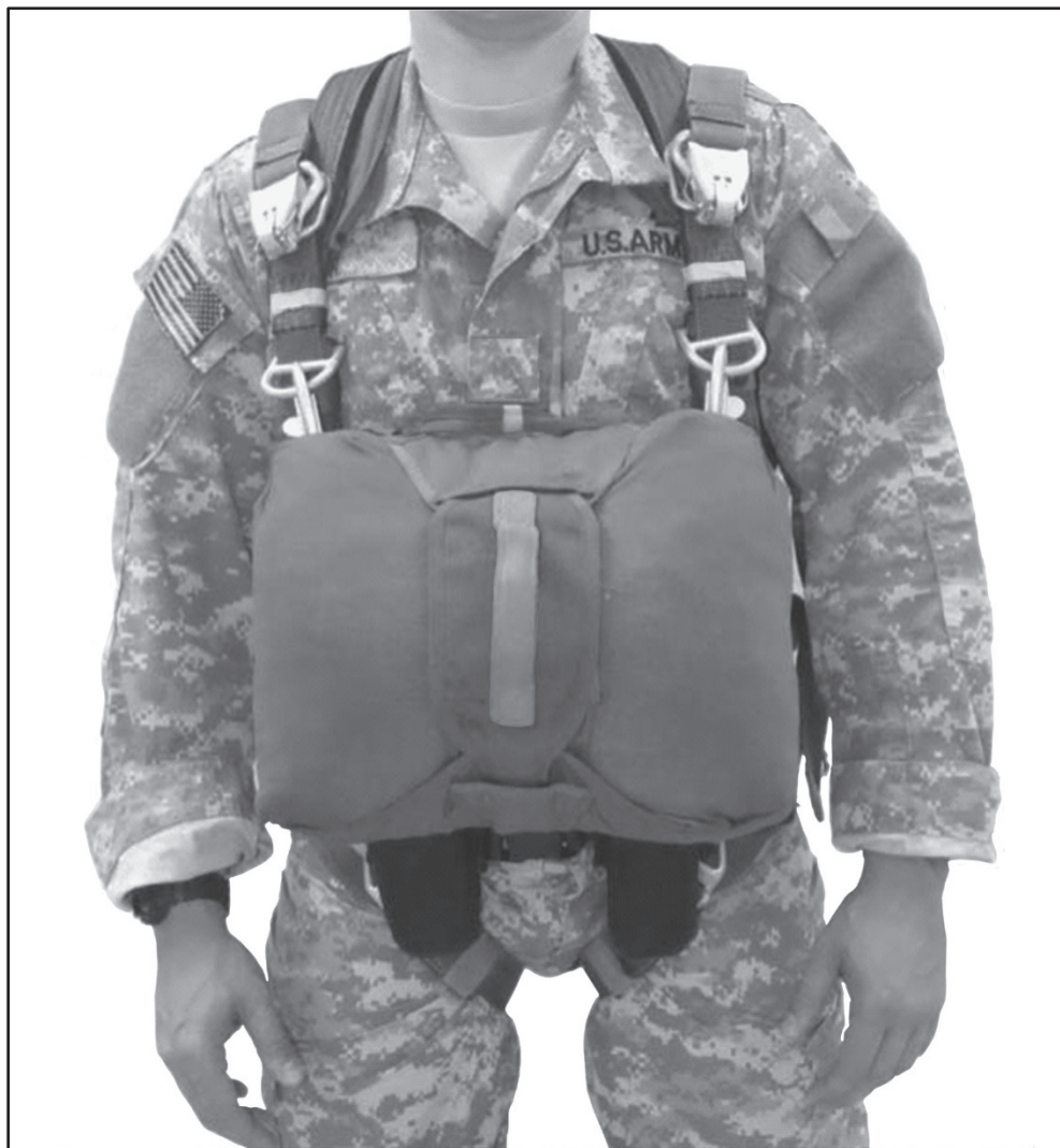
Figure 12-63. TFSS 5326 fastened to a Soldier's waist belt
