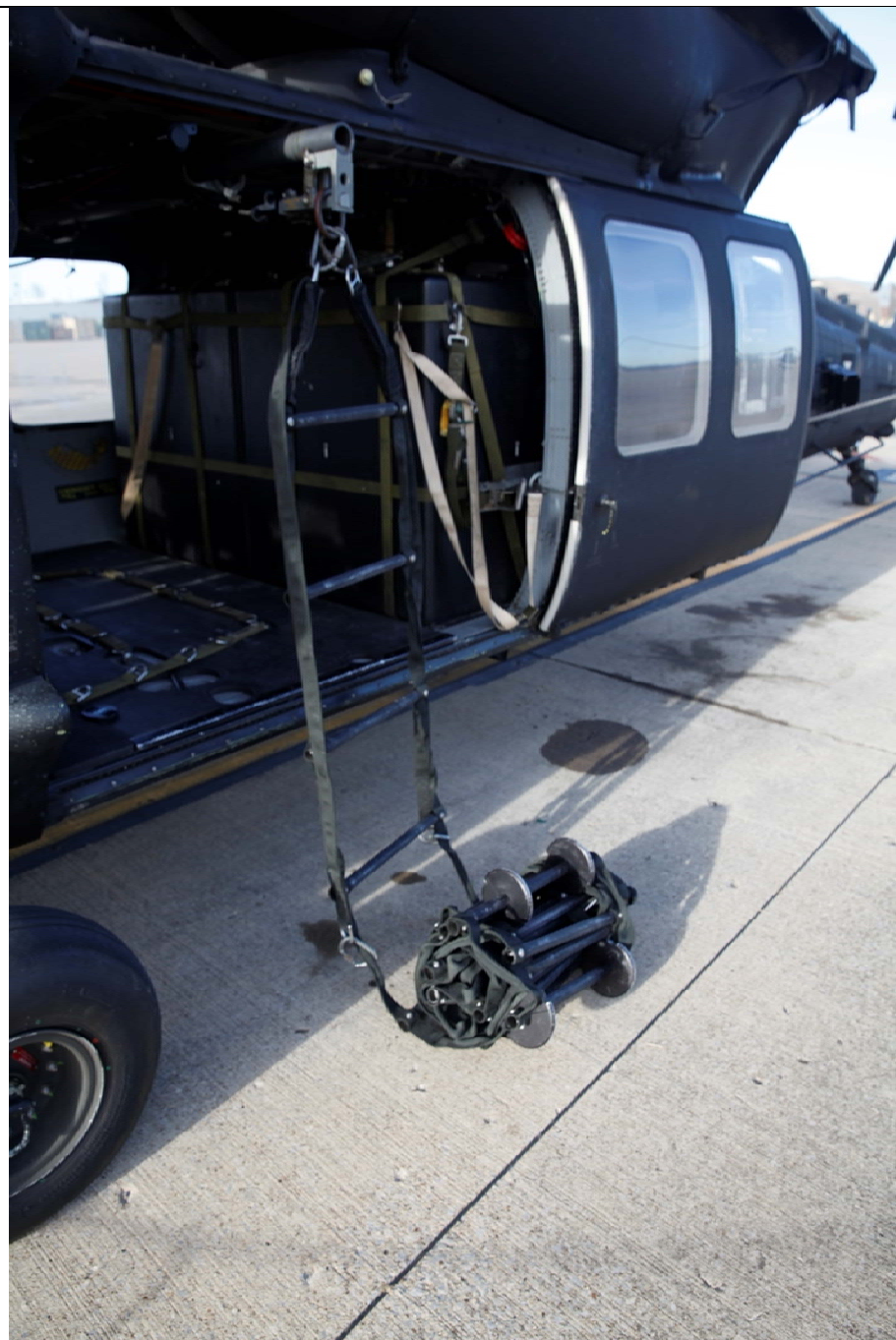
Figure 11-9. Nylon Ladder attached to FRIES Bar.
