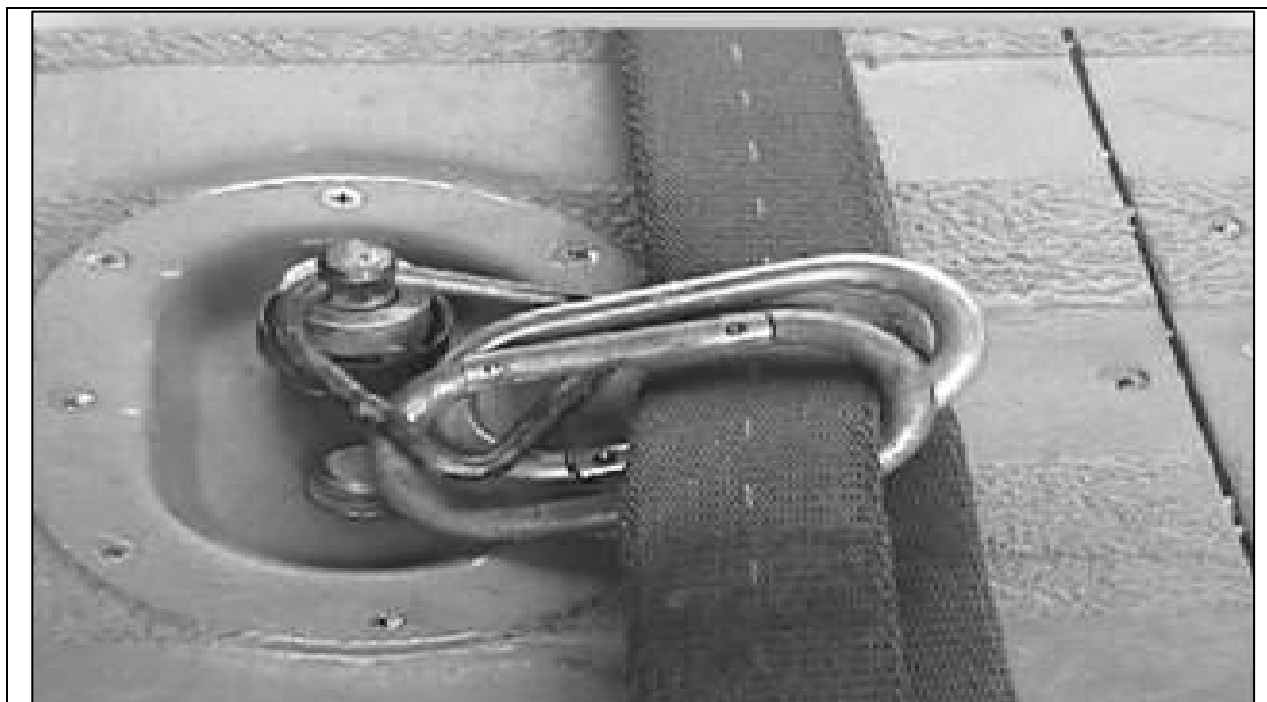
Figure 10-11. H-60 Snap Links Connected to Sling and Ring, Gates Reversed.
