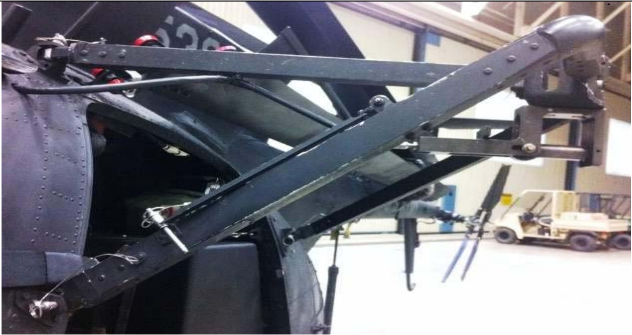
Figure 9-37. Mount for External Fast Rope System on MH-6.
