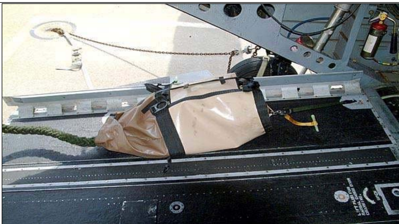
Figure 9-24. Small Fast Rope Bag Positioned on the Ramp.
