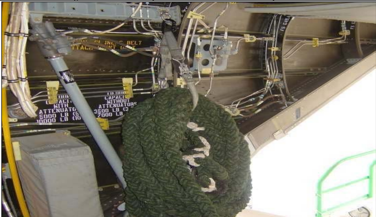
Figure 9-15. Fast Rope Secured on V-22 (STA 602).
