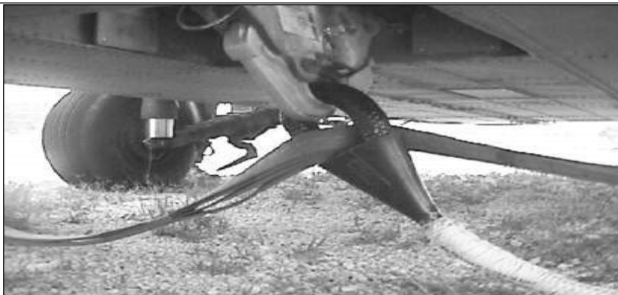
Figure 10-6. H-60 SPIES Rope Connected to H-60 Cargo Hook and Sling.
