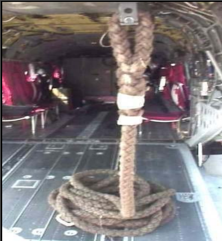
Figure 9-42. Fast Rope Attached to H-47 Aft FRIES Bar.
