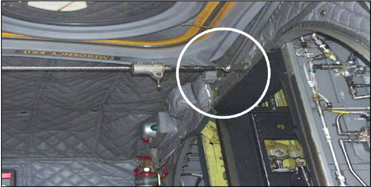
Figure 13-14. Forward anchor line cable (attachment)
