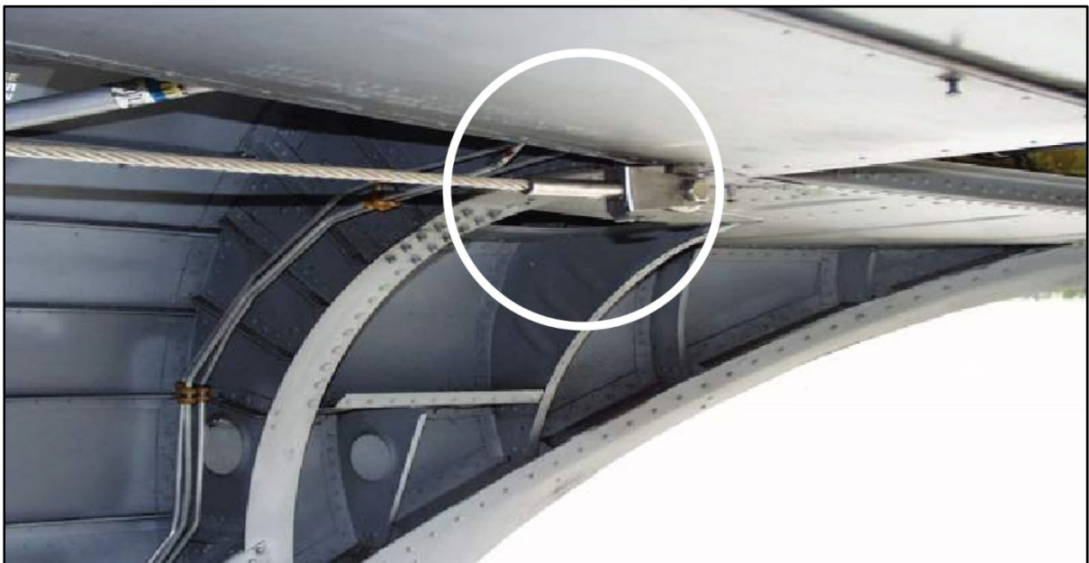
Figure 13-15. Rear anchor line cable (attachment)
