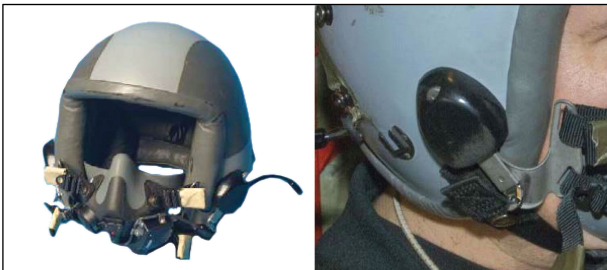
Figure 12-5. Parachutist oxygen mask with bayonet connectors and taped straps
