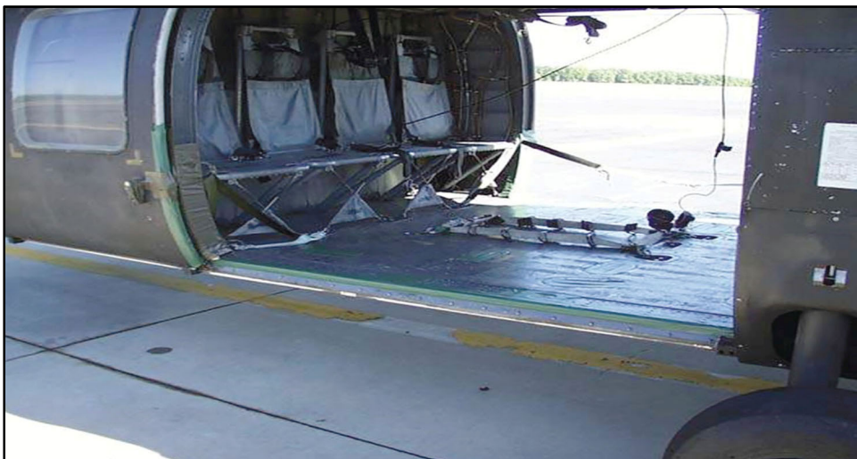
Figure 13-3. UH-60A compartment prepared for jumping
