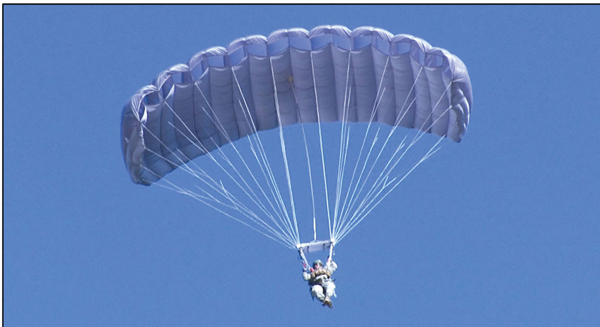
Figure 1-3. Double-bag static line configuration (canopy deployed)
