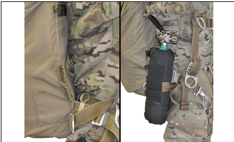
Figure 12-11. A composite 3,000 psi bottle and pouch attached to jumper
