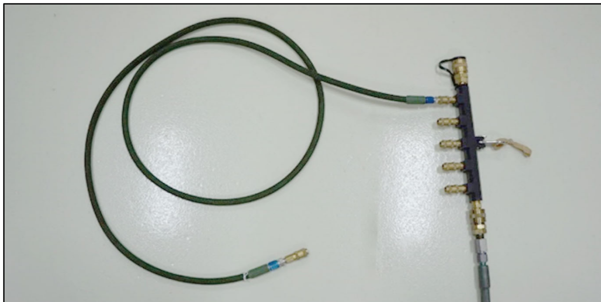
Figure 12-17. Main oxygen supply hose from console with five port adaptor and jumper oxygen supply hose
