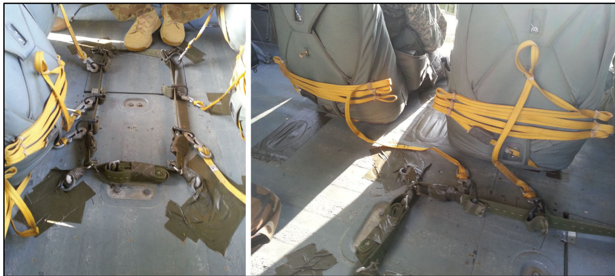
Figure 13-8. Proper universal static line snap hook and static line routing
