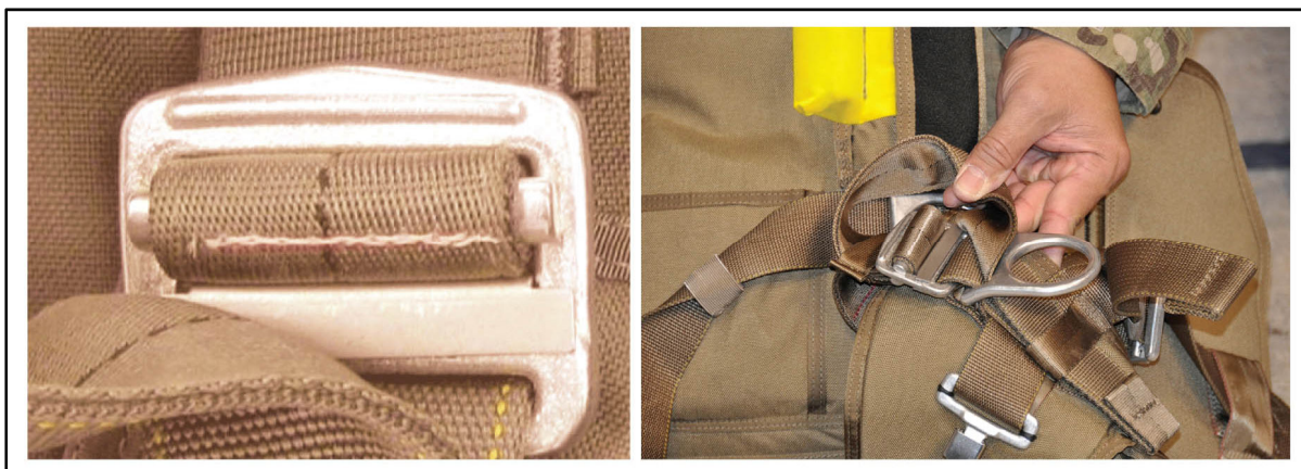
Figure 4-4. Main lift web thread stitching location
