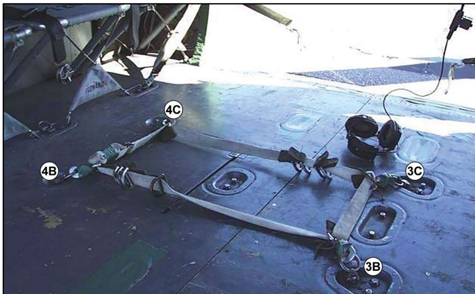
Figure 13-5. UH-60A modified anchor line secured to floor
