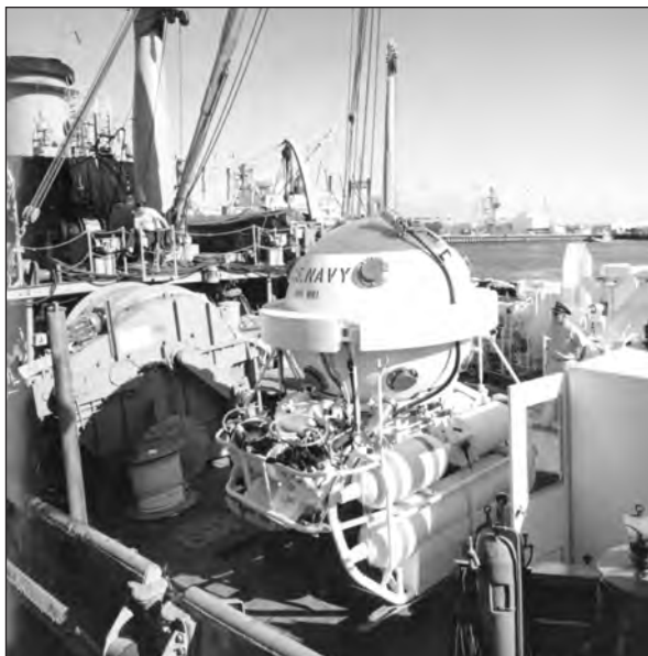
Figure 1-19. DDS MK 1 Personnel Transfer Capsule.
