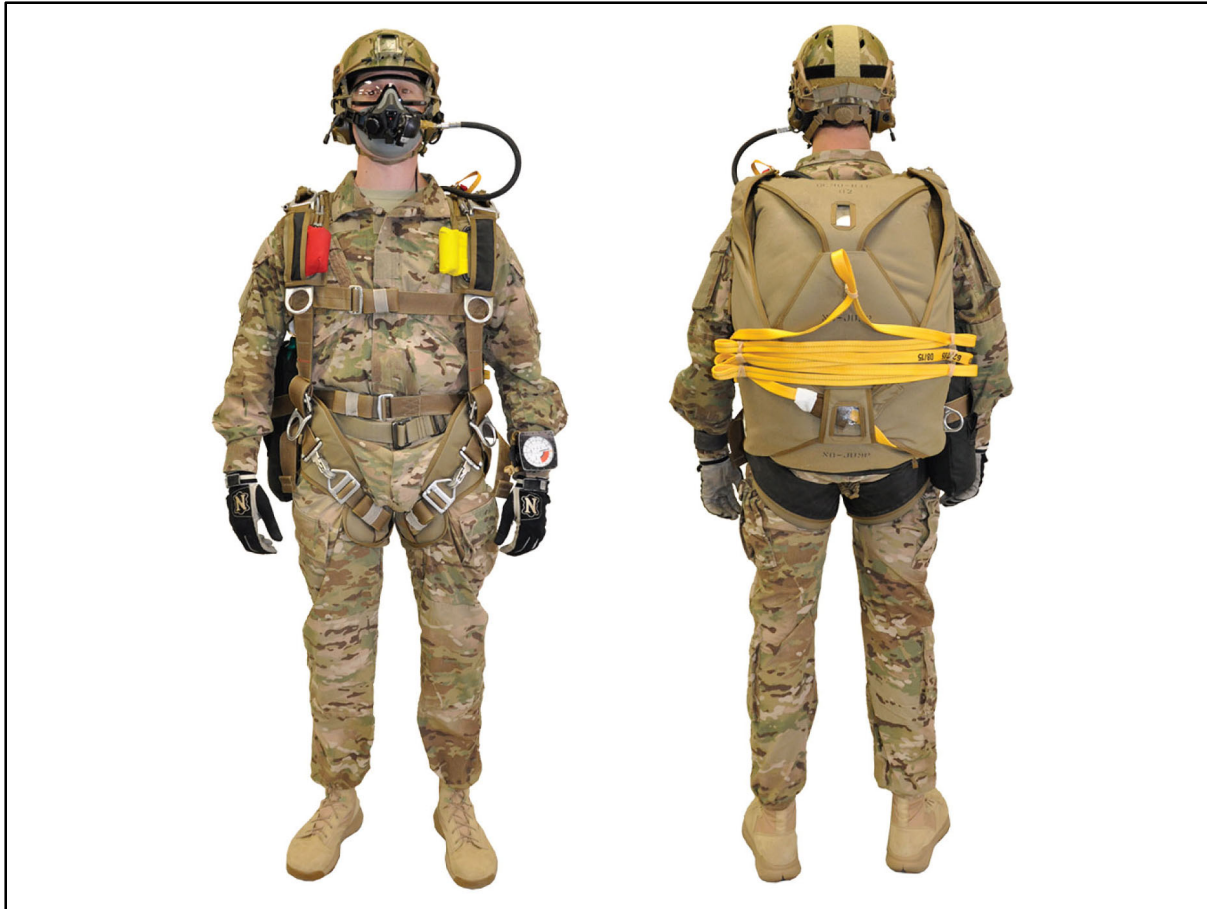
Figure 1-2. Double-bag static line configuration (rigged)
