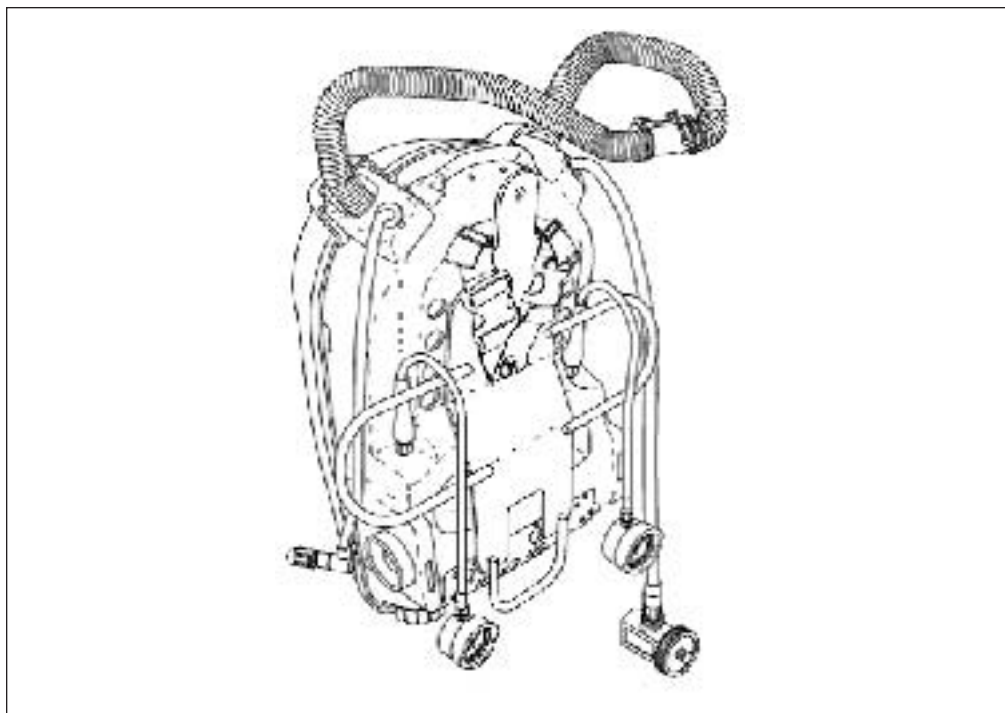
Figure 15-5. Typical EC-UBA Emergency Breathing System.
