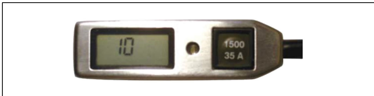
Figure 10-9. Beginning of Military CYPRES 2 self-test countdown in absolute (operational) mode
