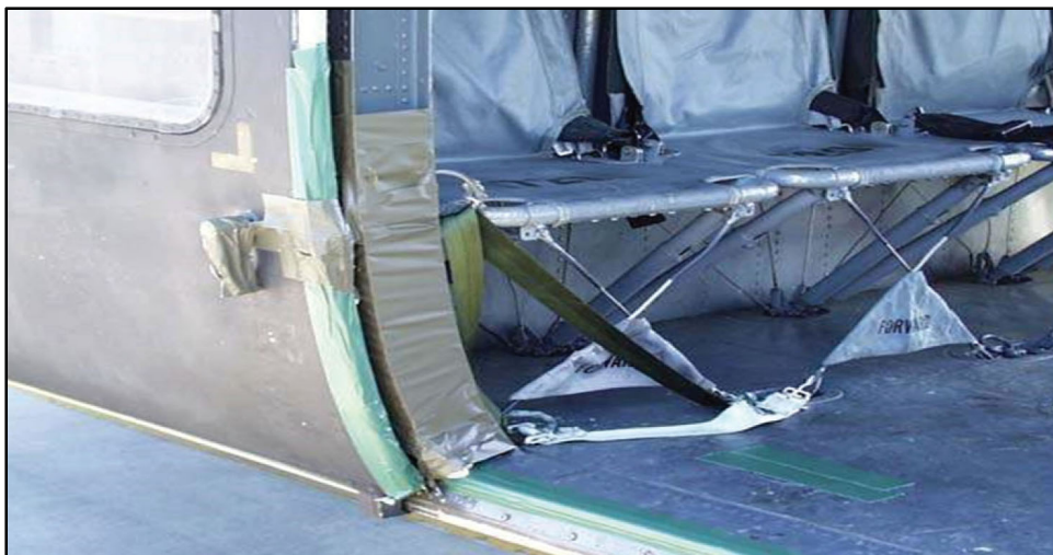
Figure 13-4. UH-60A door edge padded and taped
