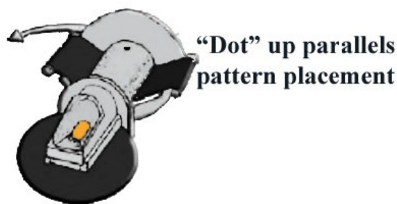
Figure 3-11. Place the pattern in a vertical position.
