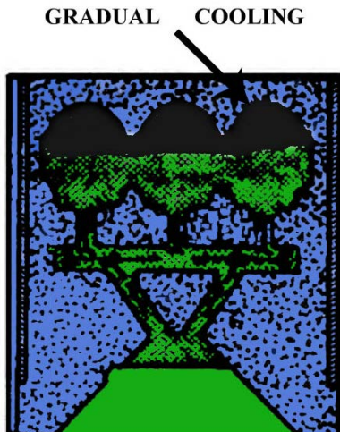
Figure 3-6. Investment heat prevents rapid cooling of the casting.
