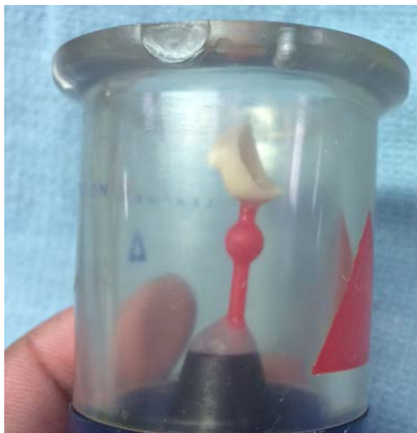
Figure 3-8. Sprue directly to the incisal edge.
