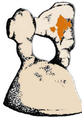
Figure 2-53. Hole in casting caused by a thin spot in the pattern.
