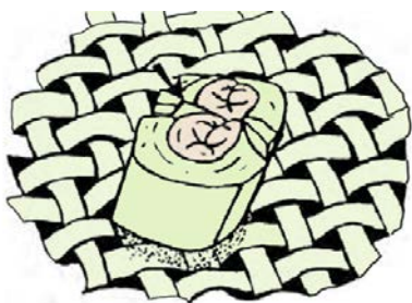
Figure 3-29. Solder patty on soldering frame.
