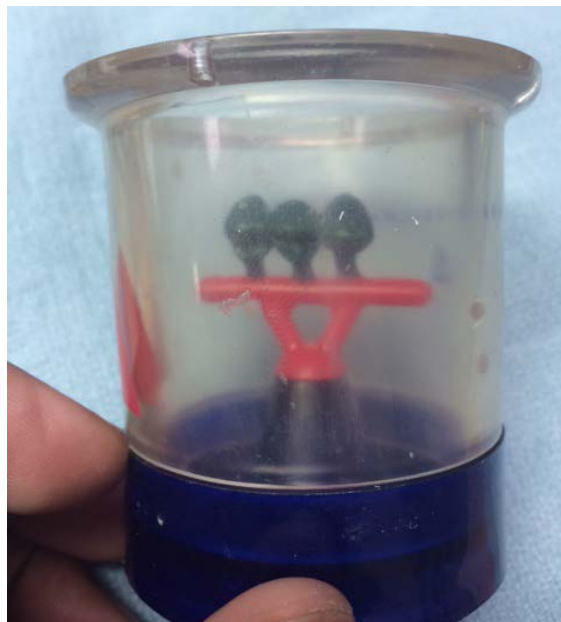
Figure 3-4. Example of indirect spruing.
