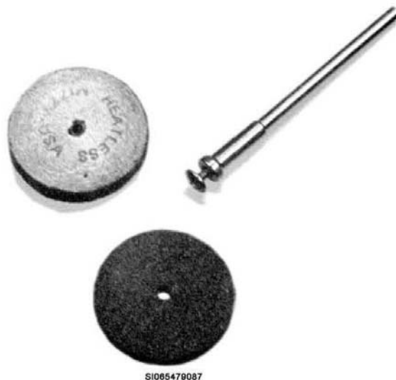
Figure 2-31. Abrasive stone wheels with screw on straight mandrel.
