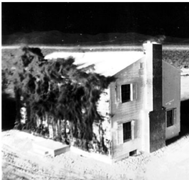
Figure 4-12. The thermal pulse charring the paint.
