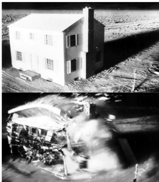
Figure 4-10. The effects of the blast wave on a typical wood framed house.
