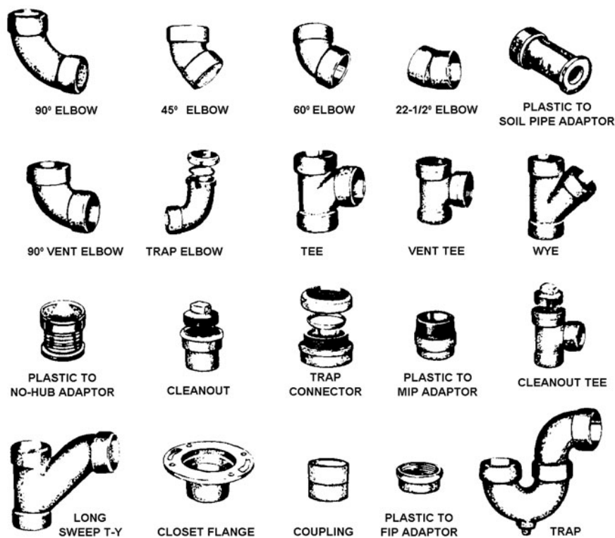
Figure 1-13. Types of plastic fittings.
