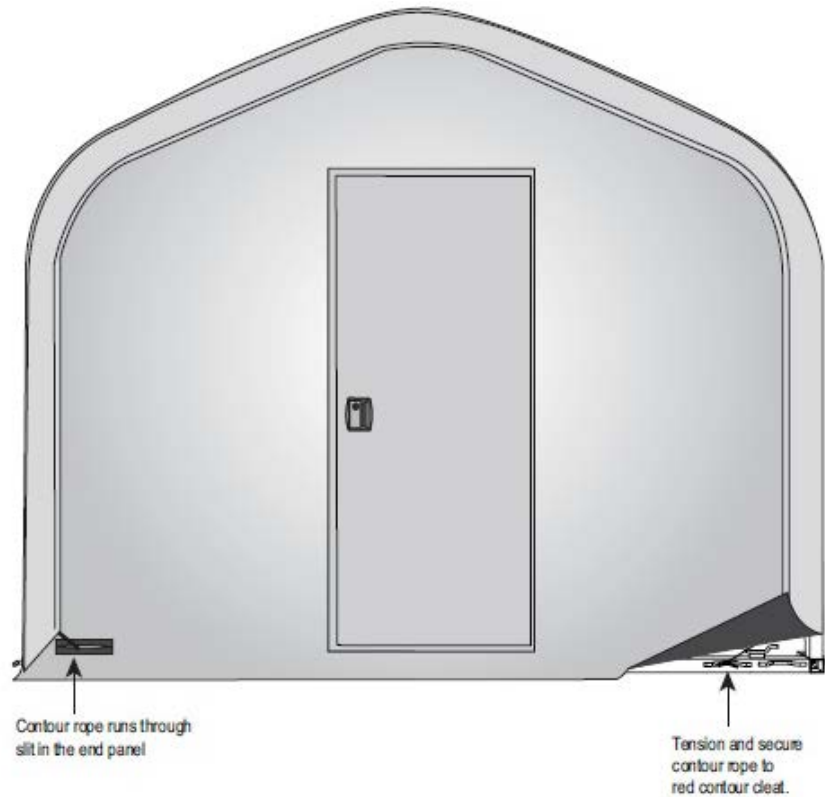
Figure 2-87. Ground flap.
