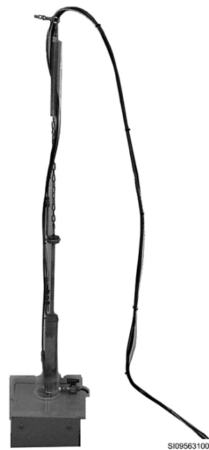
Figure 3-10. Pneumatic probe assembly.
