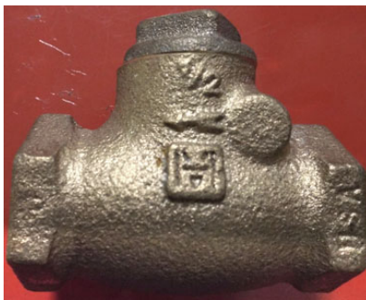
Figure 2-16. Check valve.
