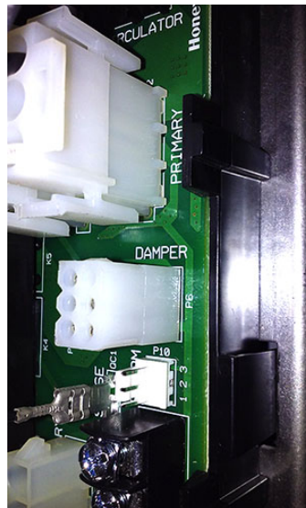
Figure 2-65. Damper connector on circuit board.
