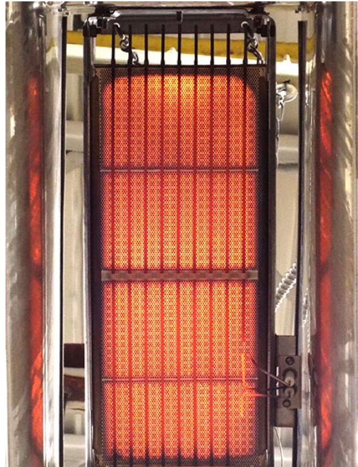
Figure 3-23. Gas lit and distributed evenly over material.
