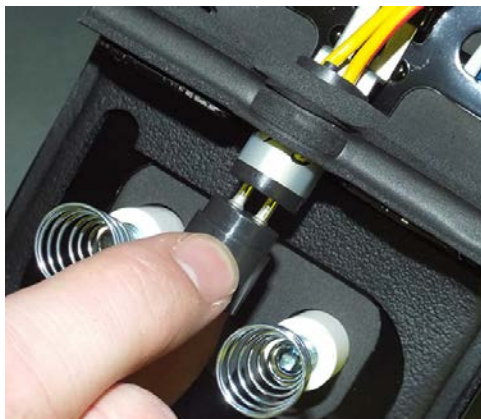
Figure 2-76. Plugging in new cad cell.
