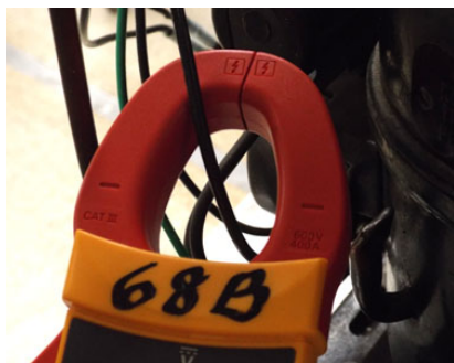
Figure 1-18. Proper way to take ampere reading.
