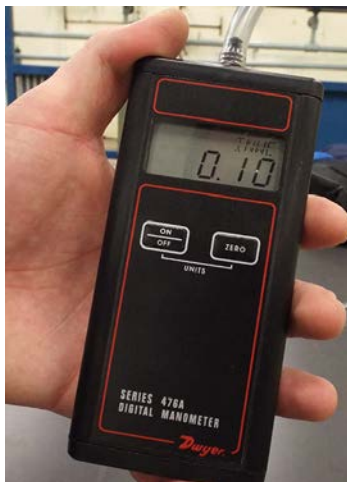
Figure 2-47. Digital manometer.
