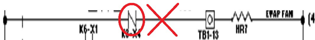
Figure 1-37. ECU series circuit with an open.
