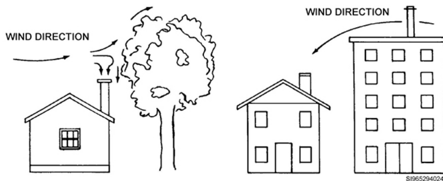
Figure 3-27. Causes of downdraft.
