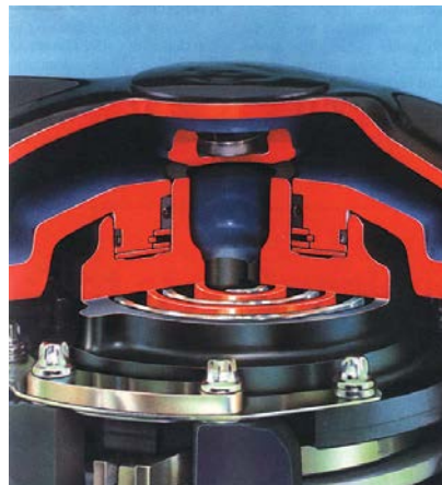
Figure 1-14. Scroll compressor cutaway. (Courtesy Cengage Learning.)
