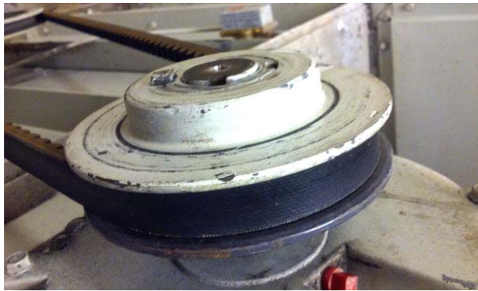
Figure 1-16. Drive sheave or pulley.
