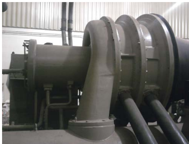
Figure 1-11. Centrifugal compressor.
