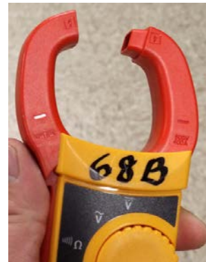
Figure 1-17. Clamp on ammeter.
