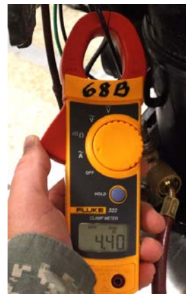
Figure 1-19. Ampere reading.
