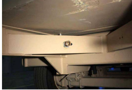
Figure 1-52. Ground stud location.
