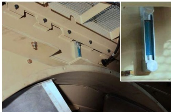
Figure 1-50. Coolant level indicator.
