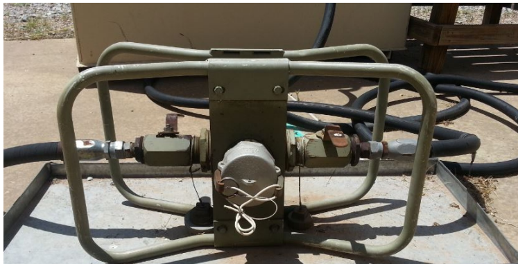
Figure 1-7. Fuel manifold.
