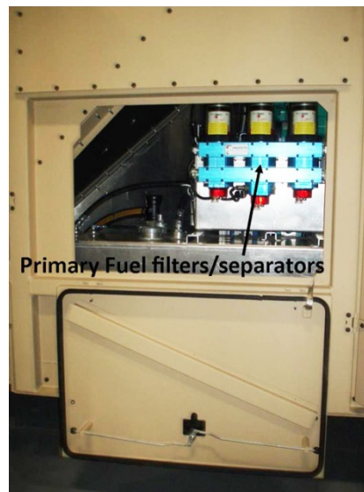
Figure 1-39. Primary fuel filter assembly.
