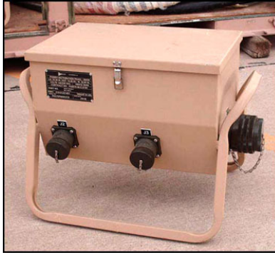
Figure 2-8. PDP.200 Amp.
