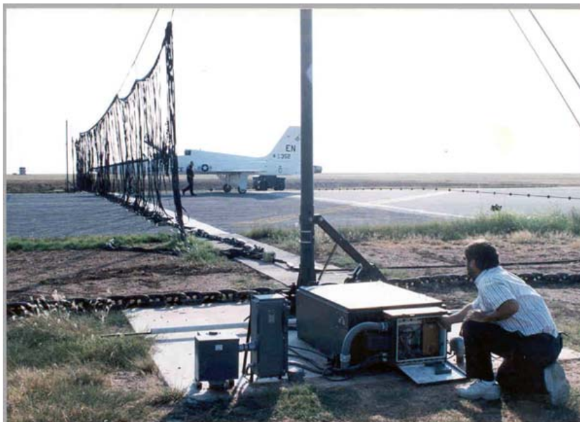
Figure 1-6. BAK-15 aircraft arresting system.
