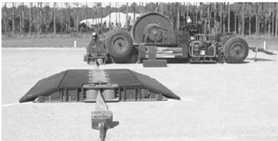
Figure 1-46. Typical MRES installation.
