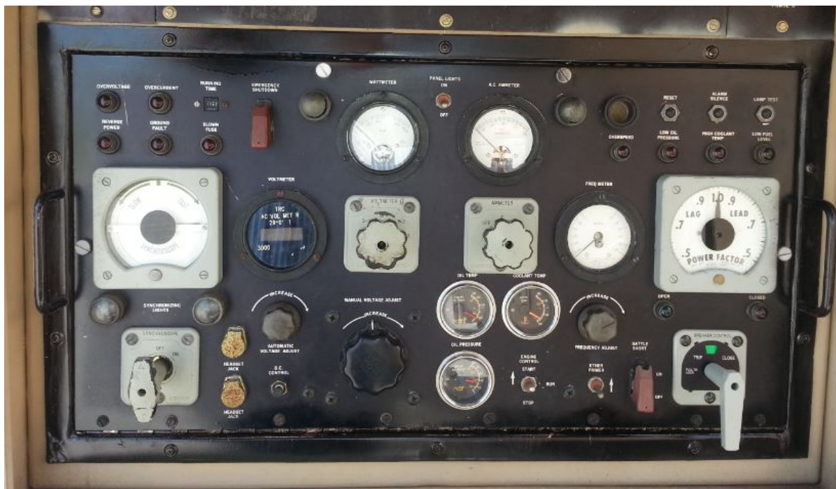
Figure 1-2. MEP-12 control panel.
