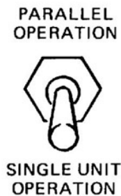
Figure 1-17. Parallel and single unit operation switch.
