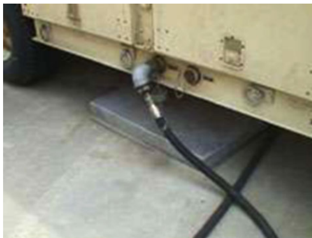
Figure 1-9. MEP-12 fuel connections.
