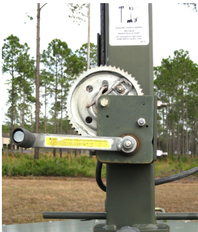
Figure 3-12. Tower Hand Crank.
