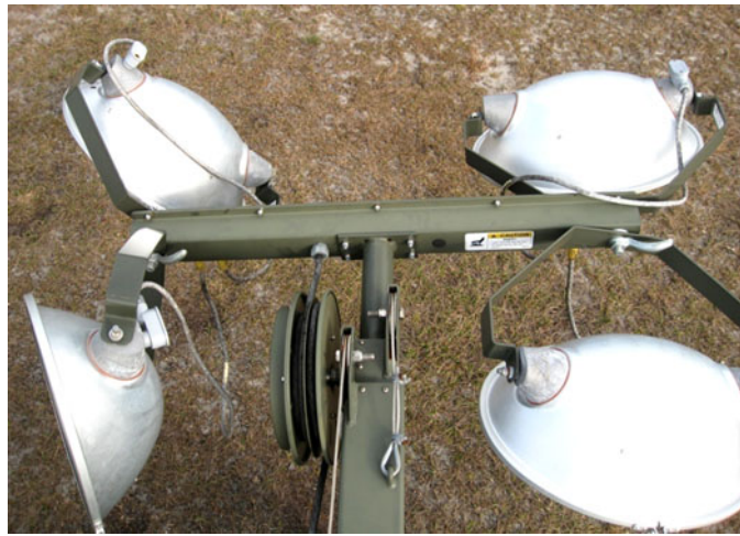
Figure 3-10. Tower floodlight fixtures.
