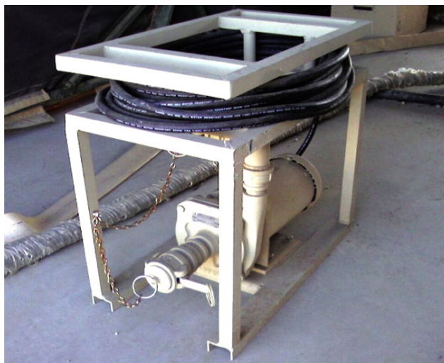
Figure 3-22. ROWPU distribution pump.
