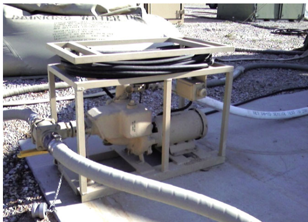
Figure 3-21. ROWPU raw water pump.
