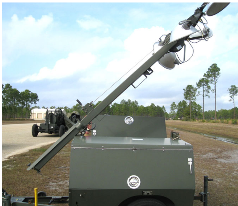
Figure 3-11. Placing tower in upright position.
