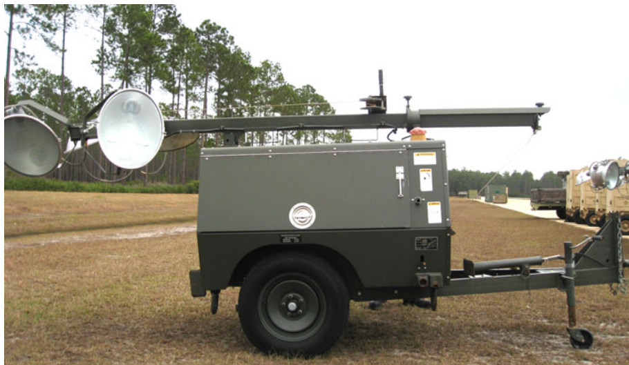
Figure 3-7. Telescoping floodlight set.
