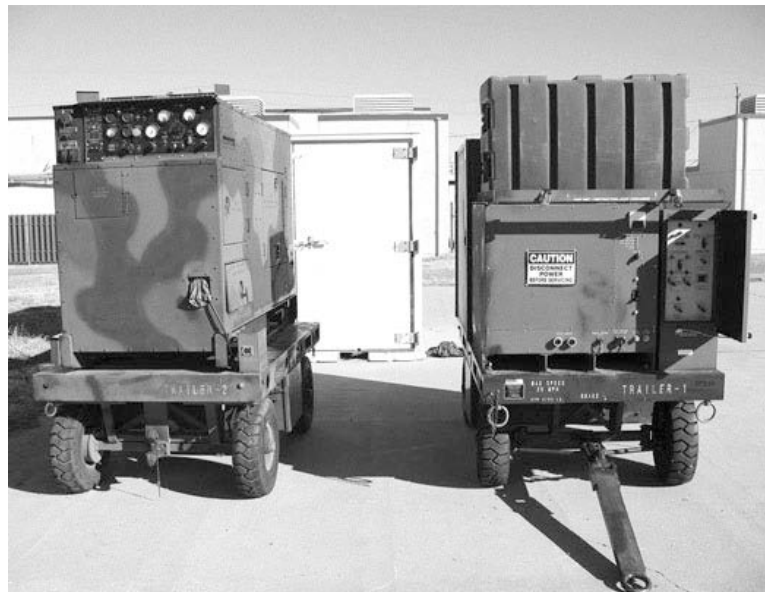
Figure 1-2. EALS regulator and generator.
