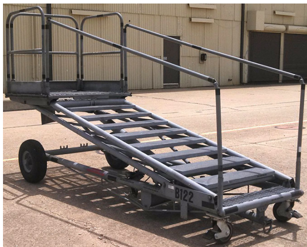
Figure 2-17. B-1 maintenance stand.
