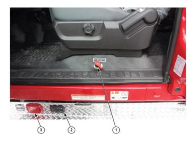
Figure 3–5. Battery switch, battery status indicator, and 110-volt alternating current connection port.
