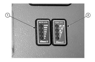
Figure 3–11. Water and foam level indicators.
