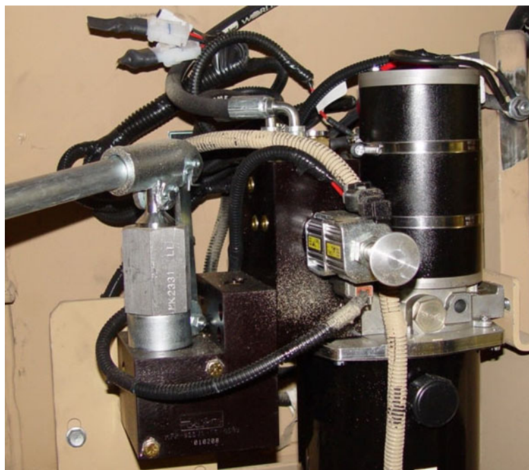
Figure 4-53. Rear-door hydraulic pump assembly.
