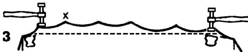
Figure 1-26. Incorrect method for repairing body damage.
