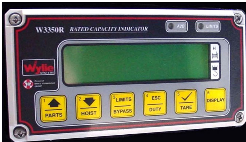
Figure 1-17. Rated capacity indicator and anti-two-block display.
