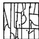
C. Line Cracking
