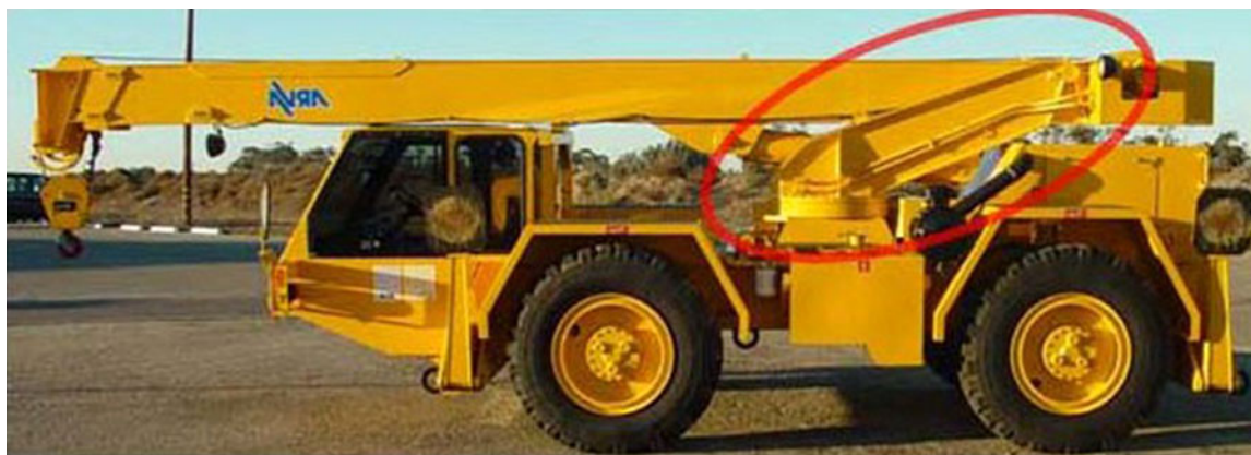
Figure 1-12. Turntable assembly.
