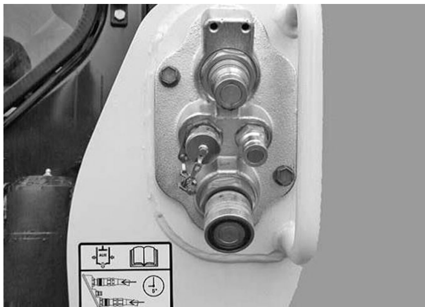
Figure 1-67. Front auxiliary hydraulic coupler block.
