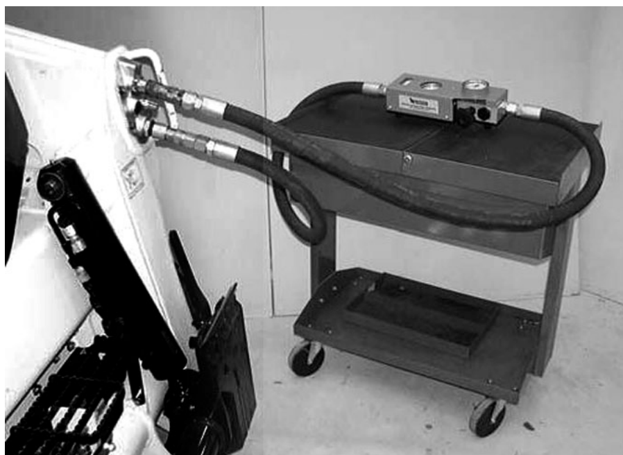
Figure 1-75. Connecting the hydraulic tester to the front auxiliary hydraulic coupler block.
