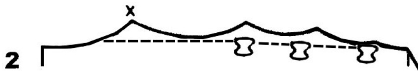
Figure 1-25. Incorrect method for repairing body damage.
