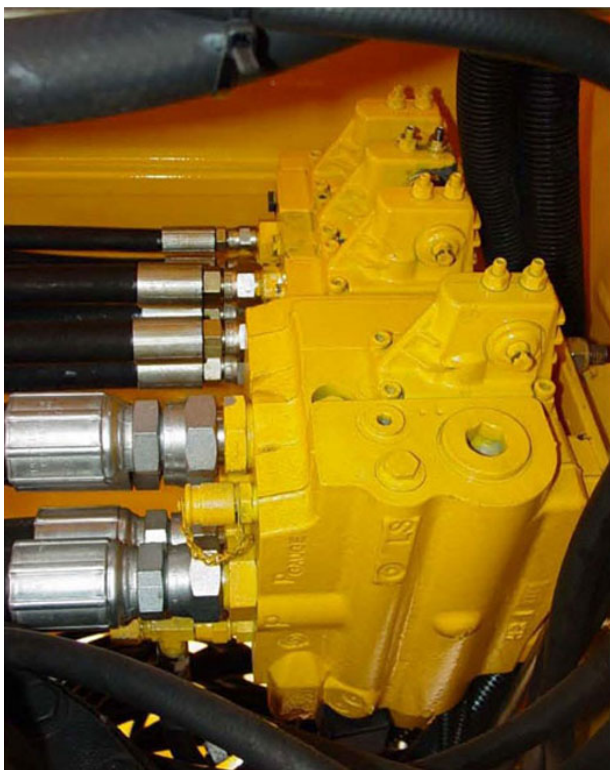
Figure 1-8. Main control valve.
