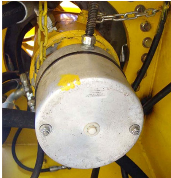
Figure 1-14. Collector ring.
