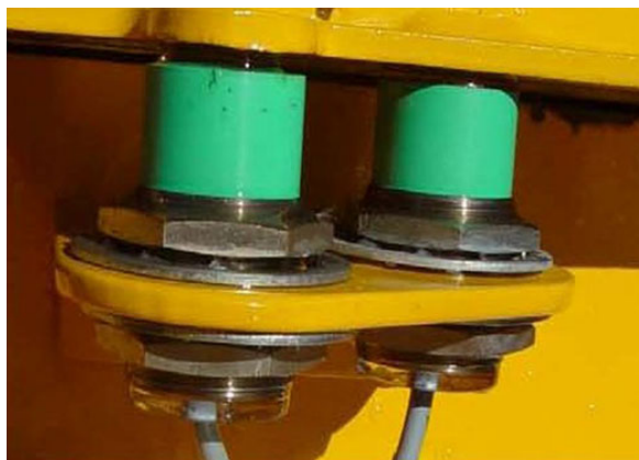
Figure 1-20. Proximity switches.
