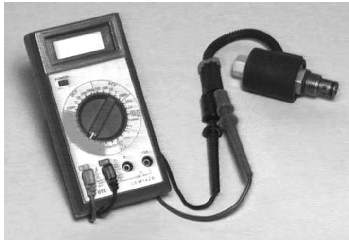
Figure 1-74. Testing resistance across a solenoid coil.
