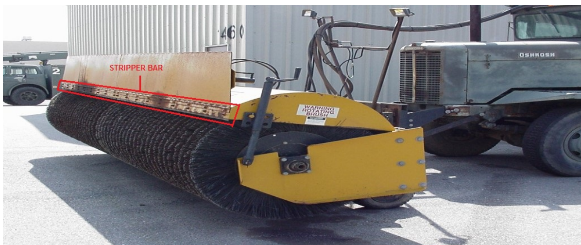
Figure 3-39. Brush stripper adjustment.
