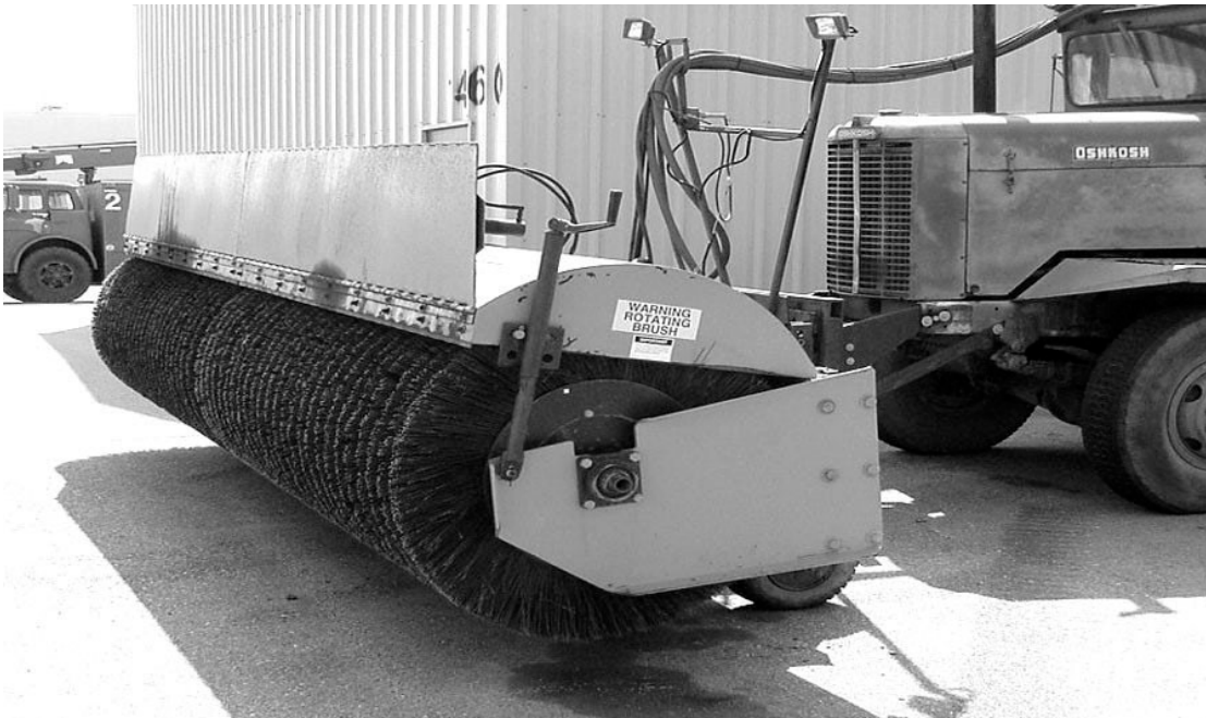
Figure 3-27. Windrow sweeper mounted on truck.
