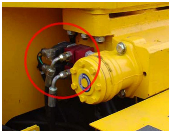
Figure 1-23. Swing cut-out solenoid valves.
