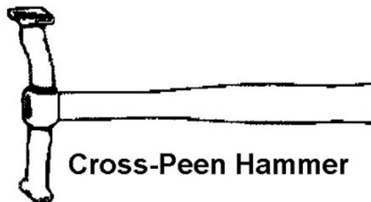
Figure 1-31. Cross-peen hammer.
