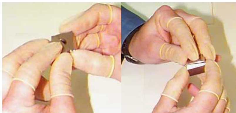
Figure 1.2-11: Wringing Gage Blocks
