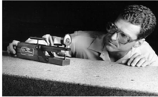
Figure 1.3-2: Repeat Reading Gage
