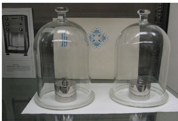
Figure 1.5-1: AFPSL 1 kg Mass Standards
