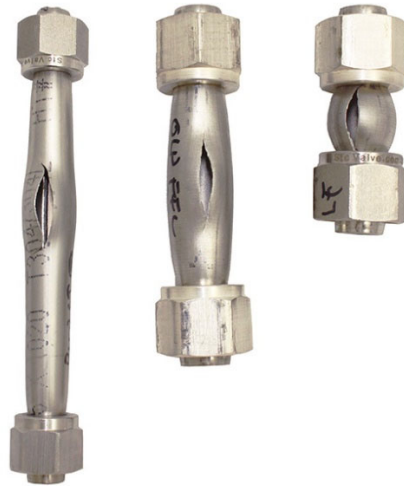
Figure 1.6-10: Tube Failure
