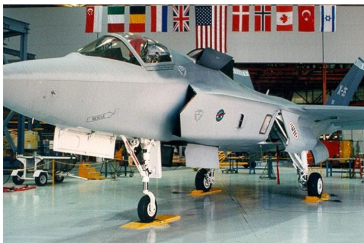
Figure 1.10-6: Aircraft on scales
