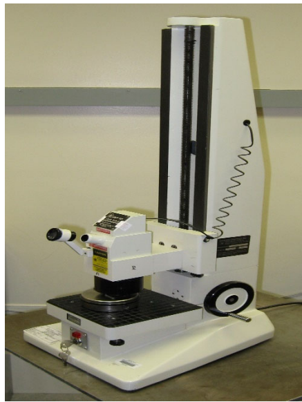
Figure 1.1-3: Gage Block Interferometer
