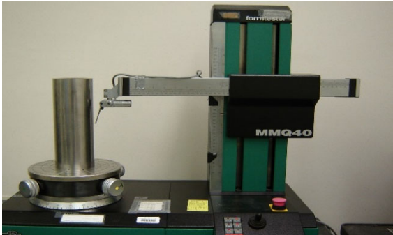
Figure 1.1-18: Roundness Machine measuring roundness of a cylindrical square
