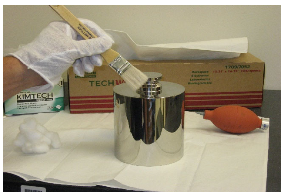
Figure 1.5-5: Cleaning the TI Using a Brush
