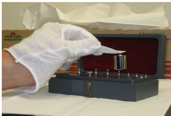
Figure1.5-8: Using forceps to Handle Small Weights
