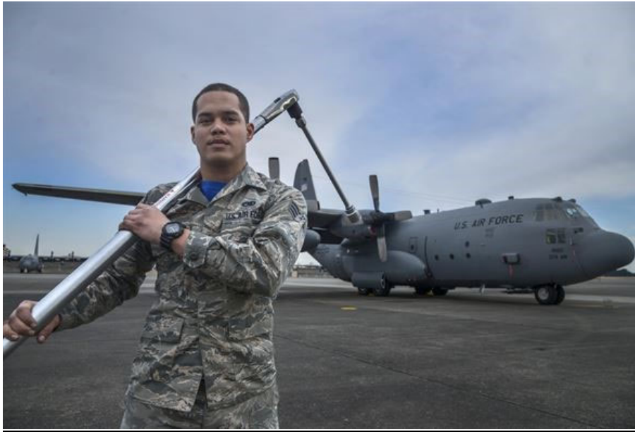
Figure 1.9-1: 2,000 lbf-ft Torque Wrench
