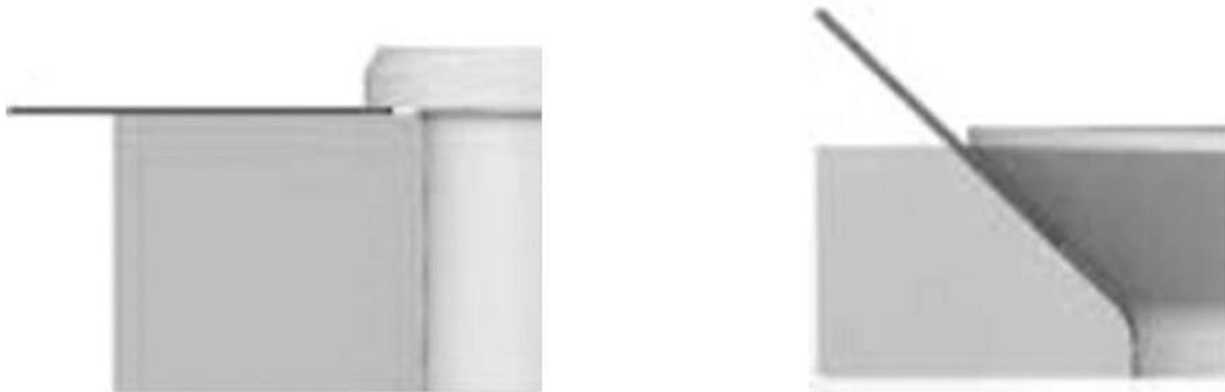
Figure 4-24. .002-inch feeler gage. (Reproduced by permission of Alcoa Global Fasteners, Inc.)
