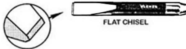
Figure 1-21. Flat chisel.
