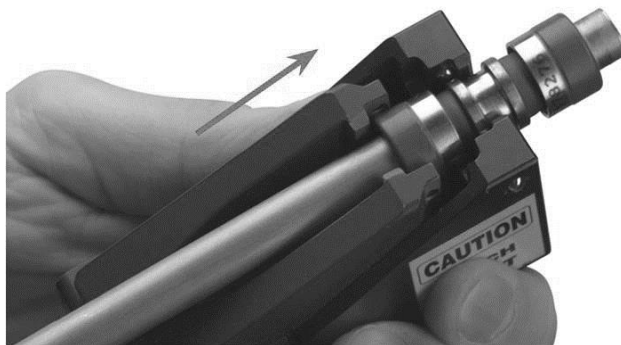
Figure 5-16. Tool position (tube position during pressurization).
