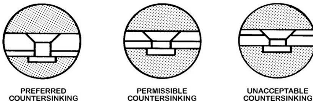
Figure 1-41. Countersinking standards.
