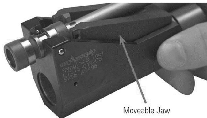
Figure 5-15. Tool position (tube position before pressurization).
