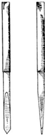
Figure 1-14. Spade (flat) bit for drilling graphite.
