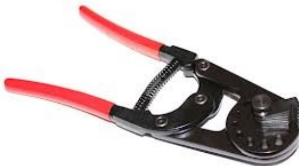
Figure 1-46. Rivet cutter.
