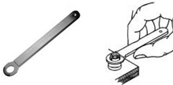
Figure 4-25. Paddle gage. (Reproduced by permission of Alcoa Global Fasteners, Inc.)
