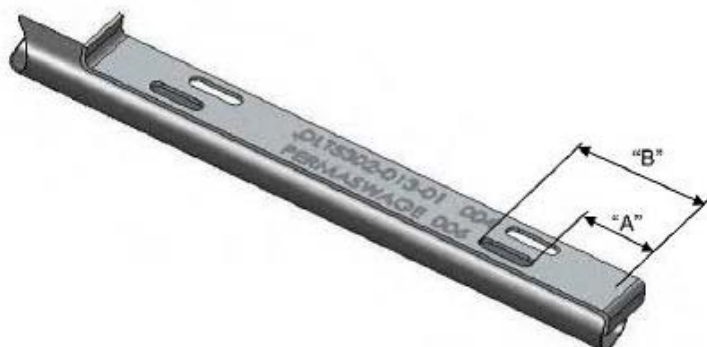
Figure 5-9. Marking with Permaswage marking tool.
