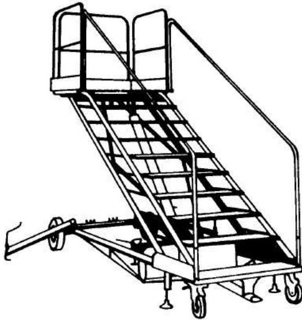
Figure 2-28. B-1 maintenance stand.
