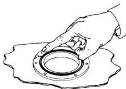
Figure 6-7. Removal of excess petrolatum.
