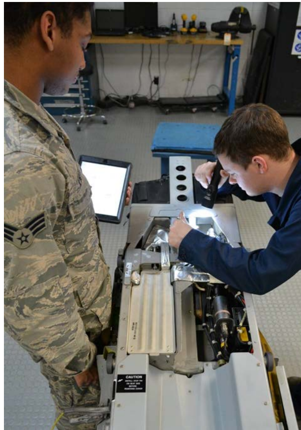
Figure 3-2. Airman performing a visual inspection on the ejection seat.
