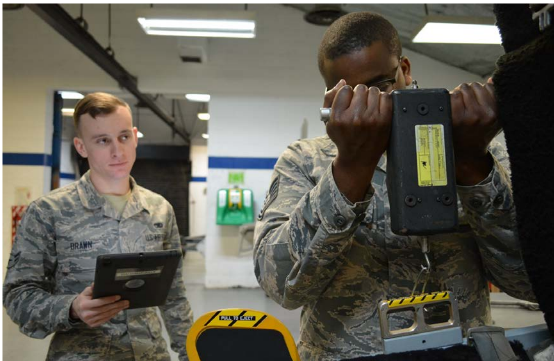
Figure 3-15. Emergency manual parachute deployment handle test.
