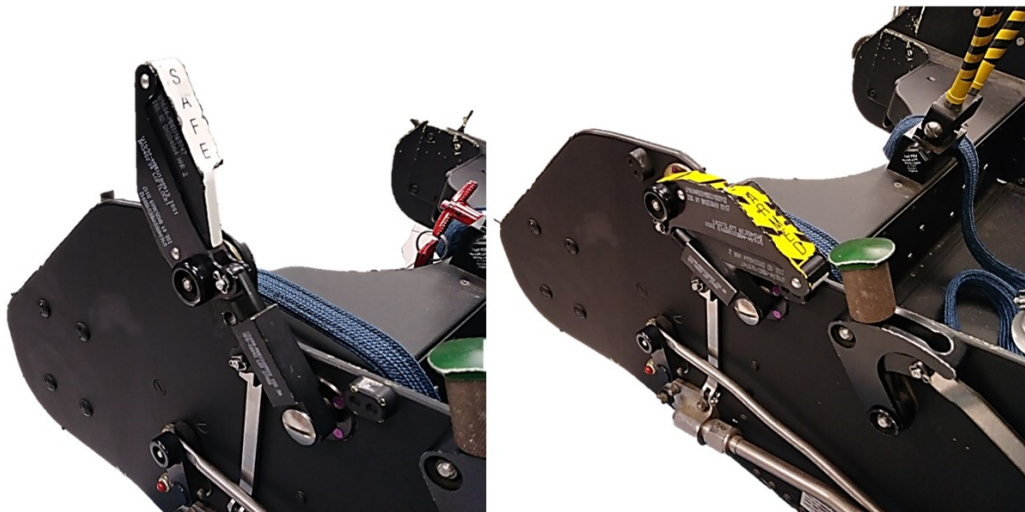
Figure 3-24. Safe/armed lever.
