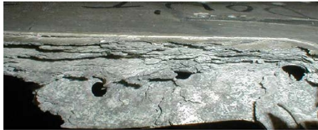
Figure 1-20. Exfoliation corrosion.
