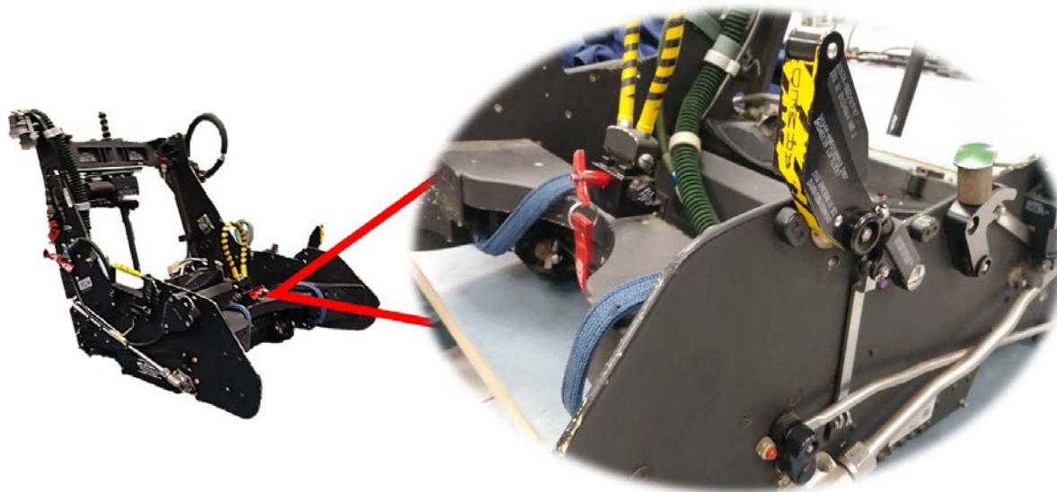
Figure 3-22. Seat bucket and firing handle.
