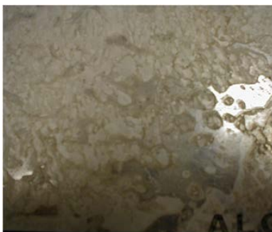
Figure 1-17. Uniform etch corrosion.
