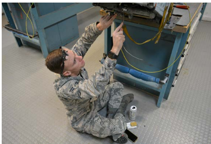
Figure 1-7. Example of what NOT to do when performing a safety wire task.
