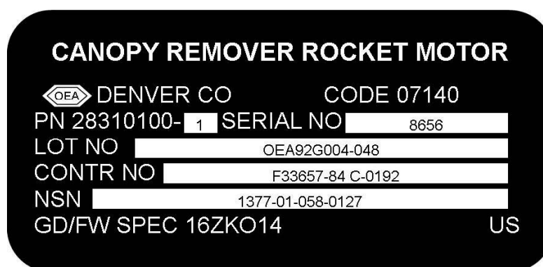
Figure 2-2. Canopy remover rocket motor data plate.
