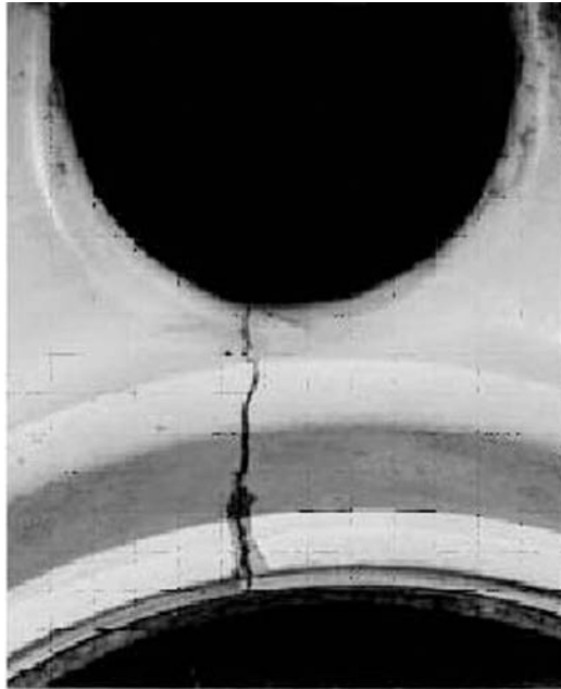
Figure 1-22. Stress corrosion.
