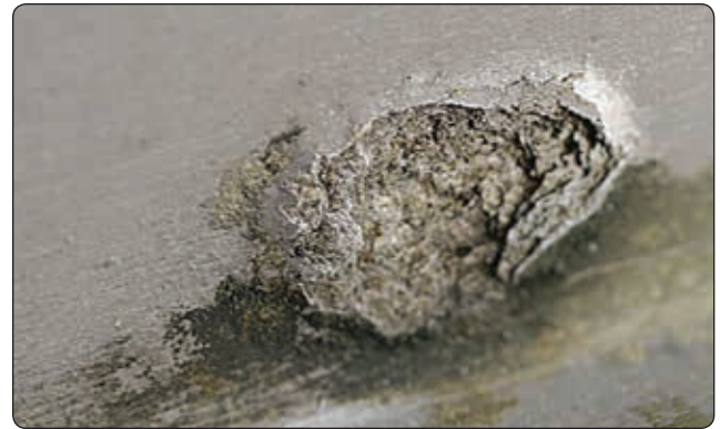
Figure 8-15. Exfoliation corrosion.
