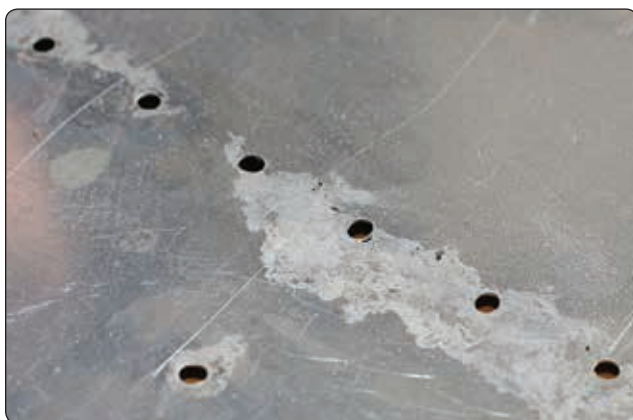
Figure 8-7. Surface corrosion.
