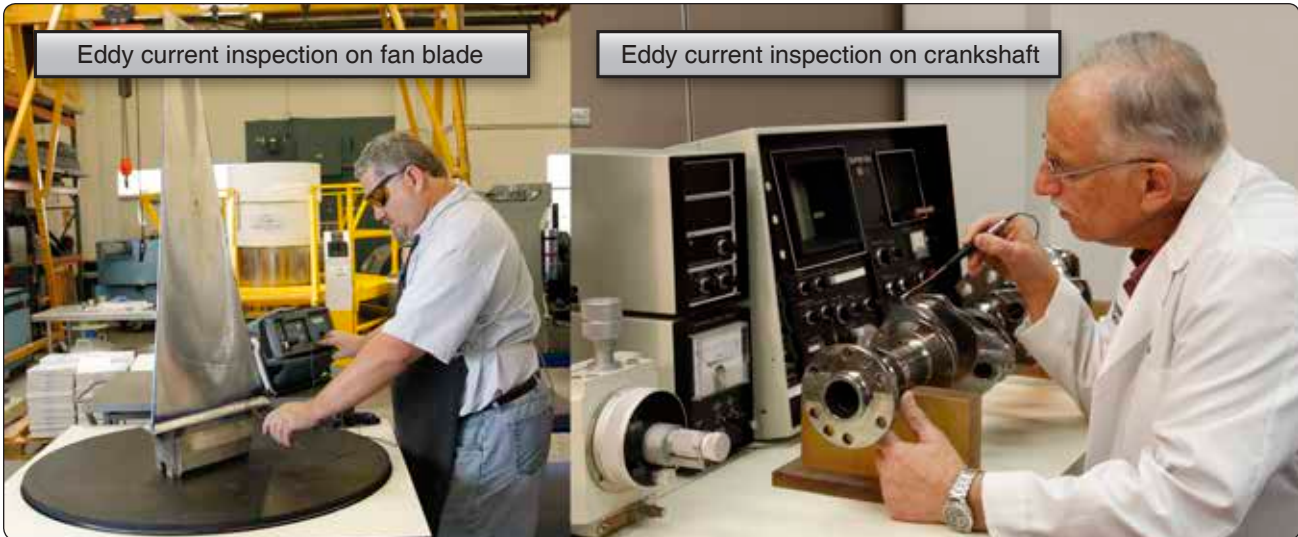
Figure 10-10. Eddy current inspection.
