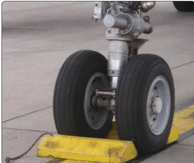
Figure 1-12. Wheels chocked fore and aft.
