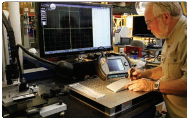
Figure 10-13. Impedance plane test.
