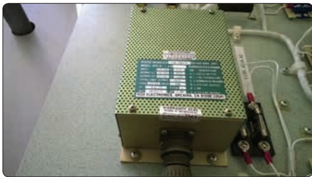
Figure 12-206. Static inverter.
