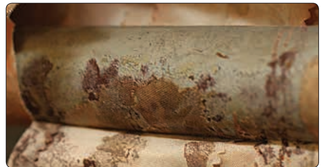
Figure 8-27. Rust on structural components.
