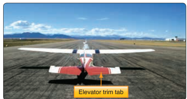
Figure 5-71. Elevator trim tab on a Cessna 182.
