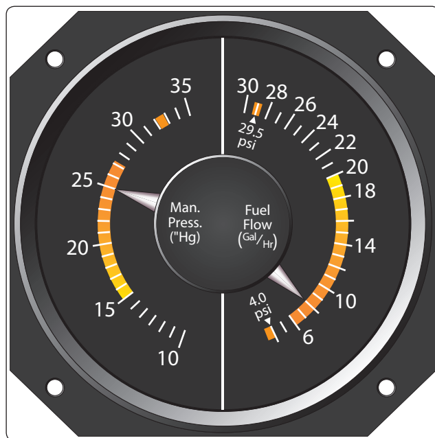
Figure 5-35. Manifold pressure gauge indicating absolute pressure.
