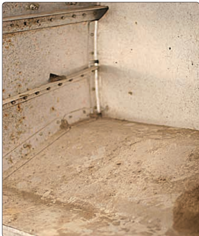
Figure 8-4. Direct chemical attack in a battery compartment.
