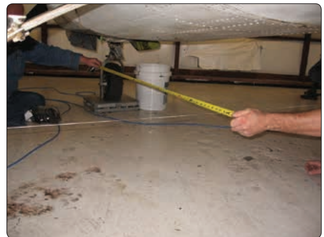
Figure 6-23. Measuring the nosewheel arm on an airplane.
