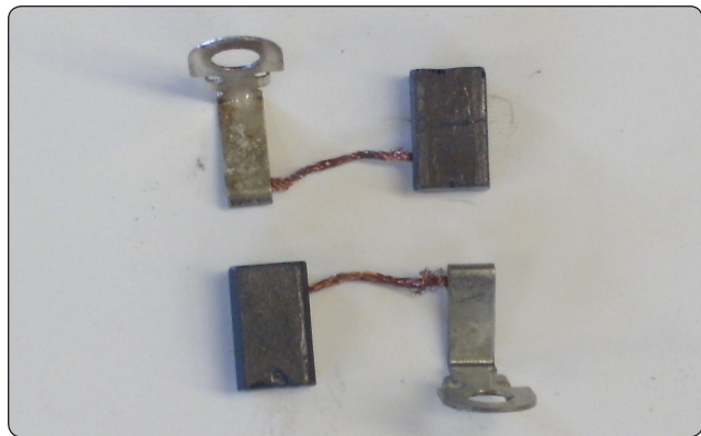
Figure 9-71. Alternator brushes.
