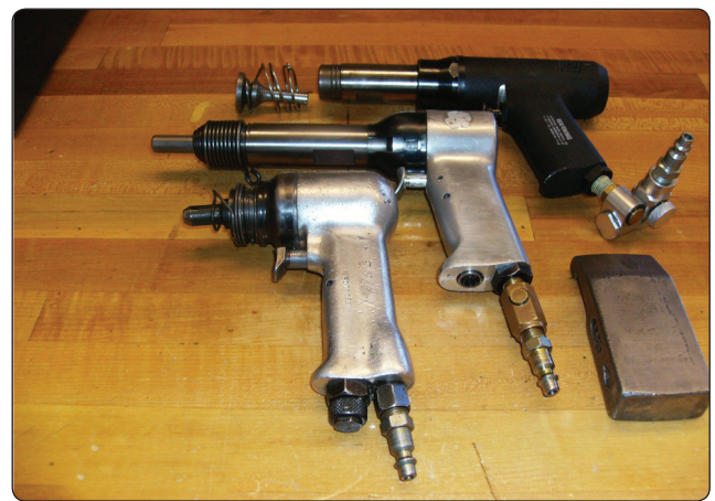
Figure 4-86. Rivet guns.
