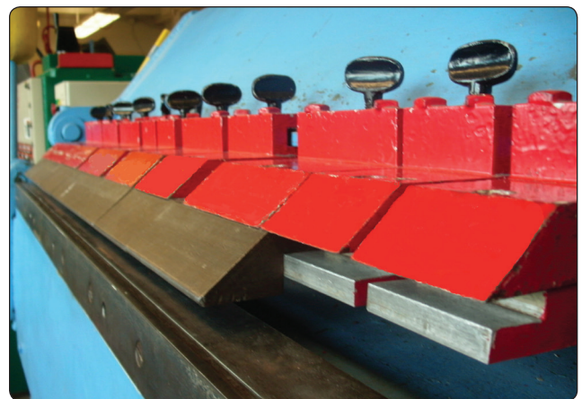
Figure 4-135. Brake radius nosepiece adjustment.
