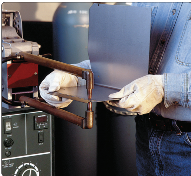
Figure 5-10. Spot welding thin sheet metal.
