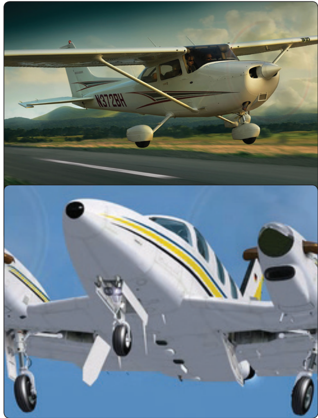
Figure 1-82. Landing gear can be fixed (top) or retractable (bottom).
