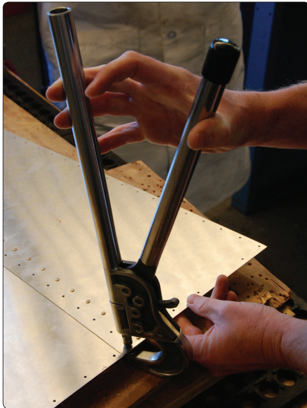
Figure 4-93. Hand squeezers.
