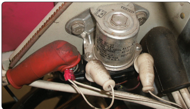
Figure 9-85. Battery solenoid.
