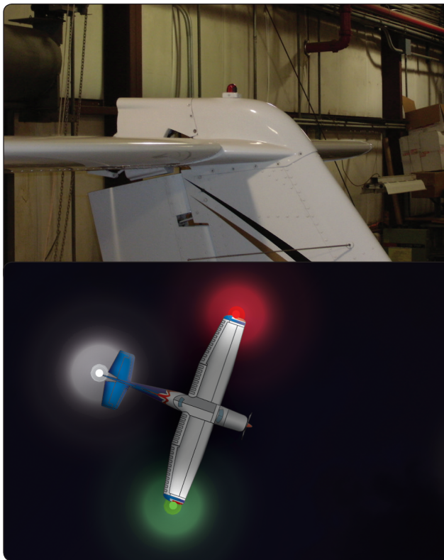
Figure 9-177. Anticollision lights.
