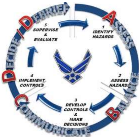
Figure 16.6. The 5-Step Risk Management Process as related to the Real-Time Risk Management Process/ ABCD Model.
